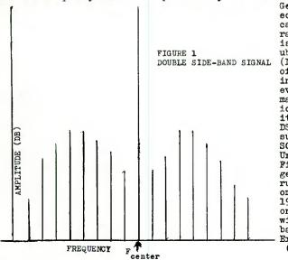
Generally, the spectrum of a broadcast station is rated as AM, which is defined as double-side-band or (DSB). An example of this is shown in Figure 1. However, there are many stations which do not exhibit the classic DSB spectrum. One such station is SODRE, Montevideo, Uruguay, 15273 kHz. Figure 2(next page) shows spectrum data taken fr om SODRE, Aug. 2. 1972,at 2320 GMT on a HQ-180A rx with a 500 Hz IF bandpass filter. Examination of the (SEE NEXT PAGE) .
