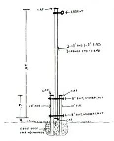
Figure 1: An antenna mast you can homebrew from parts available at your local homebuilders' store and Radio Shack.
