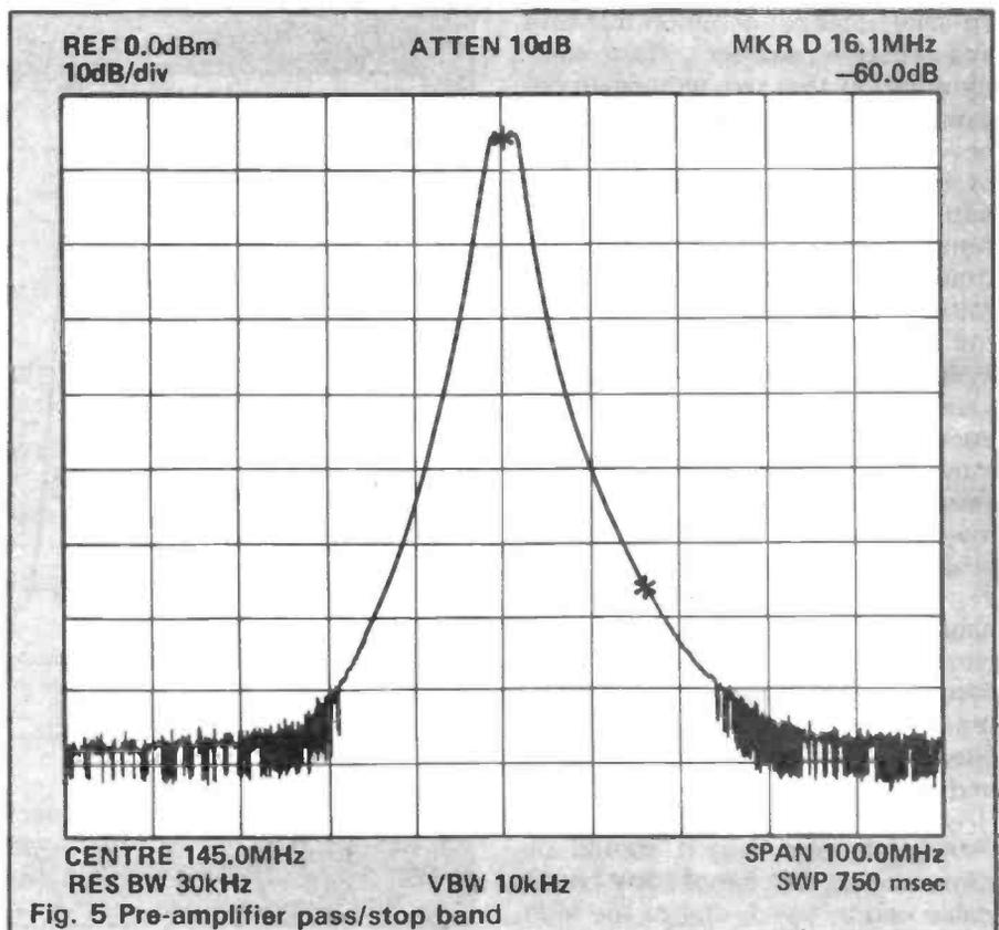
Fig. 5 Pre-amplifier pass/stop band
