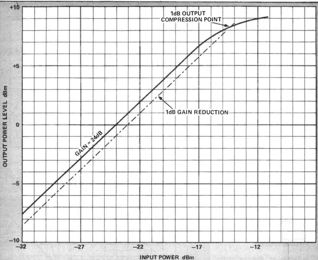
Fig. 8 Pre-amplifier output/Input 1dB compression point
