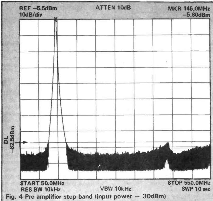
Fig. 4 Pre-amplifier stop band (input power - 30dBm)
