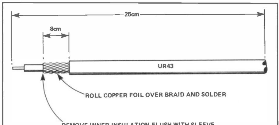
Fig. 10 Details of coaxial terminations to PCB
