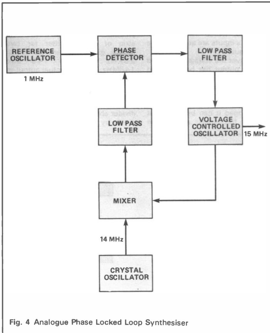
Fig. 4 Analogue Phase Locked Loop Synthesiser
