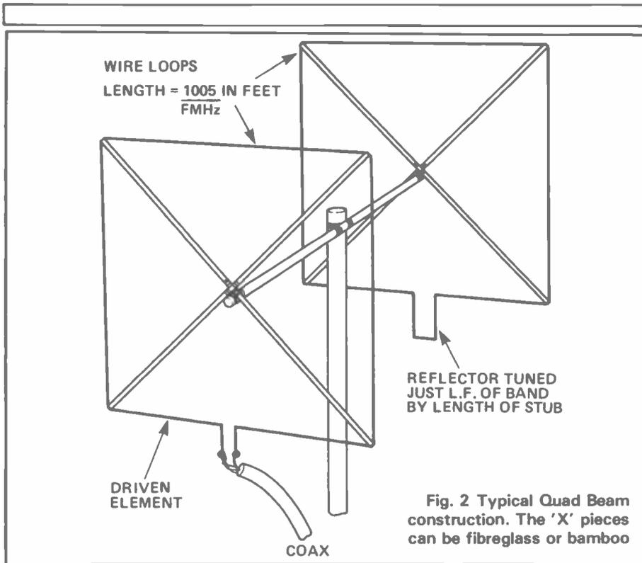
Fig. 2 Typical Quad Beam construction. The 'X' pieces can be fibreglass or bamboo
