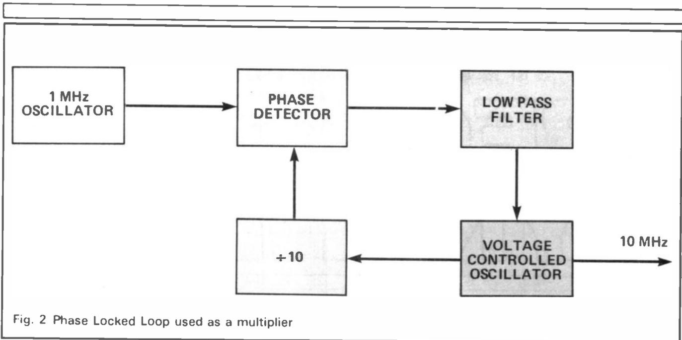
Fig. 2 Phase Locked Loop used as a multiplier
