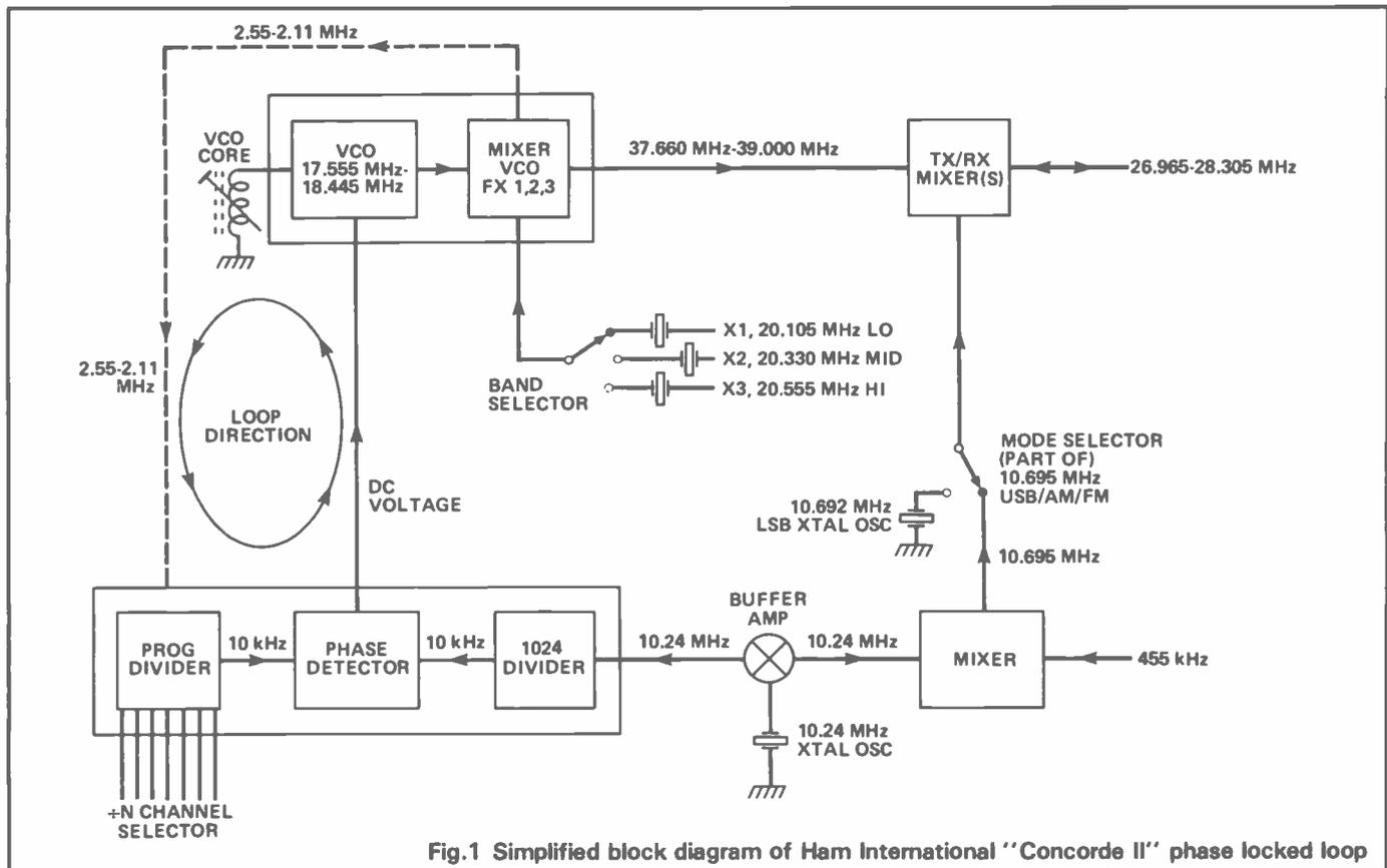
Fig.1 Simplified block diagram of Ham International "Concorde II" phase locked loop
