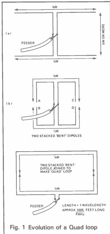
Fig. 1 Evolution of a Quad loop
