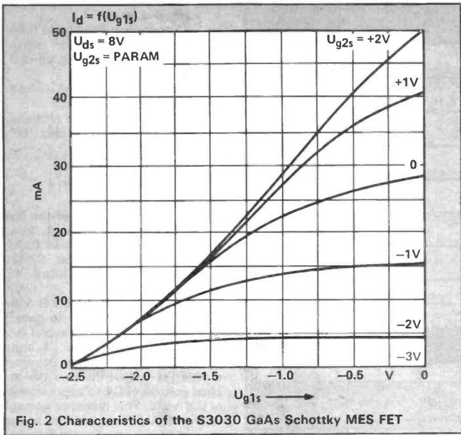
Fig. 2 Characteristics of the S3030 GaAs Schottky MES FET
