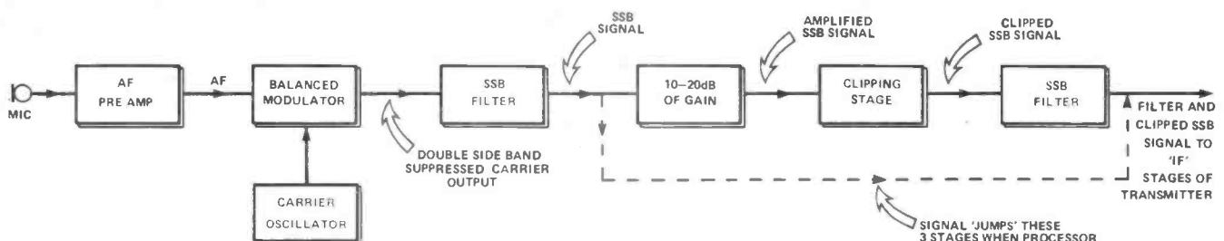
Fig. 2. RF speech clipping in the *FT101*, which will be described in a future article.
