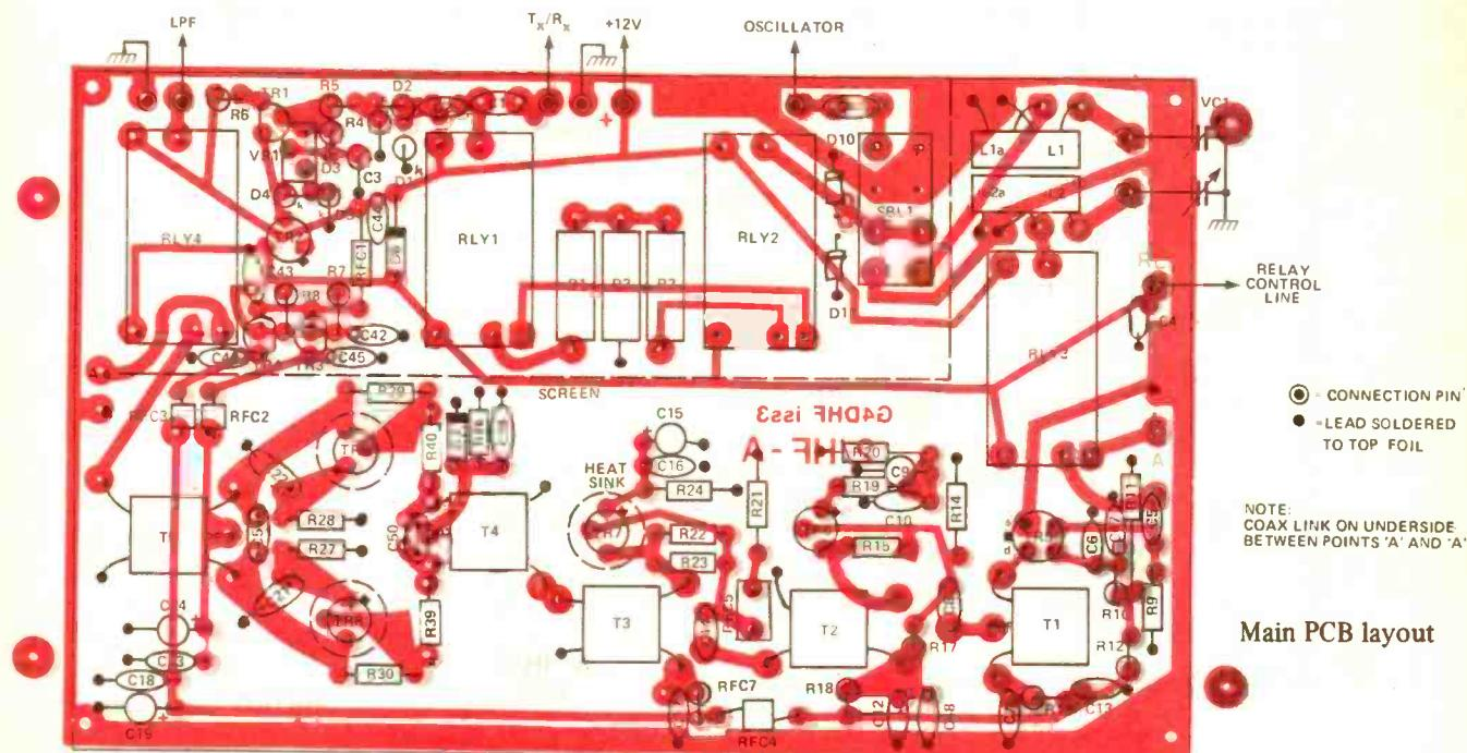
Power output to be expected from this transverter with a 12V supply is a minimum of 2W on all bands with typically 2½ to 3W available on 20 metres.
