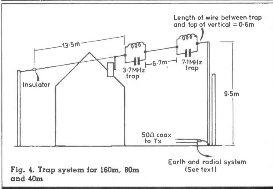
Fig. 4. Trap system for 160m, 80m and 40m
