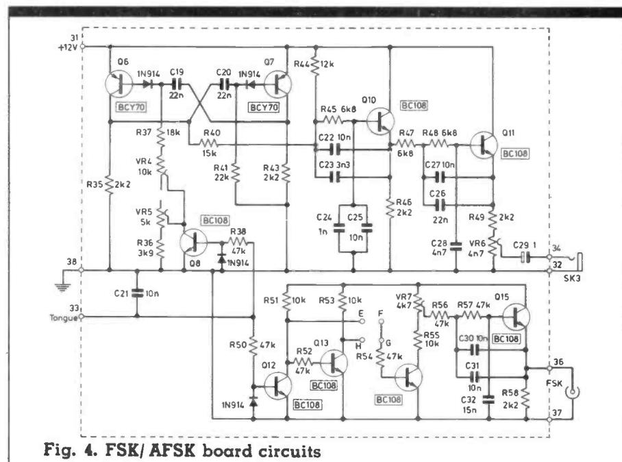
Fig. 4. FSK/AFSK board circuits
