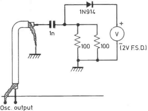
Fig. 6. Oscillator alignment
