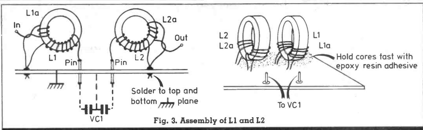
Fig. 3. Assembly of L1 and L2
