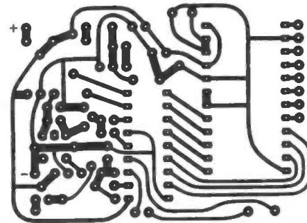
*The PCB layout for the EPROM programming board.*
