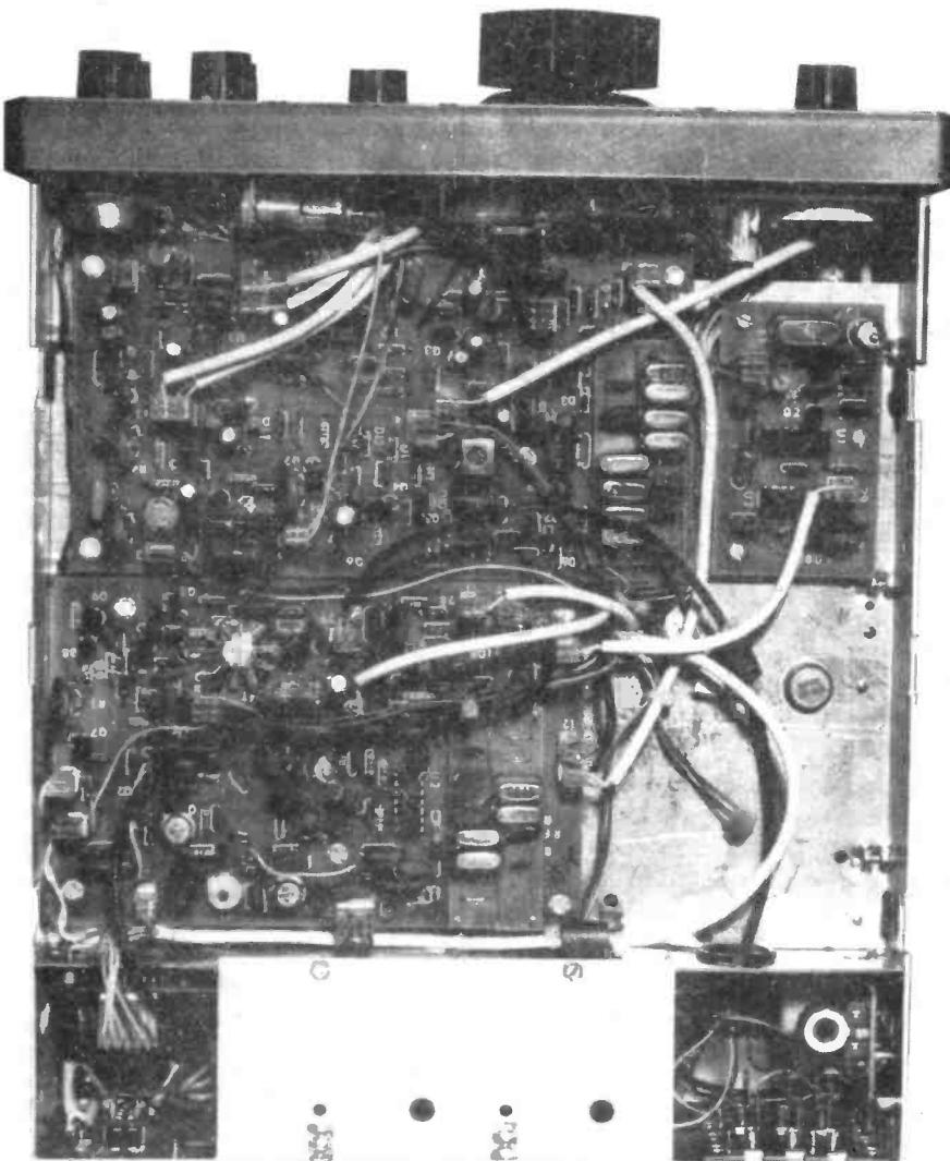
linearity, and its output is fed via the high/low power switch to the low pass filter board, where it passes through the low pass filter and the SWR bridge before being fed to the aerial.
