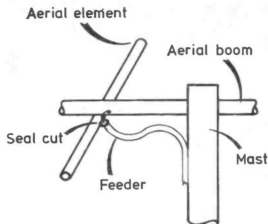
moisture enter the feeder as comparatively small amounts accumulating over the years will slowly but steadily build up the losses to a point where the cable becomes unuseable and has to be replaced which can become very expensive if some of the low loss types of feeder are used. If these precautions are observed then not only should events like those that I have just recounted be avoided but also the life of the feeder should be extended.
