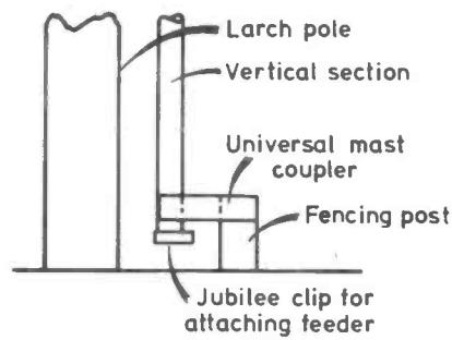
Fig. 5. Base of vertical section on insulated fencing post
