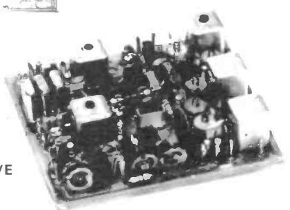
Converts any surplus radio telephone into a continuously variable F.M. transceiver. Microphone is connected to unit and a stable 2 metre F.M. signal is available for driving the amplifier stages. On receive the unit produces a local oscillator signal 10.7MHz below signal frequency. •600KHz repeater shift •Suitable for other I.F.'s •Extension for digital display •Kit includes all components (exc 3 Xtals and varco) •8 pages of directions. £17.15 (directions only £0.95)
