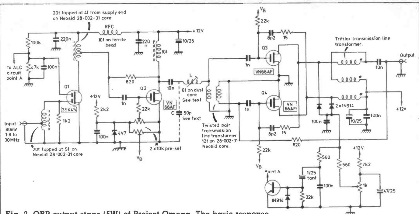
**Fig. 2. QRP output stage (5W) of Project Omega. The basic response is 1 to 120MHz but see text.**
