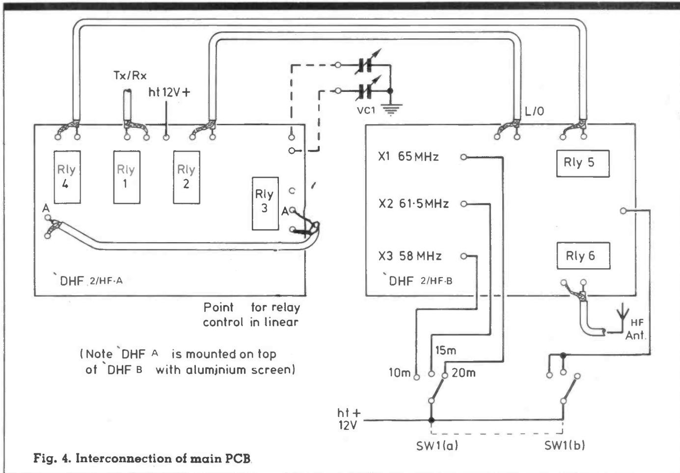
Fig. 4. Interconnection of main PCB
