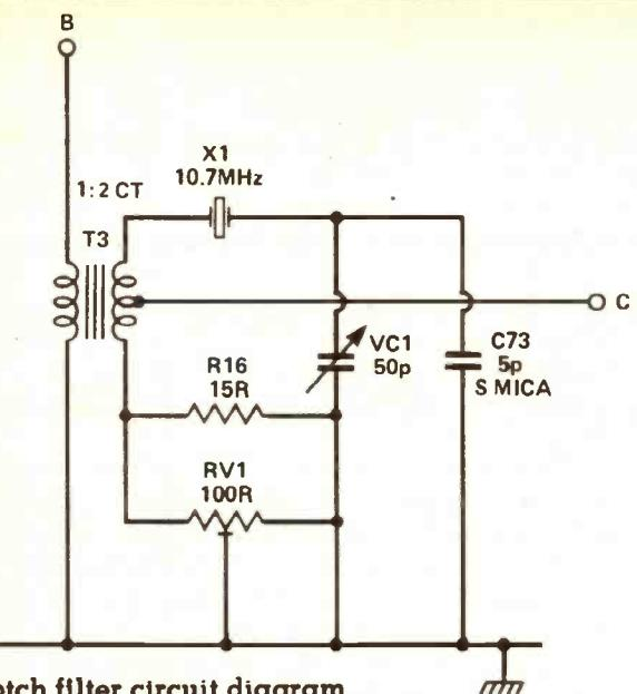
Notch filter circuit diagram
