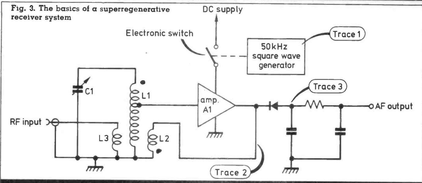
oscillator and the second is a means of detecting the presence of RF oscillations in the system. In practice, the quenching may be done by a secondary oscillatory loop switching on and off the first one. Similarly an RF oscillatory state may be detected by the non-linearity of the oscillator transistor itself, ie looking for a change in collector current with oscillation.
