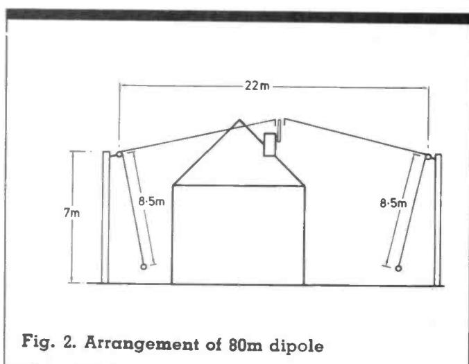
Fig. 2. Arrangement of 80m dipole
