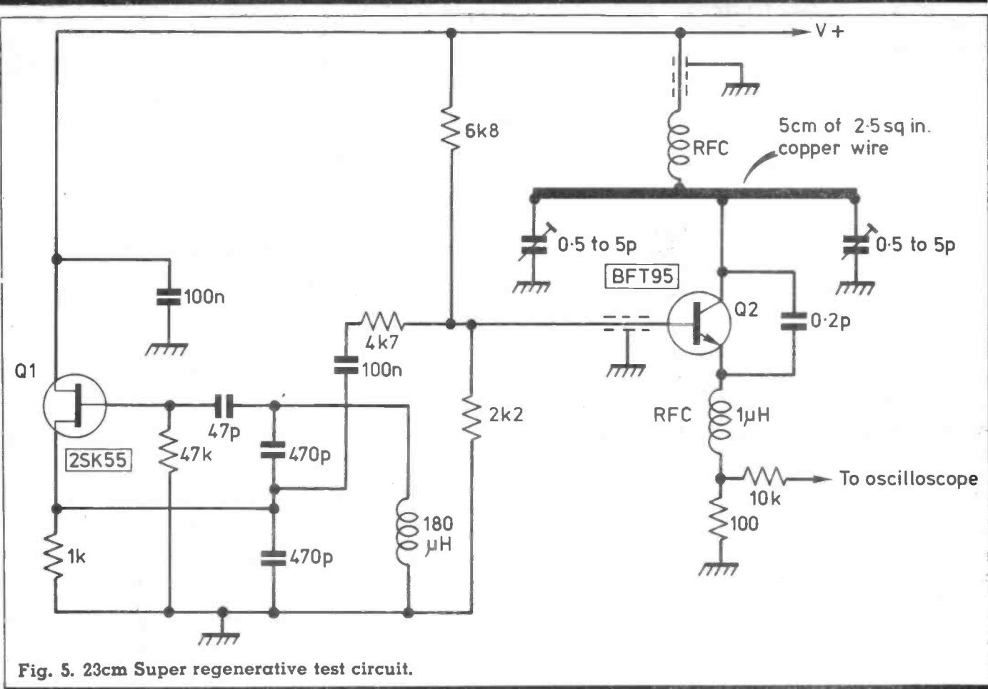
Fig. 5. 23cm Super regenerative test circuit.
