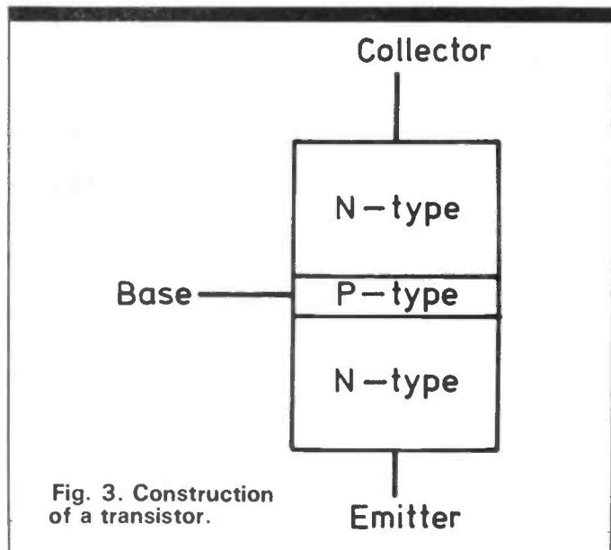
Fig. 3. Construction of a transistor.
