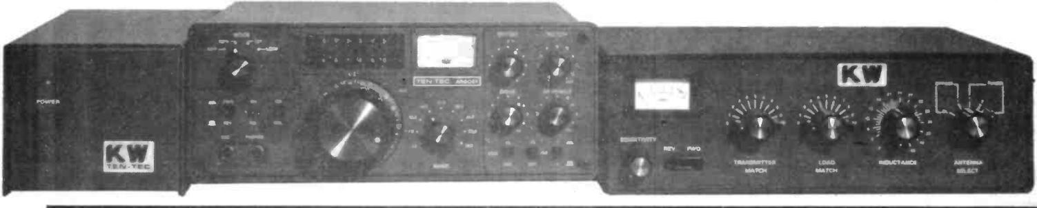
deed. The calibrator, which is, incidentally, an optional extra, provides signals at 25kHz intervals and is pulsed at a rate of two or three times a second to assist identification.
