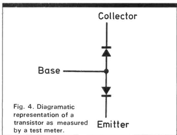
Fig. 4. Diagrammatic representation of a transistor as measured by a test meter.
