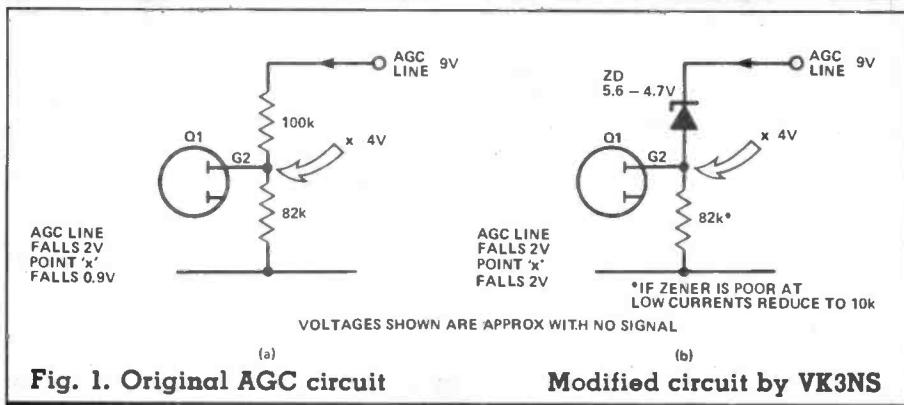
**Fig. 1.** Original AGC circuit
