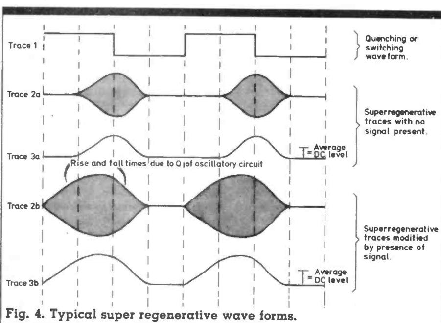
**Fig. 4. Typical super regenerative wave forms.**
