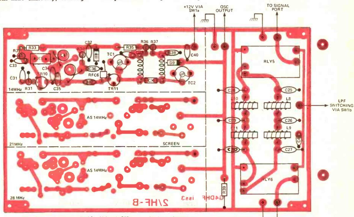
Oscillator/low pass filter PCB layout
