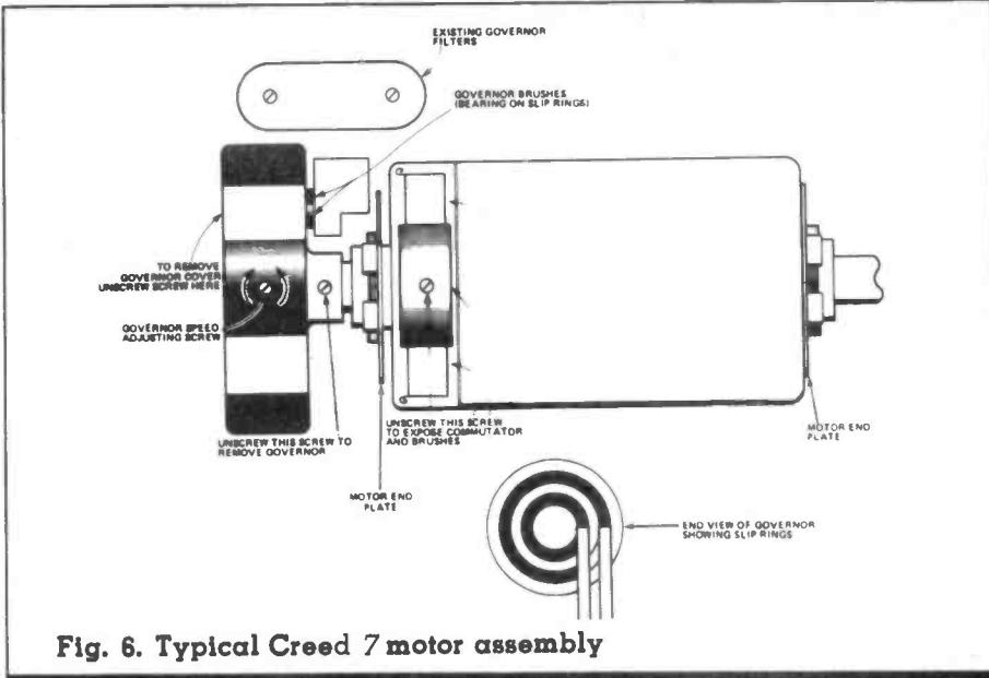
Fig. 6. Typical Creed 7 motor assembly
