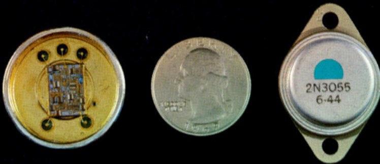
Figure 1: The Small Hybrid Thin-Film Amplifier, Compared with a Quarter and a Transistor from a Conventional CATV Amplifier Power Supply.
