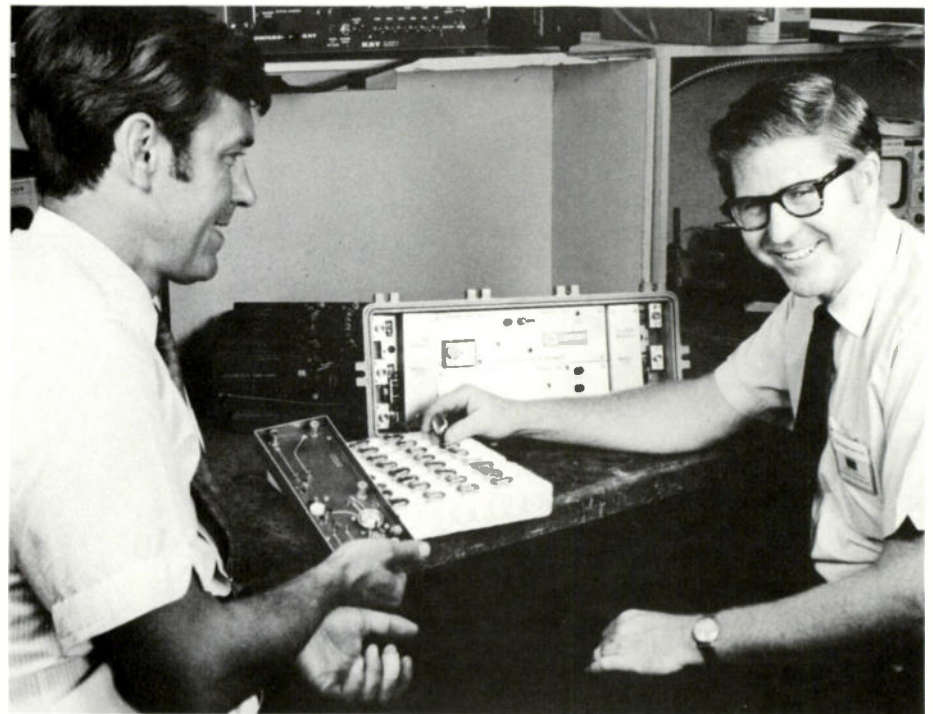
Gay Rogeness (r), Director of Engineering at Anaconda Electronics, and Vic Tarbutton (l), R & D Engineer were key men in Anaconda's development of microelectronic circuitry for CATV. They are shown here displaying the new hybrid thin-film IC amplifier as it is located in a module of the Century Trunk Amplifier.
