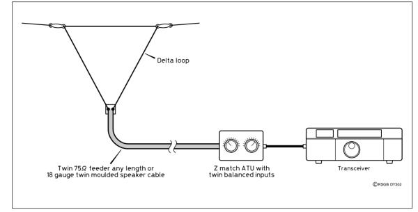
Fig 1: Multiband version of the delta loop connected to the ASTU using  $75\Omega$  twin feeder.
