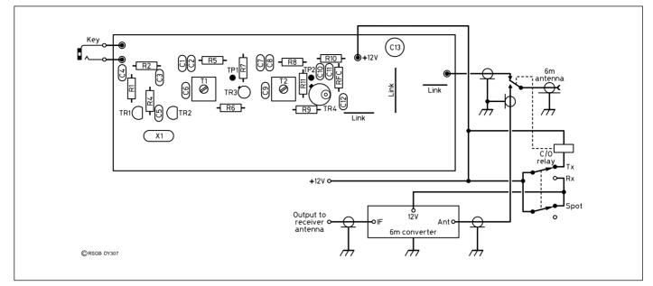
Fig 2: Layout of the components and antenna changeover relay. This is also shown with the 6m converter; see text.
