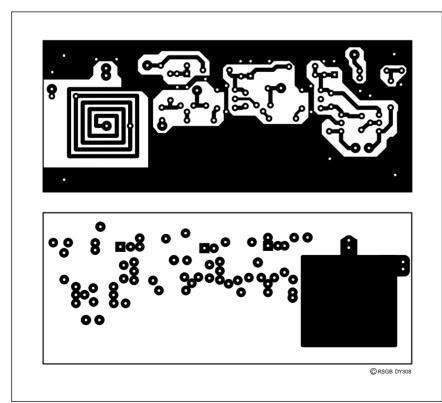
Fig 3: Printed Circuit Board: (Top) Track side showing PCB 'coil' L1. (Bottom) Ground-plane side or components side. The black areas on this side of the board are where the copper must be removed. Note that the above layout is 70% of the true size.
