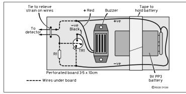
Fig 3: Water detector constructed from stripboard.
