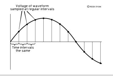
Fig 3: Sampling an analogue waveform.
