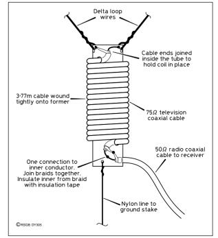
Fig 4: Detail of the 20metre band coaxial balun.
