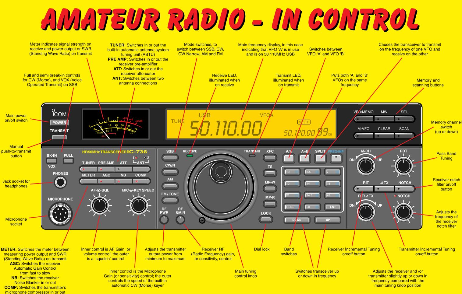
Many HF and VHF transceivers can look very complicated at first glance. However, all the controls have a logical function, and these are described above with the aid of the drawing of an Icom IC-736 transceiver, which covers all the HF bands (1.8 - 28MHz) plus the 6m (50MHz) band.
