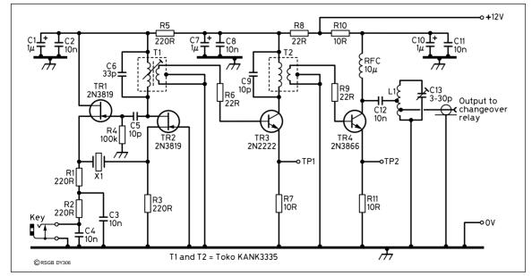
Fig 1: The 50MHz transmitter circuit diagram. TP1 and TP2 are included to assist in setting up the transmitter; see text.
