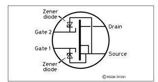
Fig 1: how the Zener diodes in a IGFET are arranged. Note that they are not normally shown on a diagram.
