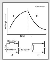
connected across a resistor (see B) current will flow through the resistor and discharge the capacitor. The capacitor's voltage now drops - see curve B. The higher the value of the resistor, the longer it takes to charge, or discharge, the capacitor.
