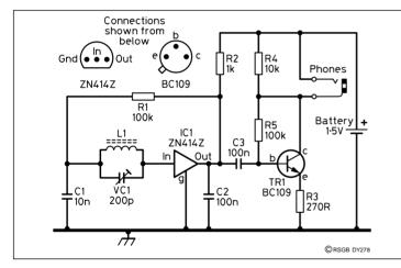
Fig 1: Simple medium -wave radio, circuit diagram. Note that the pin connections to IC1 and TR1 are shown from below.
