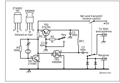
Fig 1: Circuit diagram of the breadboard transmitter.
