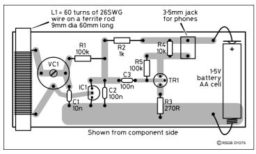
Fig 2: Component layout using PCB board.
