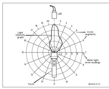
Fig 2: Torch light intensity pattern plotted at RSGB HQ.
