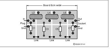
Fig 2: Layout and construction of filter.
