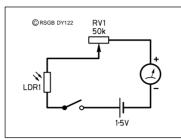
Fig 1: Circuit diagram of photometer.
