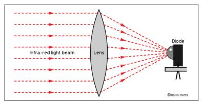
Fig 2: A simple lens focuses the infra-red light to improve the signal.
