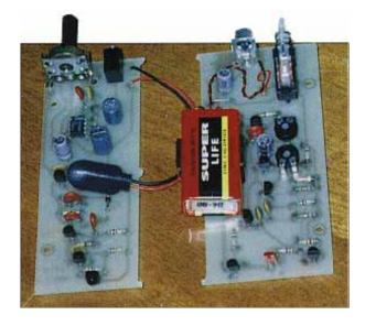
components; we made a few silly mistakes in our haste to complete the project. Some parts needed their leads bending a little in order to fit them into the board.
