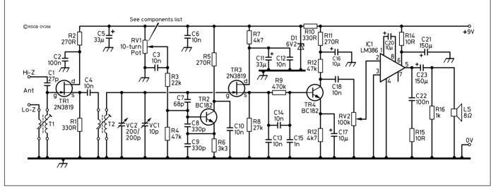
Fig 2: The circuit diagram showing the 10-turn potentiometer RV1. This is the regeneration control for the Nicky.
