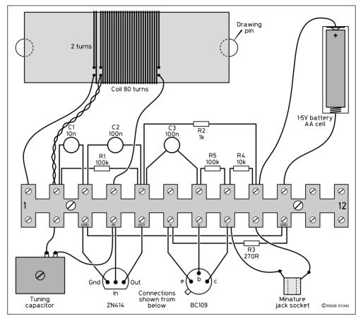
Fig 3: Component layout using connector strip. This layout is shown using the plastic or cardboard tube alternative coil former. An external wire antenna can be connected to tag strip connector 1 if required.
