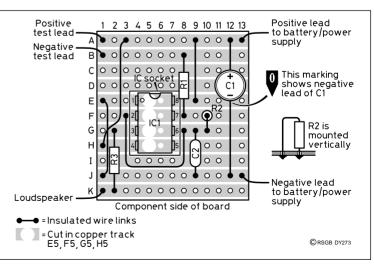
Fig 2: Veroboard Layout for the D-i-Y'er 555. If you can read a circuit diagram, the project can be built using other methods.
