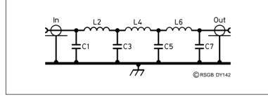
Fig 1: Circuit diagram of filter.
