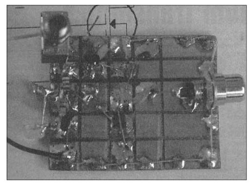
The breadboard transmitter, showing its construction on PCB pads.
