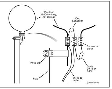
Fig 2: Broadband and tunable field strength meter.
