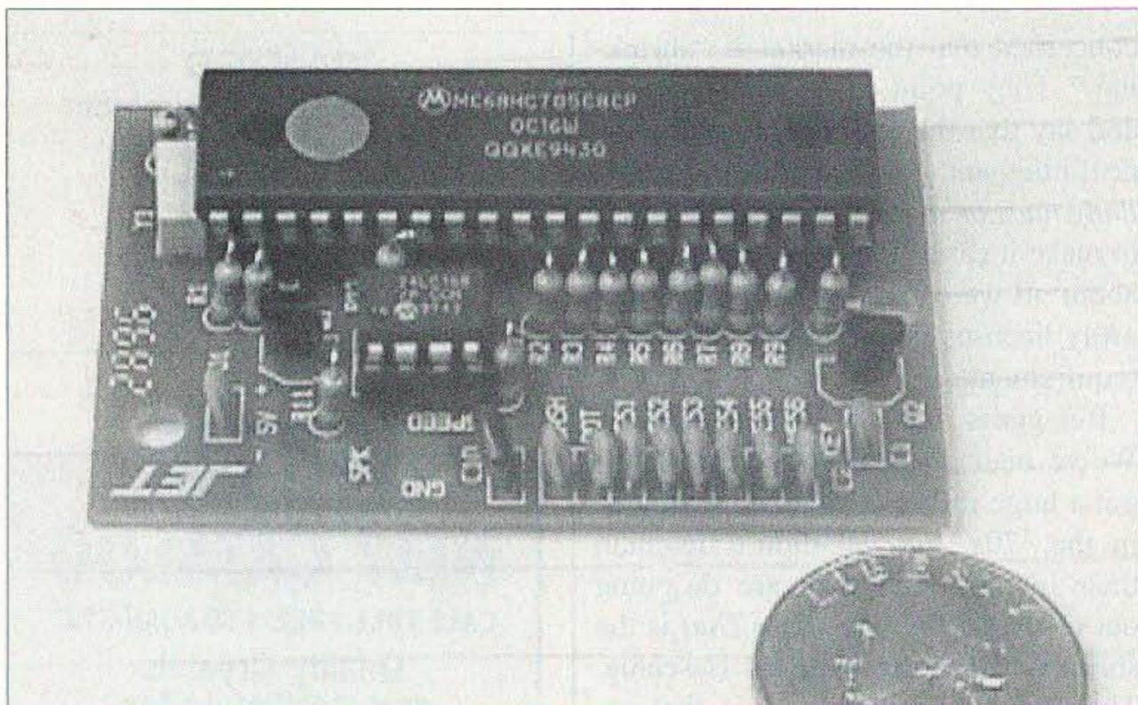
**Photo D.** Modern "single chip" electronic memory keyer, with microprocessor control.
