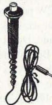
Good-quality pushbutton with 39" cord, probably originally designed for photographic application. Normally-open, momentary switch (current rating unknown) is encased in a 2" long plastic and rubber assembly with cable strain relief. The cable is terminated with a small co-ax barrel plug. Black assembly with white pushbutton.
