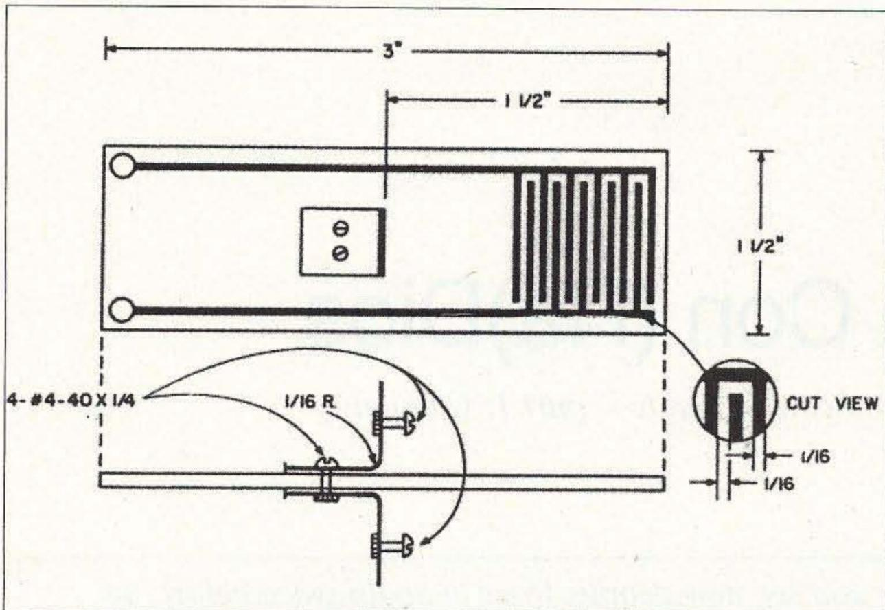
Fig. 2. Etch board on both sides.
