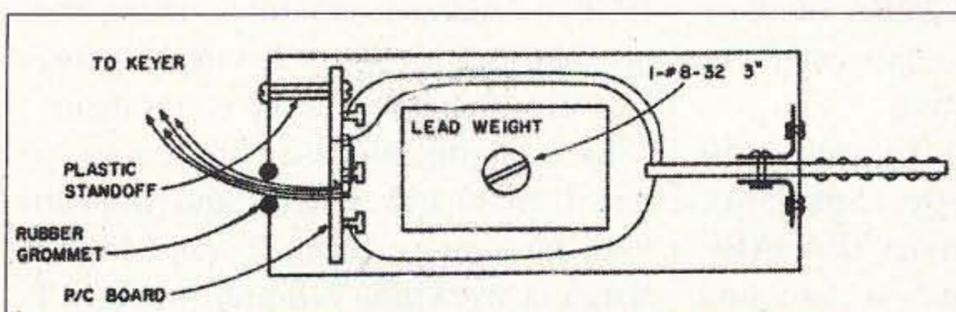
Fig. 3. Box layout, top of box looking up.
