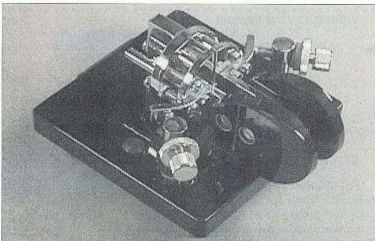
**Photo E.** Modern high-speed dual paddle, by G4ZPY. The design is optimized for operation at up to 60 wpm.
