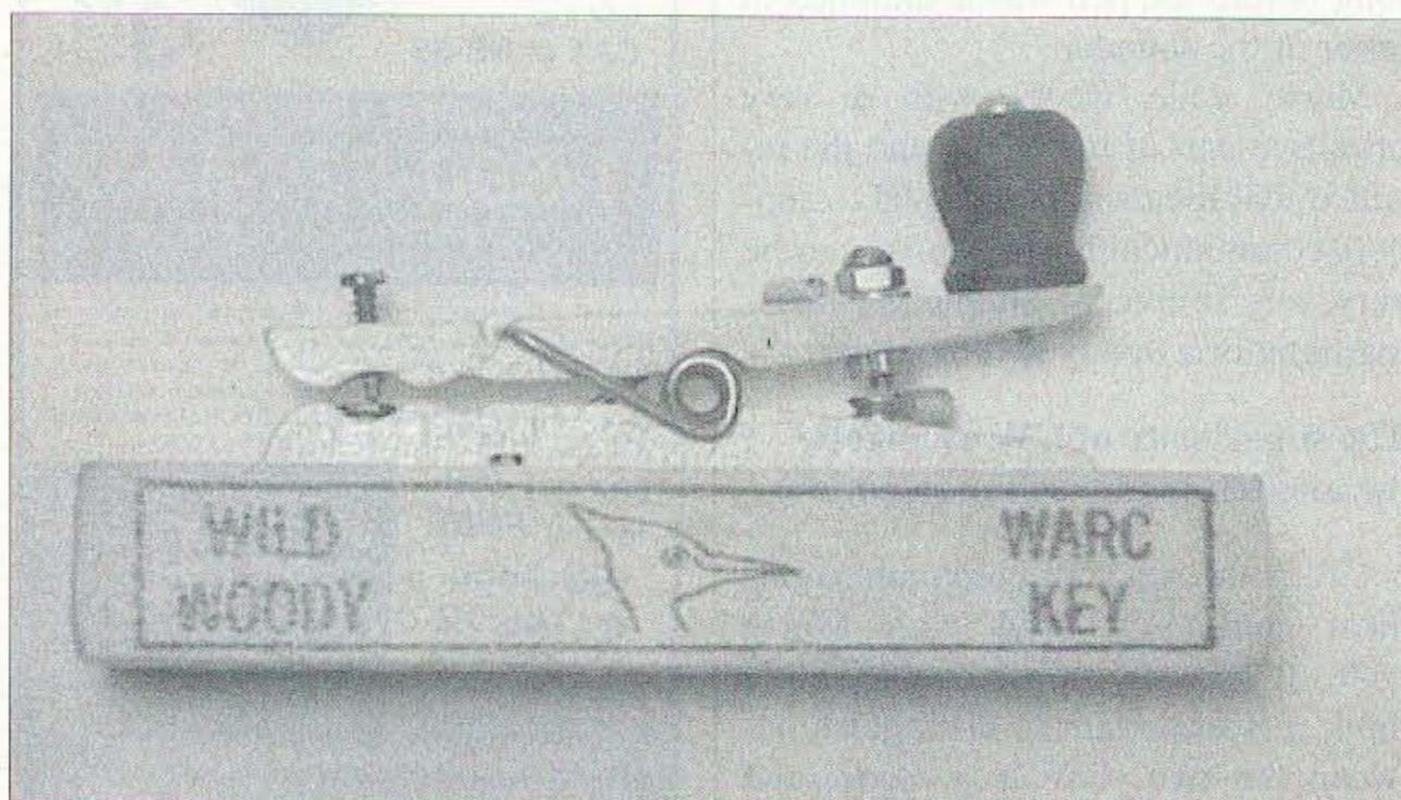
**Photo C.** A fully functional telegraph key made from a clothes pin by K4TWJ.
