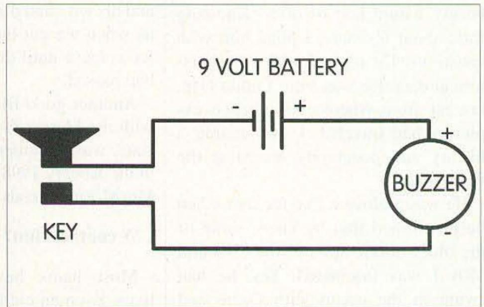
**Fig. 1.** Wiring diagram for the Morse code buzzer.
