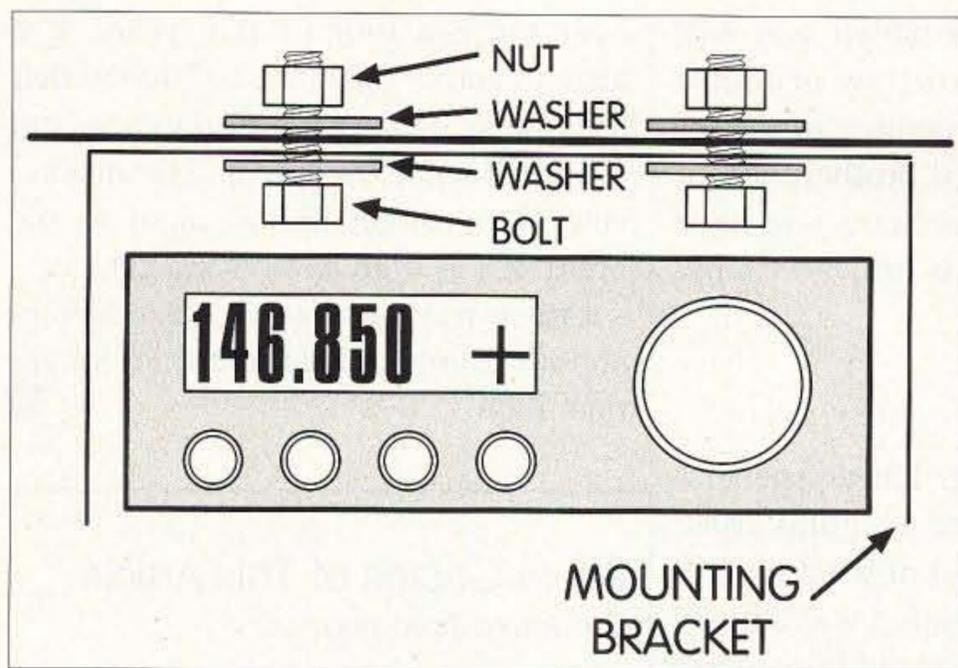
**Fig. 1.** Using large washers or a piece of sheet metal to distribute the weight of the radio can make it possible to mount a small radio to the underside of a plastic dashboard.
