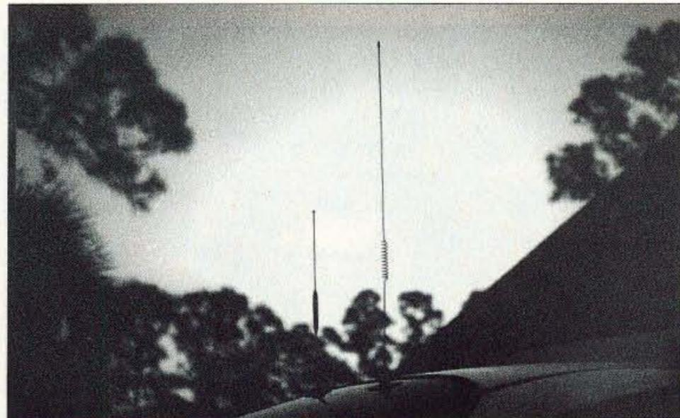
**Photo B.** On-glass mount antennas have benefited from technology developed by the cellular telephone industry, and work well for VHF and UHF applications.
