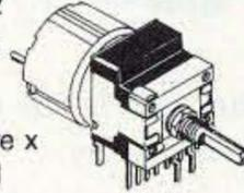
Alps Electric # 726T-10KBX2 Dual 10K linear pot powered by a small reversible 6 Vdc gearhead motor. Pot and motor assembly are 1" square x 1.7" long excluding shaft and bushing. 6 mm flatted shaft is 0.5" long. 9mm threaded bushing. PC pins and mounting tabs for pc board mounting.
