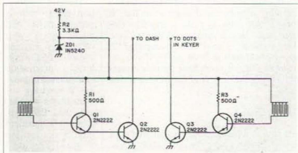
Fig. 1. R1, R3 — 500Ω, 1/2 W; R2 — 3.3kΩ, 1/2 W; Q1, Q2, Q3, Q4 — 2N2222 or equivalent; ZD1 — 10 V, 0.5W 1N5240.
