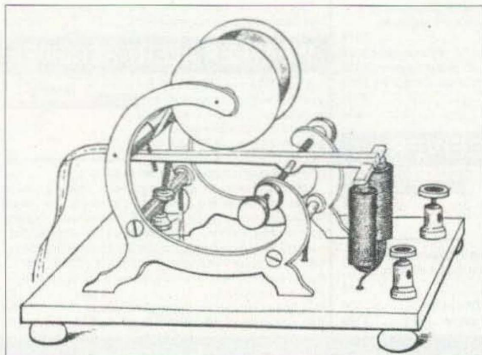
**Photo A.** 1850s pen register. During a dot or dash, the current through the coils creates a magnetic field that pulls the lever down, pressing a pen against the paper tape.
