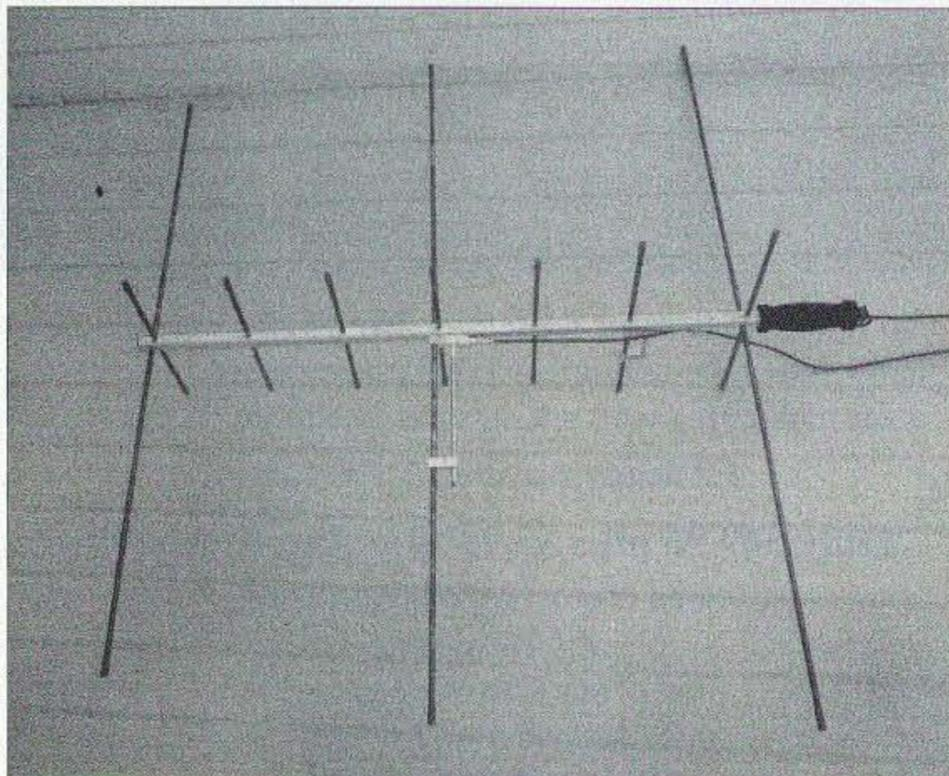
**Photo C.** After only a few minutes, the bag of parts turns into a very effective hamsat antenna.
