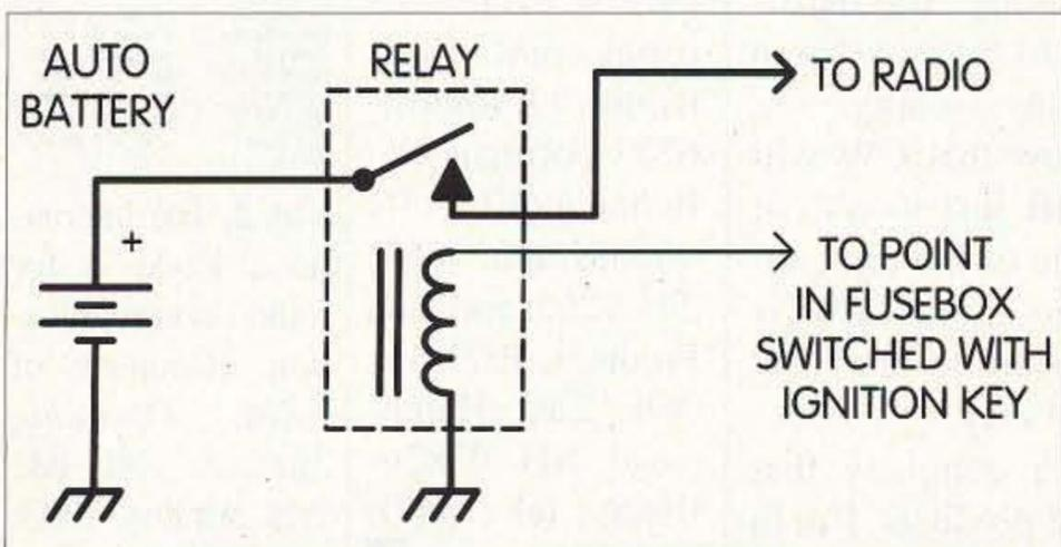
**Fig. 2.** A relay can be used to switch off a mobile radio whenever the ignition is turned off. Make sure you use a relay that can handle the current required by your radio.
