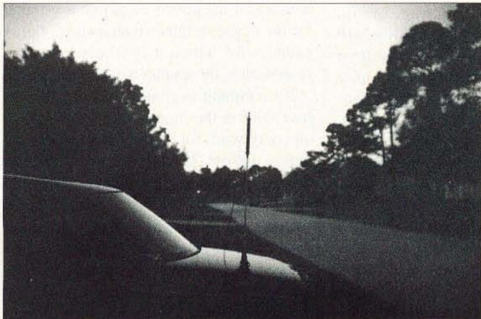
**Photo A.** Taller mobile antennas should be mounted on the driver's side to better clear tree limbs hanging over the road.
