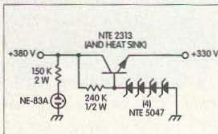
**Fig. 2.** Schematic of the +330-volt regulator. The NE-83A indicator and 33k resistor are on the original SB-620 front panel.
