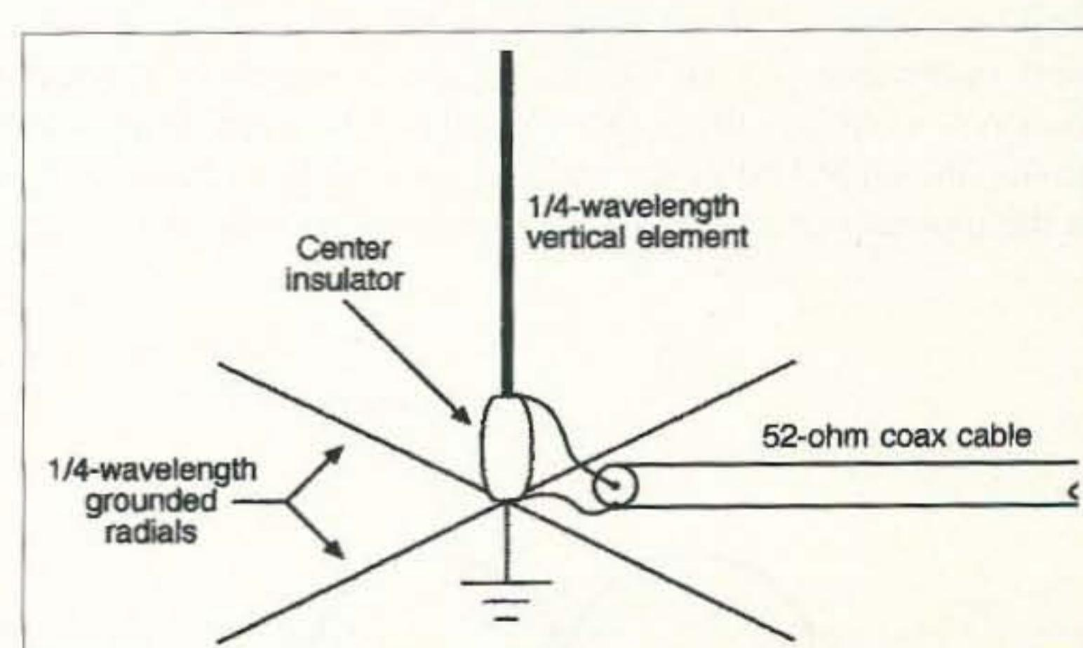
**Fig. 3.** Quarter-wave vertical, viewed from the side. Each radial, and the main vertical element, is 1/4-wavelength long. The center conductor of the coax is connected directly to the vertical element and the shield of the coax to ground.
