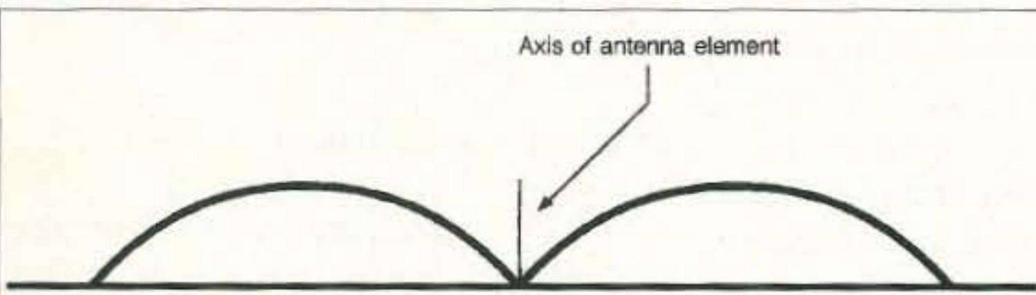
**Fig. 6.** Idealized vertically compressed radiation pattern of a 1/4-wave gain-designed antenna.
