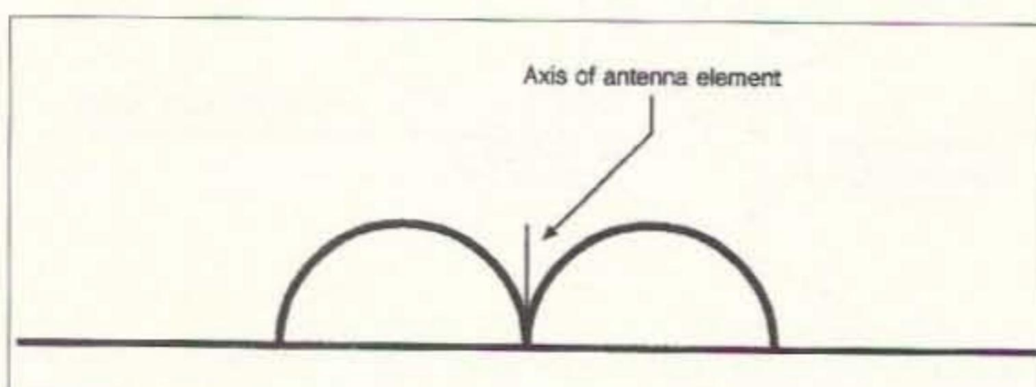
**Fig. 5.** Idealized radiation pattern of a 1/4-wave vertical, viewed from the side.
