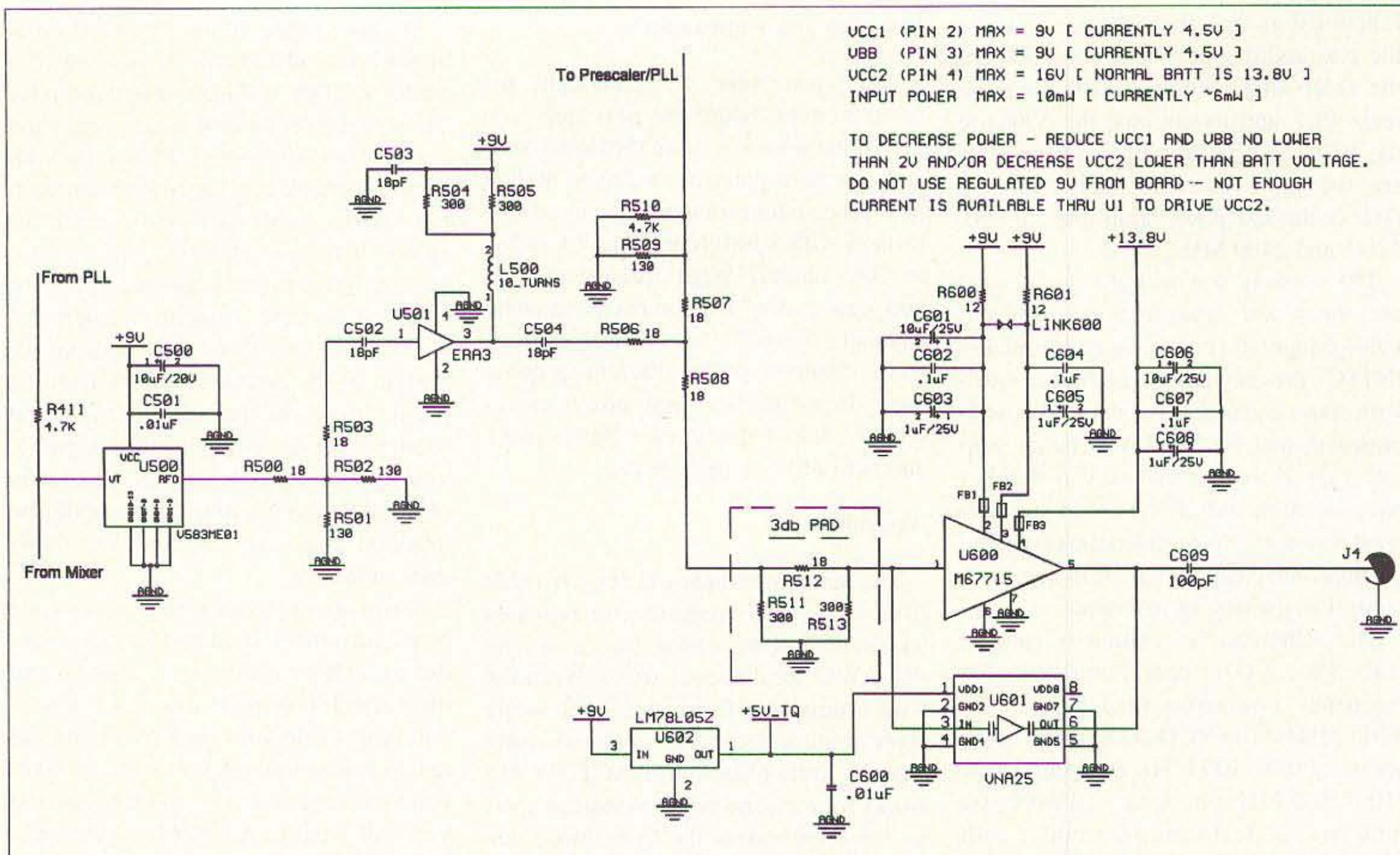
**Fig. 7.** High- and low-power amp. VCC1 (pin 2) max = 9 V (currently +4.5 V). VBB (pin 3) max = same. VCC2 (pin 4) max = 16 V (normal battery is 13.8 V). Input power max = 10 mW (currently ~6 mW). To decrease power, reduce VCC1 and VBB no lower than 2 V and/or decrease VCC2 lower than battery voltage. Do not use regulated 9 V from board—there is not enough current available through U1 to drive VCC2.
