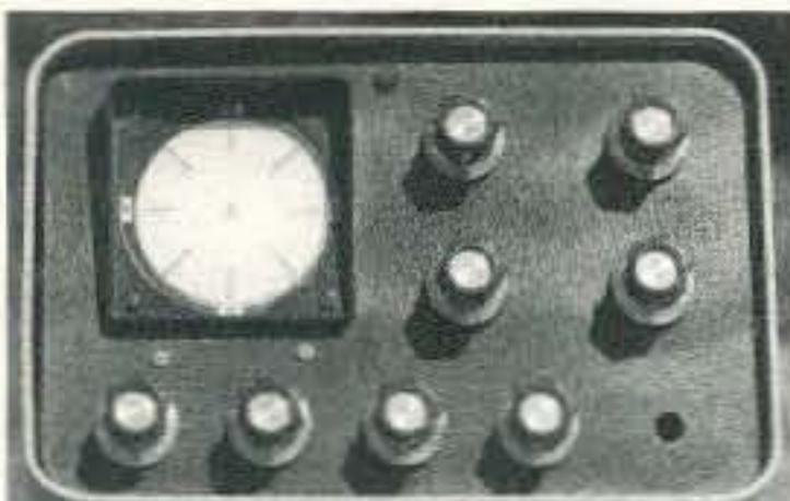
**Photo A.** The Heathkit Scalyzer after repainting the front panel and replacing the grid screen under the CRT bezel with a transparent compass overlay. Next comes labeling. The hole at lower right will be filled by a future control.
