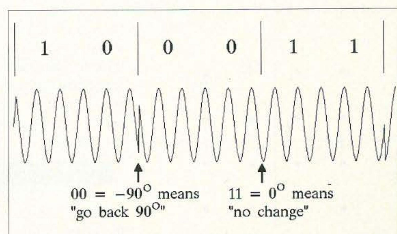
**Fig. 6.** DPSK-4 with four phase angles.
