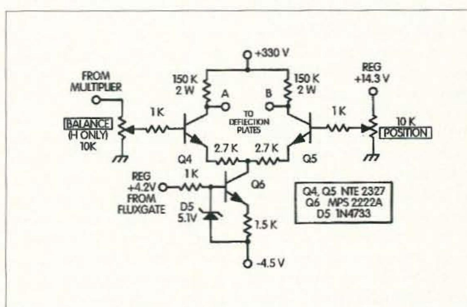
**Fig. 1.** Schematic of the new deflection circuits. Two are required, each with a spot positioning potentiometer on the front panel. A and B outputs of the horizontal (X) circuit go to the orange and yellow CRT socket wires, respectively. A and B outputs of the vertical (Y) circuit go to white and violet socket wires.
