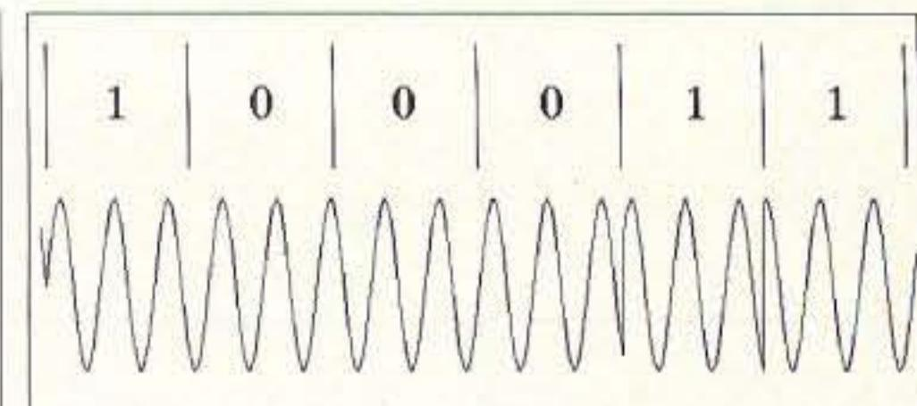
**Fig. 5.** DPSK-2 with two phase angles.
