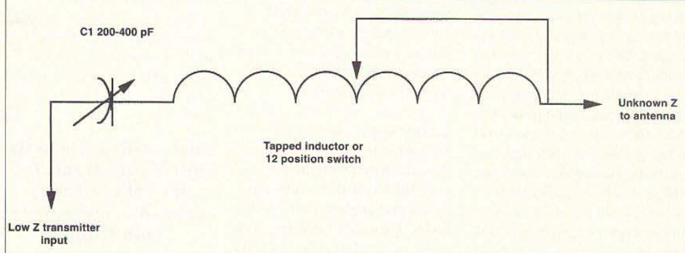
Fig. 1. Schematic for the tuner.
