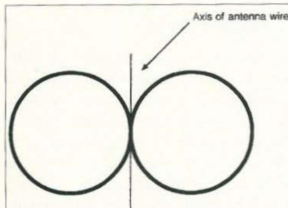
**Fig. 1.** Idealized radiation pattern of a half-wave horizontal dipole antenna, as viewed from directly above.
