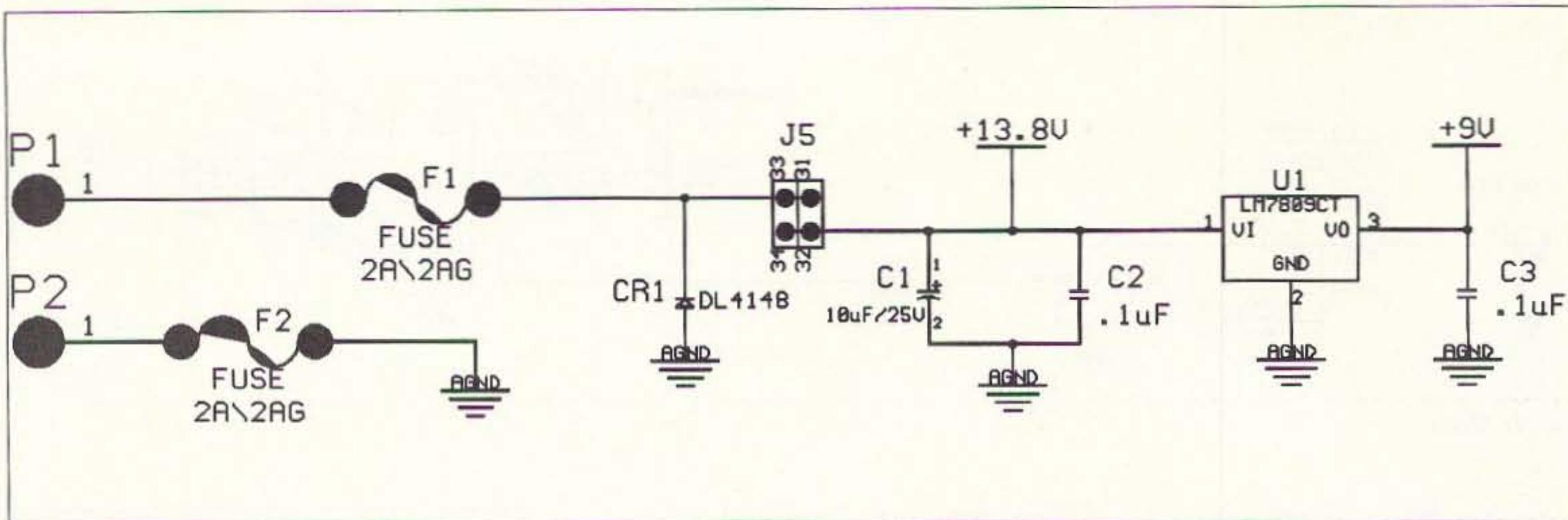
Fig. 5. Power input section.
