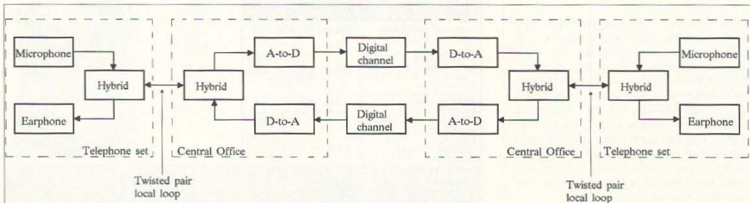
**Fig. 1.** Signal path through the POTS network.
