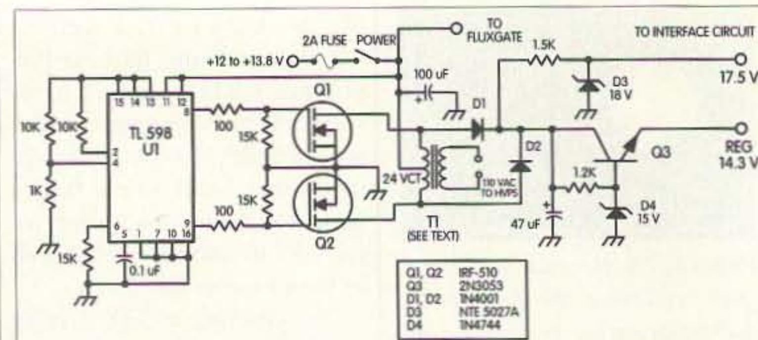
**Fig. 3.** Schematic of the DC-to-AC converter. Outputs are 110 VAC square-wave for the high voltage supply and positive DC for the analog multiplier circuits.
