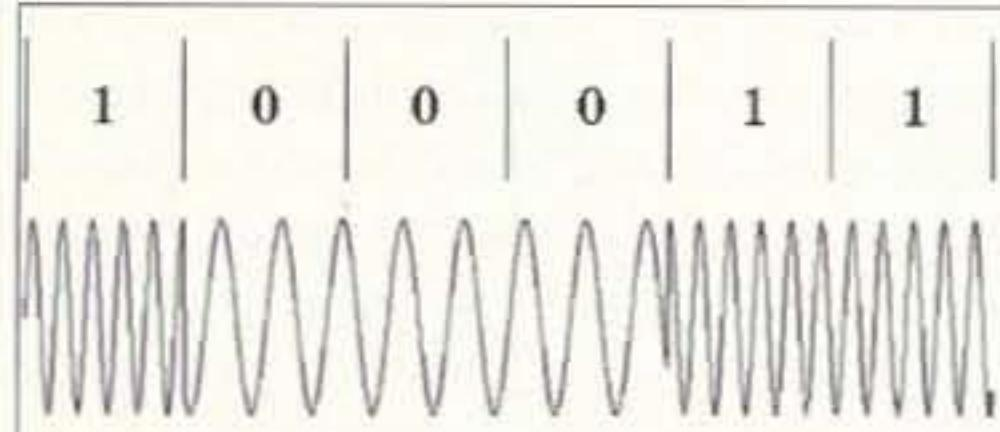
**Fig. 2.** Frequency-shift keying (FSK).
