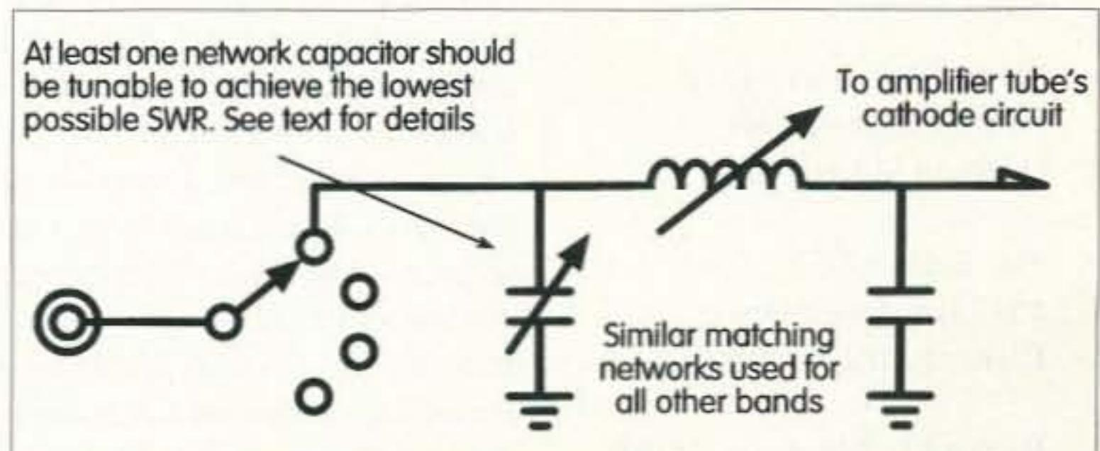
Fig. 2. Typical pi-network used for input matching in a commercial amateur linear amplifier.
