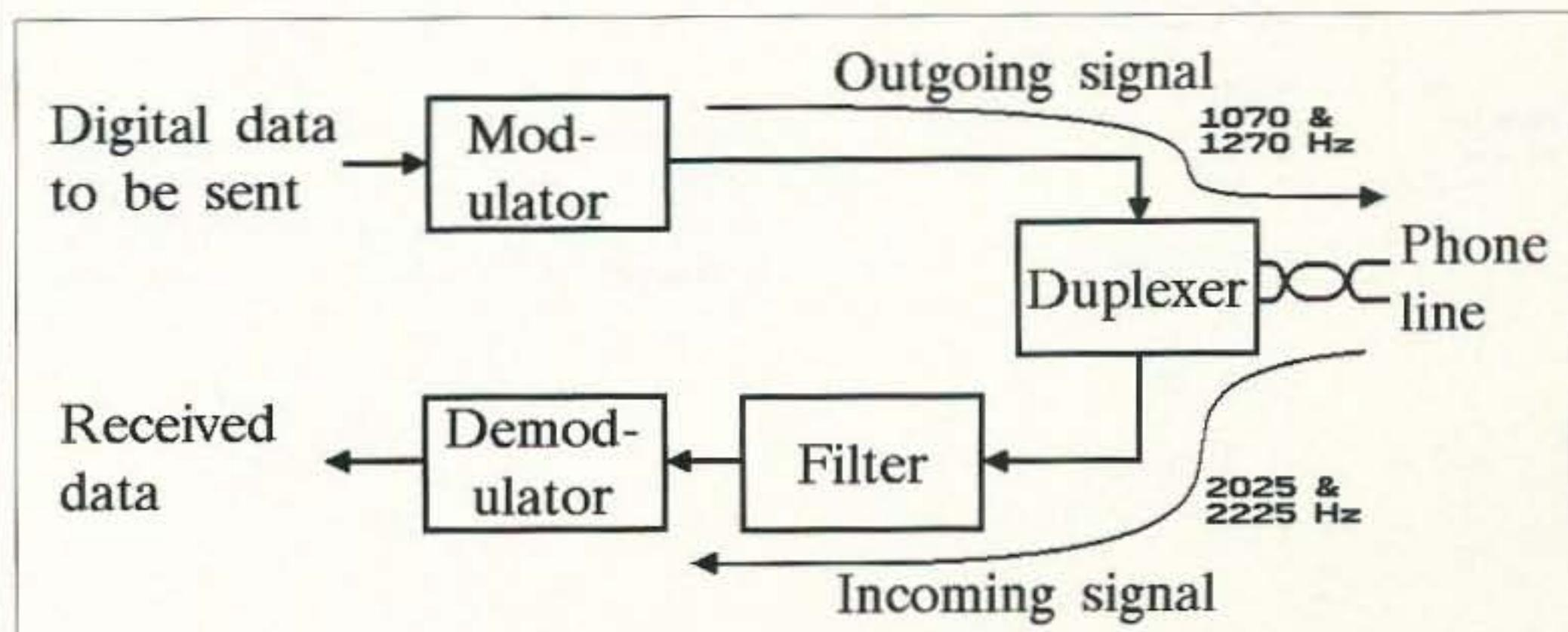
**Fig. 3.** Bell 103 modem block diagram.
