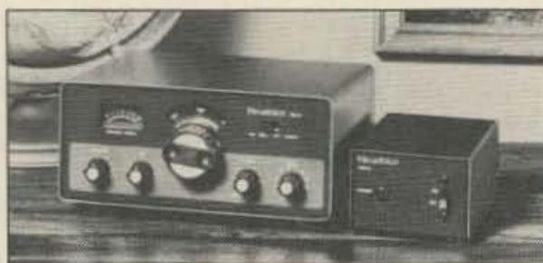
Photo A. The Heath HW-9 QRP transceiver.
