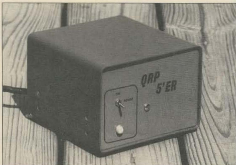
Photo A. The QRP 5er—A small 5-amp power supply just for the low-power operator.
