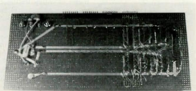
Photo B. Bottom view of the I/O board. The 2 × 20 header is at the right. The electrolytic and ceramic capacitors for the regulator circuit are at the left. Power buses are 1/8"-wide adhesive copper strips made by Circuit-Stik™. Small white spots are paint used to mark correct positions for the sockets and headers. Terminating resistors (input port) were added after the photograph was taken.
