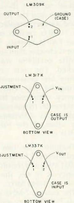
Fig. 2. Pin connections for the LM309, LM317, and LM337 voltage regulators (TO-3 packages).
