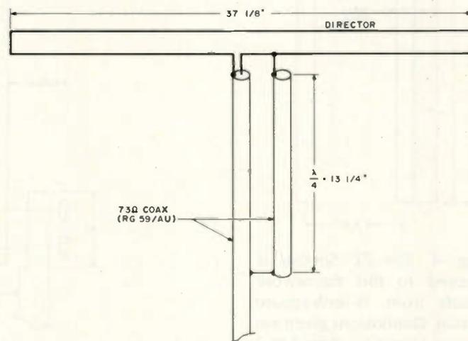
Fig. 3. Dimensions given for the 1-to-1 balun are for 146.5 MHz using coax with a velocity factor of .66. For other frequencies, balun length in inches is calculated from  $2952 \times .66 \div \text{MHz}$ .
