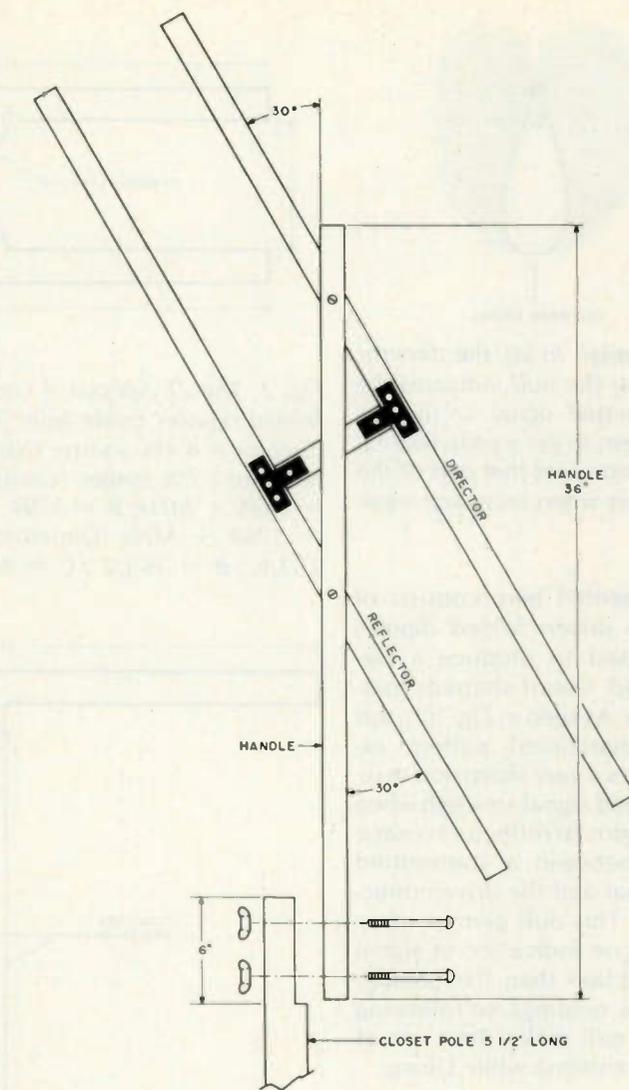
Fig. 5. The positioning of the "H"-shaped framework on its handle determines the tilt of the antenna. The handle is then bolted to a 1 1/4" wooden closet pole.
