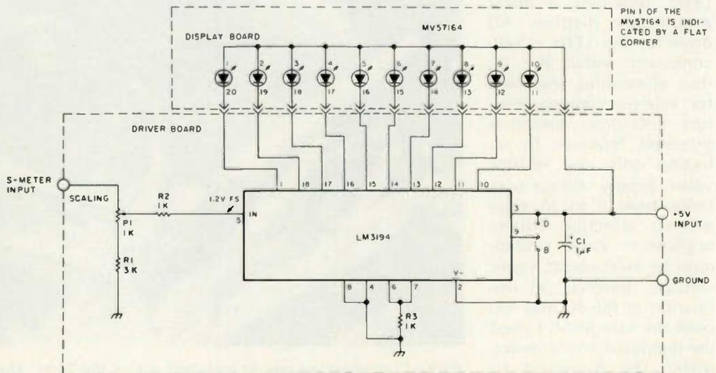
Fig. 1. Schematic of bar-graph S-meter.
