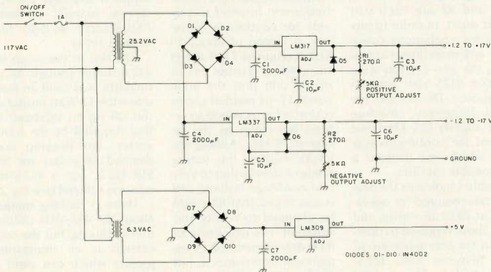
Fig. 1. Tri-voltage power supply schematic.
