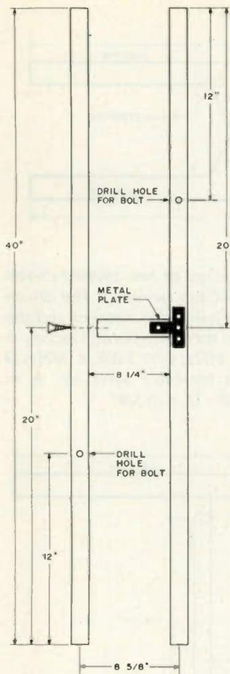
Fig. 4. The ZL Special is tacked to this framework made from 3/4-inch-square wood. Dimensions given are for an antenna cut for 146.5 MHz.
