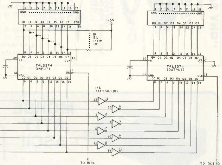
Fig. 2. Schematic of port function circuit. Unmarked capacitors are 0.1-uF, 25-volt disc ceramic. Tie enable inputs (pins 1 and 15), unused data inputs (pins 2, 4, and 6), and ground pin (8) of the 74LS368s to ground. Tie +5-volt pin (16) of each 74LS368 to +5 volts and bypass to ground via a 0.1-uF, 25-volt disc ceramic capacitor.
