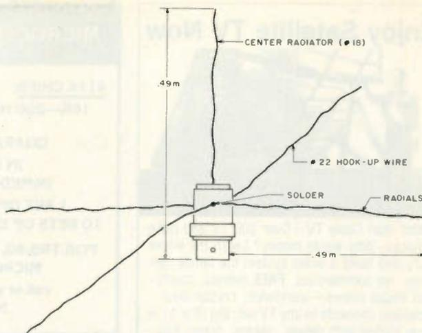
Fig. 1. The Flexi-Plane with BNC connector.
