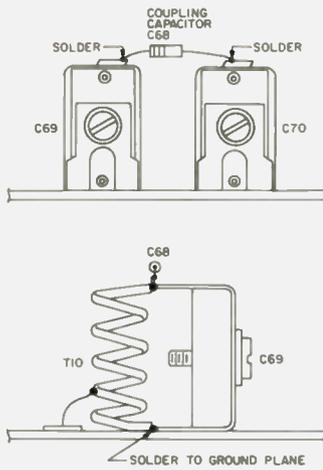
Fig. 7. Construction technique—2-section antenna filter and 5-section spurious filter.
