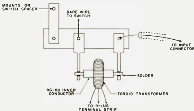
Fig. 4. Mounting the current transformer.
