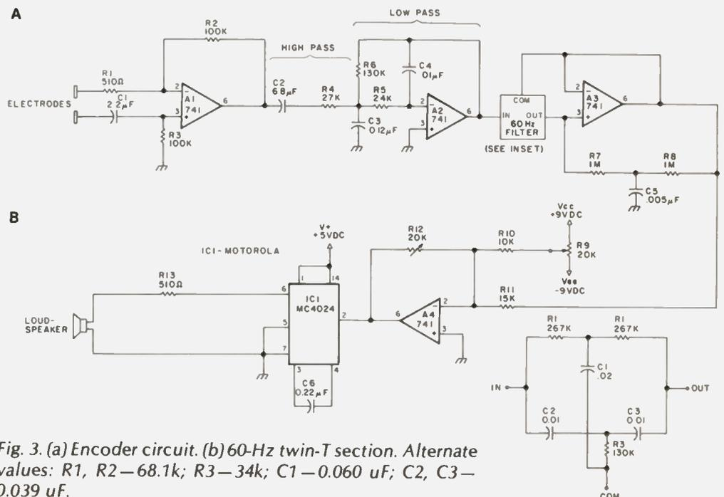
Fig. 3. (a) Encoder circuit. (b) 60-Hz twin-T section. Alternate values: R1, R2—68.1k; R3—34k; C1—0.060 uF; C2, C3—0.039 uF.
