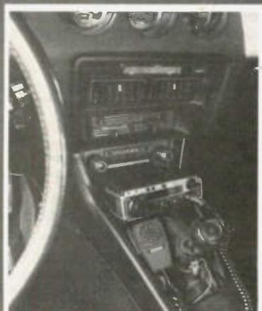
IC-280 control head mounted in Datsun 280Z
