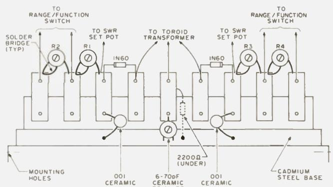
Fig. 5. Wiring diagram, nine-lug terminal strip.
