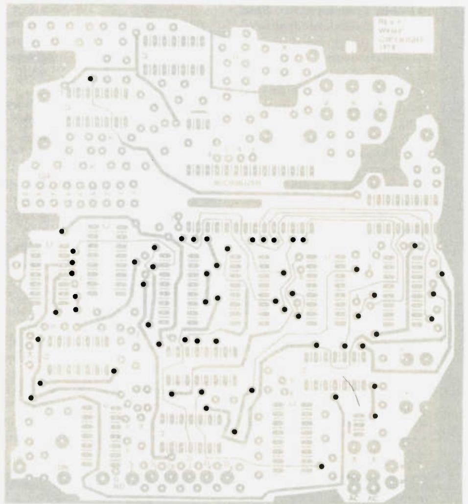
Fig. 7. “Z”-wire placement, along with method of installation.
