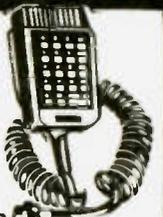
**YAESU YM-2500 keyboard mic for the CPU-2500R**
