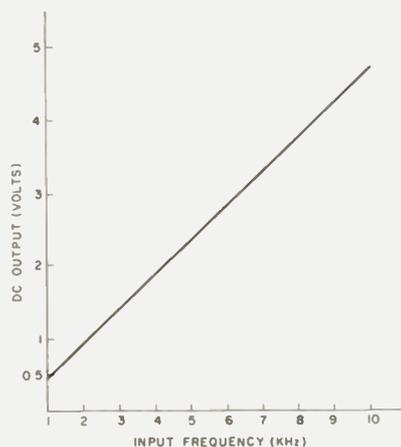
Fig. 5(b). Output voltage versus input frequency.
