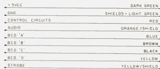
Fig. 7. Corresponding signal-to-cable colors used in the Radio Shack 24-conductor microphone cable. The end with the connectors should be placed in the Micoder.
