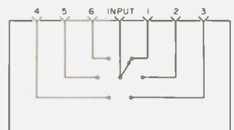
Fig. 1. Simplified wiring diagram, B&W Model 595 coaxial switch. Note: Automatic grounding (not shown) of all unused positions is incorporated.
