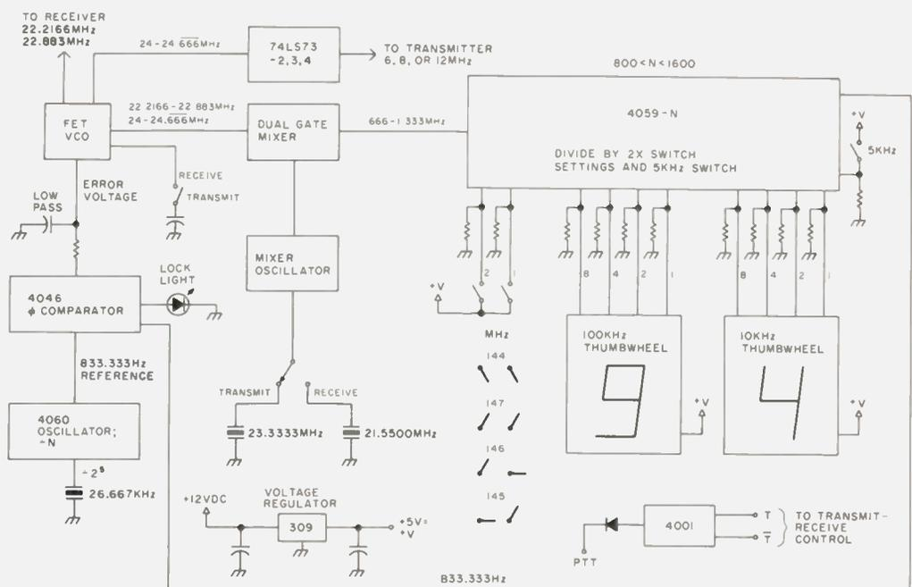
Fig. 2. 2m synthesizer block diagram.
