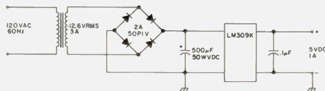
Fig. 2. 5 volts at 1 Amp dc power supply.
