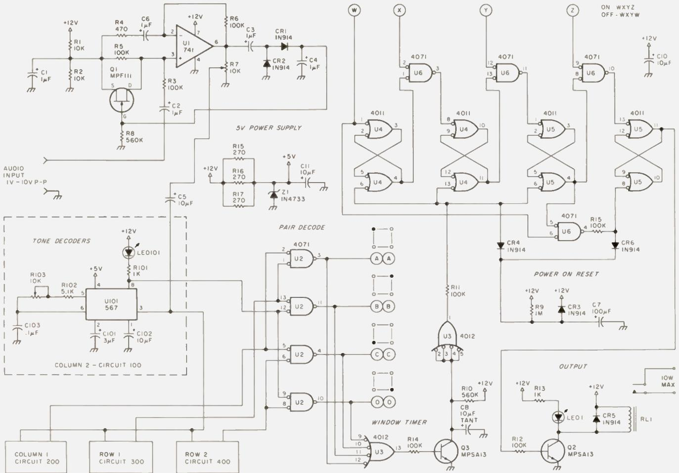
Fig. 1. Schematic of remote-control decoder. All resistors 1/4 W, 5% unless otherwise stated. On all ICs, connect pin 14 to +12 volts and pin 7 to ground unless otherwise stated. Circuits 100, 200, 300, and 400 are identical except that part 101 becomes 201, etc.
