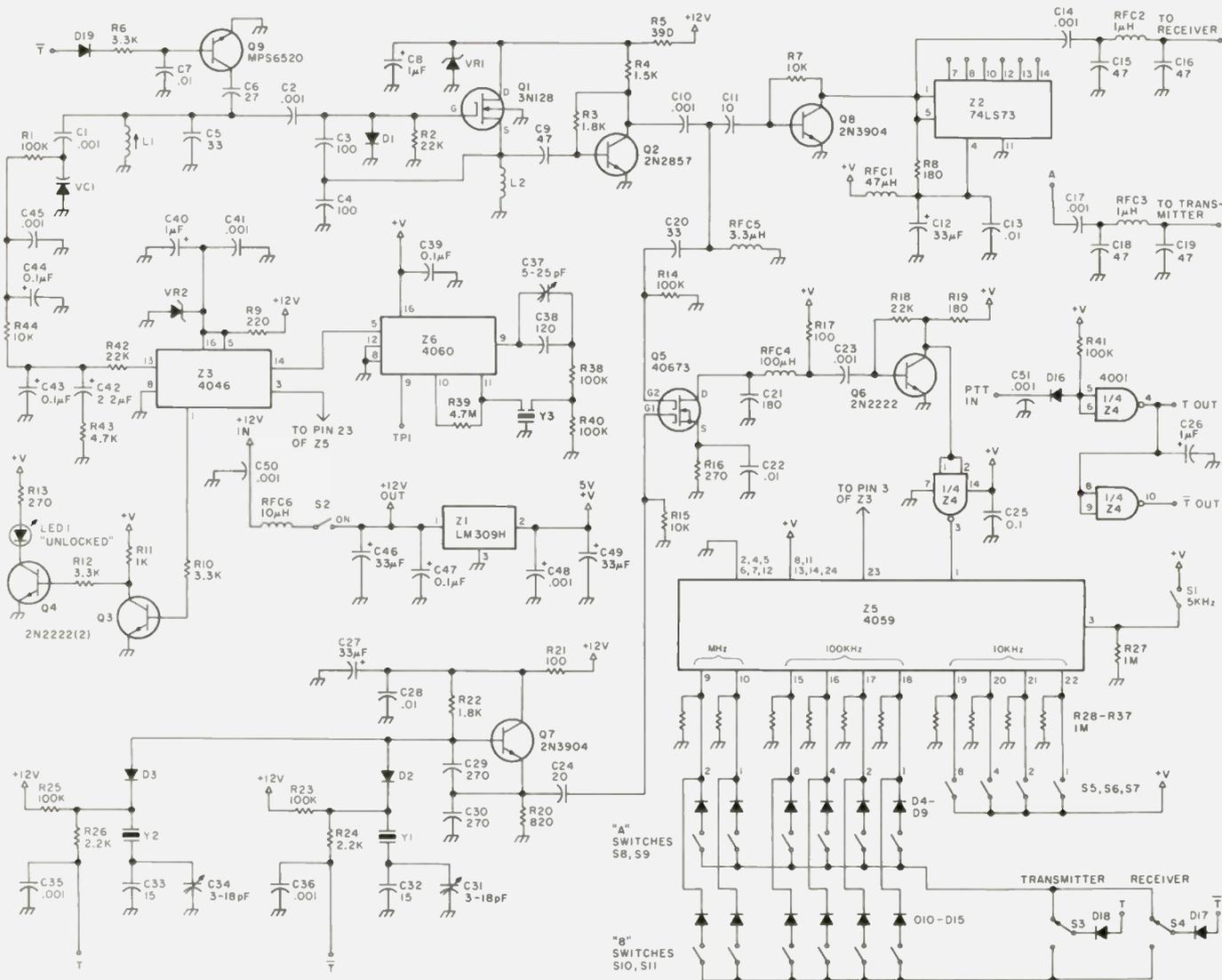
Fig. 1. 2m synthesizer schematic diagram.
