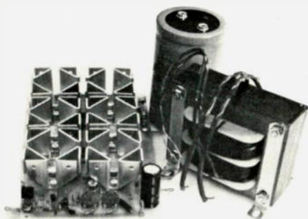
The original hefty 12V supply, and still going strong... one look at the specs will tell you why this has been our longest-running kit. Handles 8A continuous, and 12A (!) with a 50% duty cycle. Features foldback current limiting, crowbar overvoltage protection, RF suppression, adjustable output 11-14V, heavy-duty custom wound transformer, and much more.
