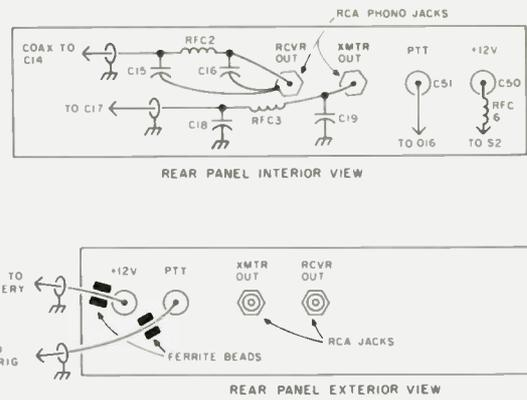
Fig. 8. Rear panel connections.
