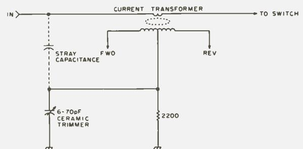
Fig. 3. Capacitive voltage divider with current transformer.
