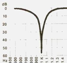
**NOTCH FILTER PERFORMANCE ADJUSTED TO 1 kHz POINT.**
