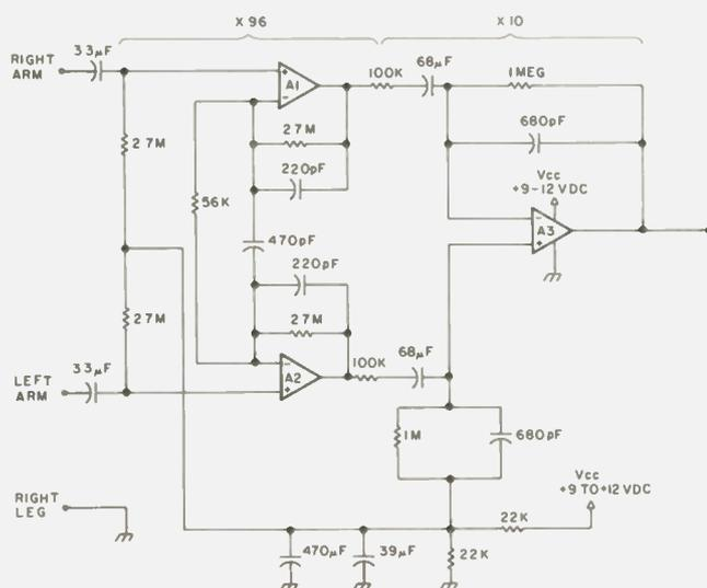
Fig. 1. Typical ECG preamplifier.
