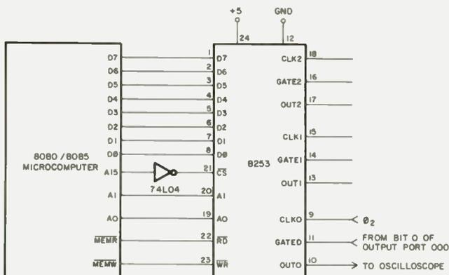
Fig. 1. Interface circuit between a 8253 programmable interval timer and an 8080/8085 microcomputer. The 8253 chip uses four locations of memory in this memory-mapped interface circuit.
