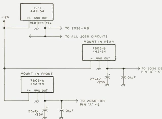
Fig. 3. 7805 voltage regulator schematic.
