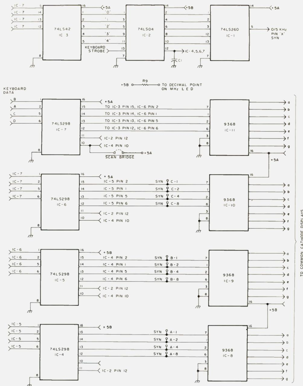
Fig. 1. 2036-DB Display Board schematic.
