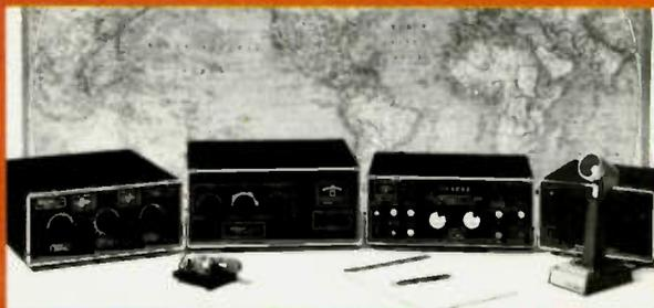
The ASTRO 102BX with it's companion PSU-6 Power Supply, 1500Z Linear Amplifier and ST-2A Antenna Tuner provides a matched and highly efficient 1500 watt PEP or 1000 watt CW complete station to be complemented by a great Swan antenna.
