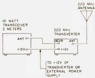
Fig. 1. Transverter connections.
