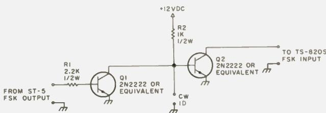
Fig. 1. An FSK relay for the TS-820S.
