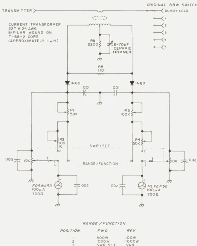
Fig. 2. Swattmeter schematic.
