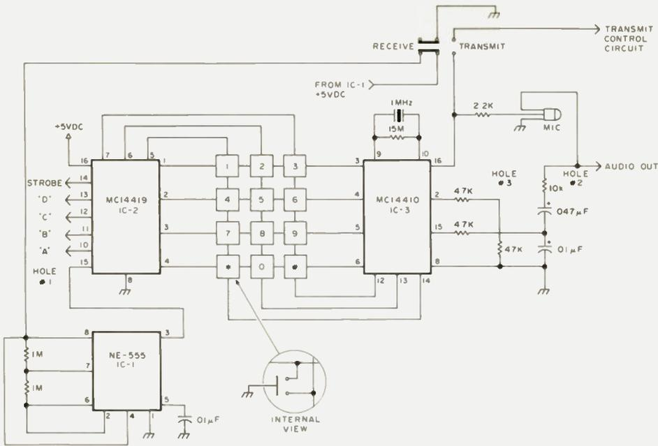
Fig. 2. 2036-MB MicBoard schematic.
