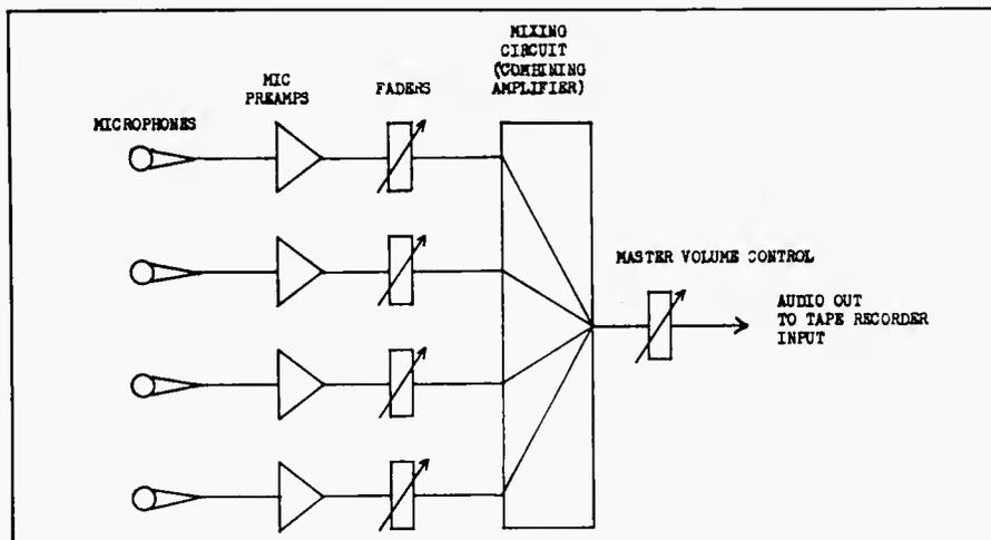
Figure 1. Signal paths in a typical mono mixer.
