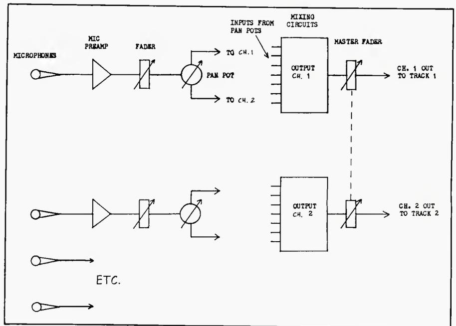
Figure 2. Signal paths in a typical 2-channel mixers.
