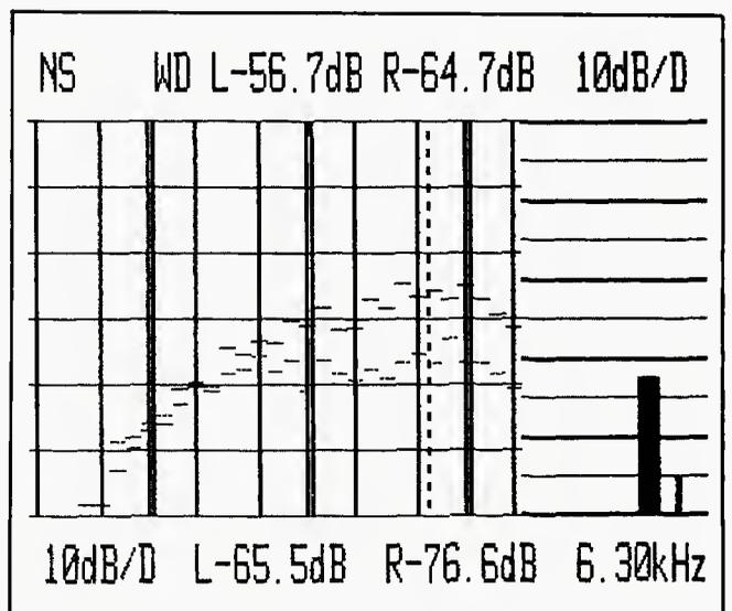
Figure 5. S/N analysis, without and with Dolby B, at 3 3/4 ips (A) and at 1 7/8 ips (B).
