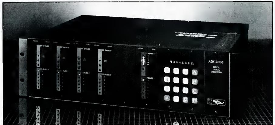
Delay settings range from 10 microseconds to 261 milliseconds (1048 milliseconds optional) in increments of one micro- or millisecond. Dynamic range is at least 100 dB (A-weighted, no companding); THD plus noise is better than 0.1%; and frequency response is
