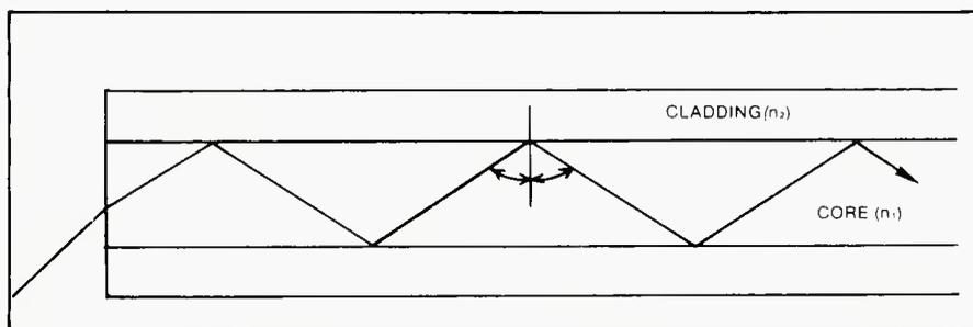
Figure 2. (top) Light entering from left into core with index  $n_1$ , reflected at the boundary with the cladding having index  $n_2$ . [page 21 from AMP] (bottom) various paths for light ray in different types of fiber optic cables. The core size and refractive index determine the light propagation characteristics of the fiber. [page 23 from AMP].
