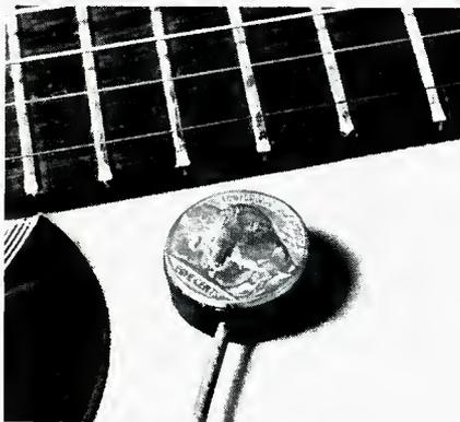
● The tiny P800 Buffalo pickup, with a Buffalo nickel as a lid, operates on an electret condenser principle and attaches to an instrument with removable adhesive tabs. It has its own power supply, which can be attached to the performer's belt or clipped to a mic stand. Power for the unit's pre-amp comes from a 9-volt transistor radio type of battery. It's equipped with a standard phone jack. Model P800Z features balanced output and an XLR-3 connector.
