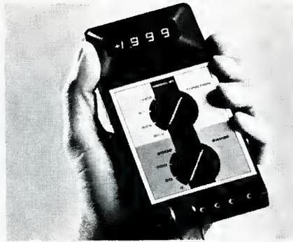
● A palm-sized hand-held digital millimeter, model 21, measures capacitance along with a.c. volts, d.c. volts, and resistance. The instrument has four d.c. voltage ranges with 1 mV resolution; four a.c. voltage ranges with 1 mV resolution; four resistance ranges with 1 ohm resolution; four capacitance ranges with 1 pFd resolution. It has l.e.d. displayed 3½ digit readout (up to 2,000 counts) and simplified five step calibration. Model 21 operates from four rechargeable NiCad batteries.
