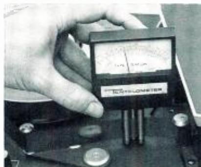
● Magnetic recording tape of all widths can be measured for dynamic or static tension with hand-held model T2 Tentelometer. Tape tension on video machines can be accurately set while the machine is operating; head wear is optimized and transient problems can be detected. The unit is self contained, requires no external power, operates in any orientation and reads both in ounces and grams of tension. Models are available in 5, 12, or 20 ounce full scale ranges, complete with carrying cases.
