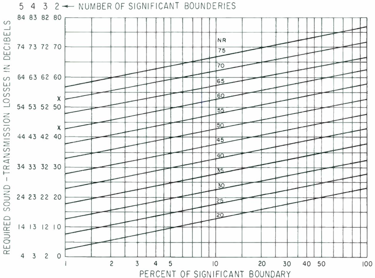
Figure 3. This graph provides quick determination of the required sound transmission losses of elements in a composite barrier to provide various noise-reductions. The abscissa refers to the per cent area of an individual element.
