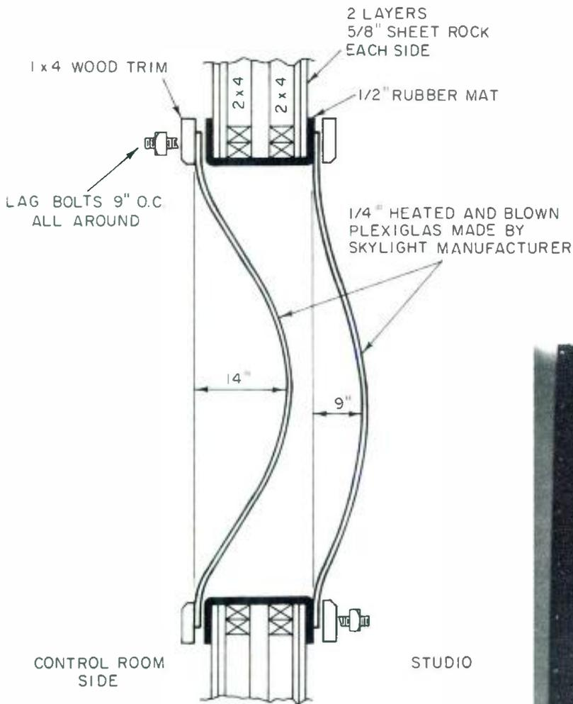
Figure 2. The construction drawing side view. From the front, the window specified is 6-feet, 4-inches across, and 5 feet, 4-inches top to bottom. The window has good dispersion and high rigidity:weight ratio. The windows cost \$85 each and total cost including construction was \$200.
