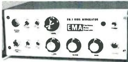
*rier*. The *blend* control adjusts the percent of modulation by selecting the desired mixture of the signal and the signal-carrier modulation products. Using a sum and difference principle, the unit can modulate complex harmonics, such as the human voice. If no carrier is provided, the signal is automatically routed to the carrier input, creating a frequency doubler effect.
