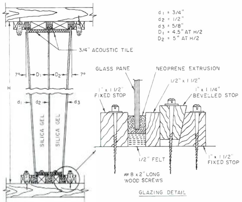
Figure 1. Details of construction of triple-pane sound-retardant window used in monitoring room. The values for the glass thicknesses shown on the figure refer to a large (8 feet x 16 feet) window in a Hollywood motion picture scoring stage.
