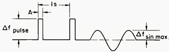
Figure 2. The pulse form for measuring dynamic characteristics.
