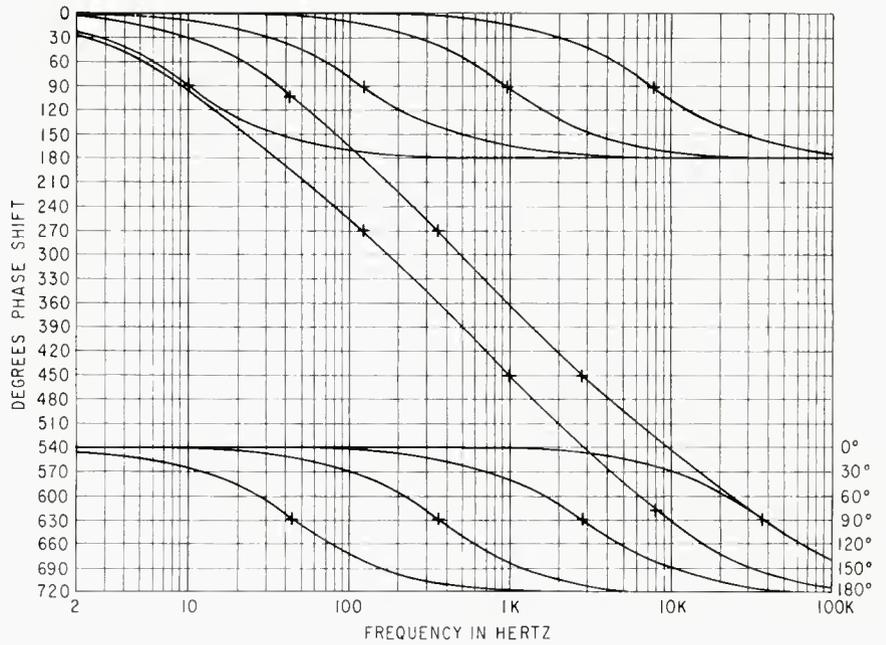
which the networks alternately center. For this to happen, the combined rate of phase shift, when adjoining networks in the other channel are, in this case, at 39 degrees and 141 degrees, must add up to the same rate produced by the one network just going through 90 degrees in this channel.
