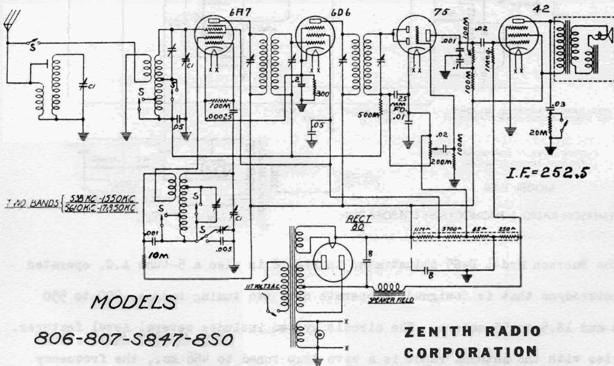
With the switch S in the short wave position, the pre-selector becomes inoperative and a special primary is cut in for the detector coil. At the same time a portion of the detector coil and of the oscillator coil is shortcircuited so that the tuning system responds to a range of higher frequencies. The rest
