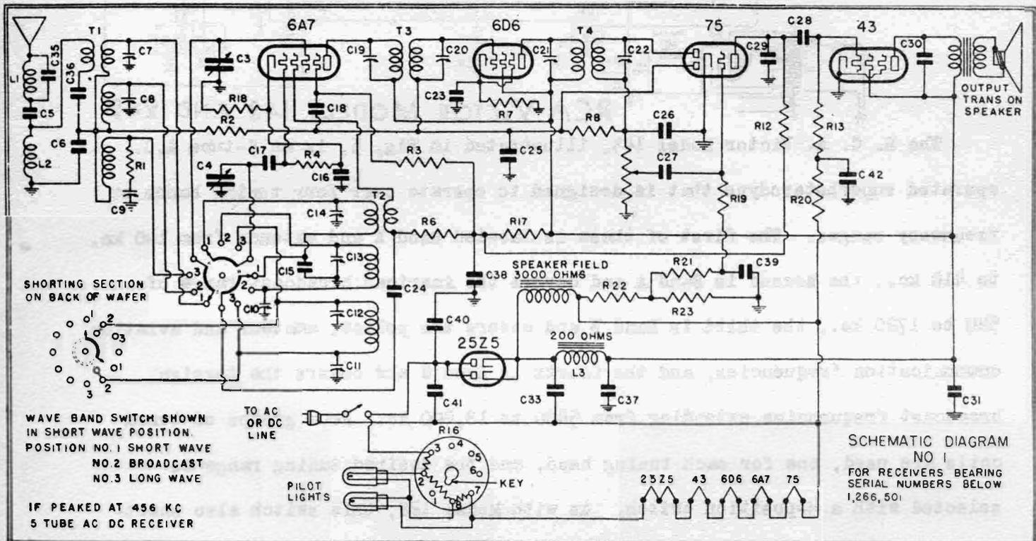
The Emerson Radio illustrated in Fig. 6, is a 5 tube, 3-band, long wave,
