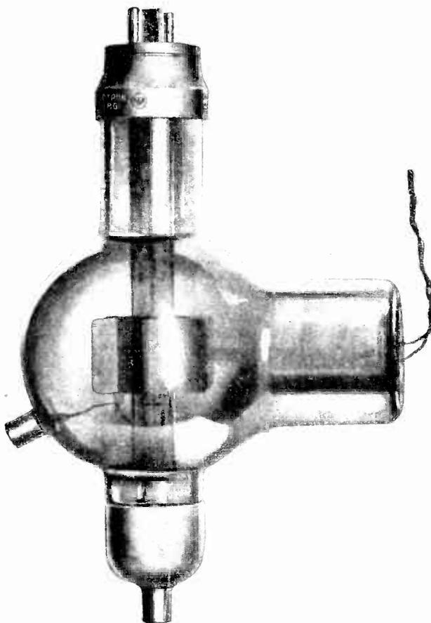
FIG. 11 - PHOTOGRAPH OF A TYPE UV-861 TUBE
