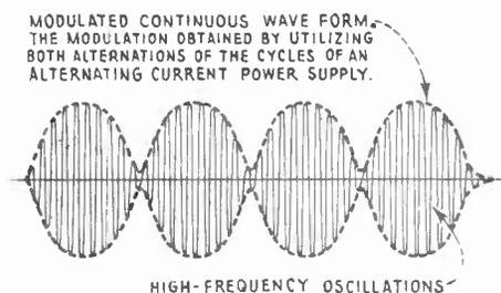
FIG. 6 - MODULATION PRODUCED BY RECTIFYING BOTH HALVES OF AN A-C POWER SUPPLY
