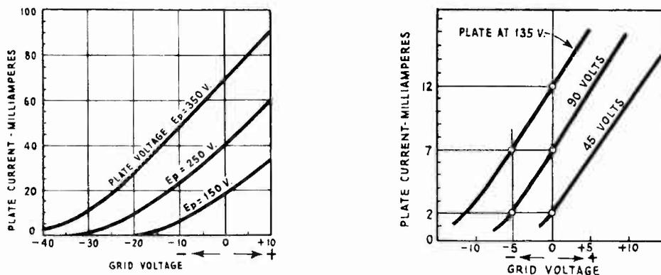
FIG. 16 - CHARACTERISTIC CURVES OF A UX-210 TUBE
