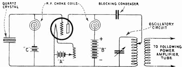
FIG. 2 - 100 WATT TUBE IN A CRYSTAL-CONTROLLED CIRCUIT
