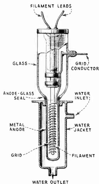
FIG. 13 - TUBE AND WATER-JACKET
