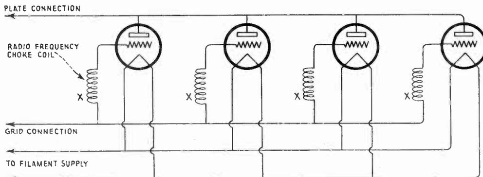
FIG. 10 - WHERE R-F CHOKE COILS MIGHT BE PLACED IN GRID CIRCUITS
