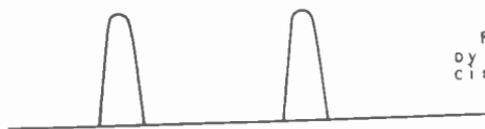
Fig. 38B. The current passed by the rectifier of this same circuit.
