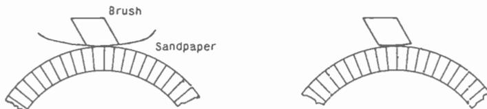
Fig. 22 Showing how the wrong curvature may result unless the sandpaper is held properly.
