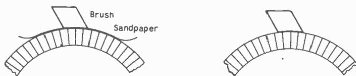
Fig. 21 Illustrating the method of using sandpaper to fit the brush to the curvature of the commutator.
