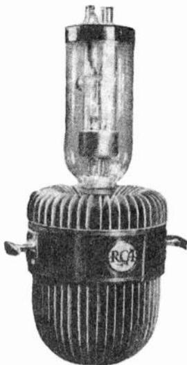
Fig. 8 A water-cooled tube with cooling fins attached.
