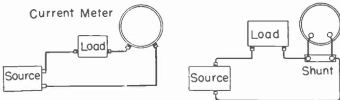
Fig. 1.—Connections for current-indicating meters.
