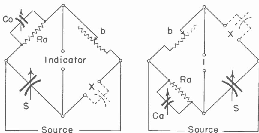
Fig. 14.—A Schering bridge for capacitance measurement.
