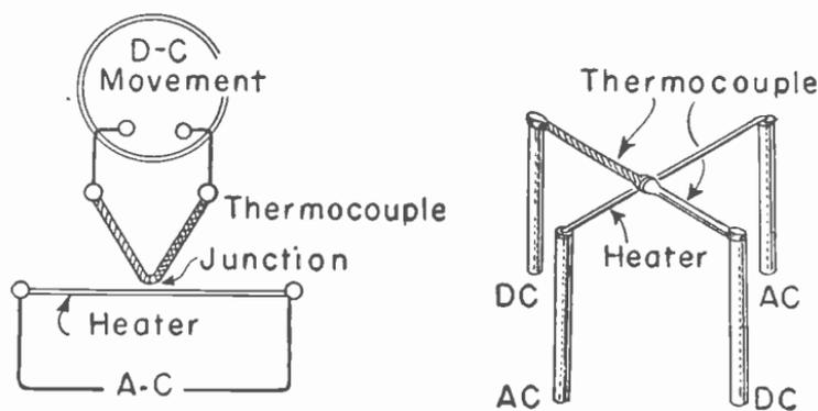
Fig. 20.—The principle of the thermocouple meter.
