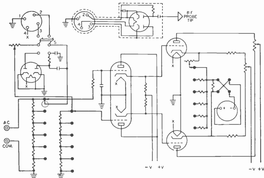
Fig. 20.—The Triplet bridge circuit as arranged for use with diode input during measurement of alternating potentials.
