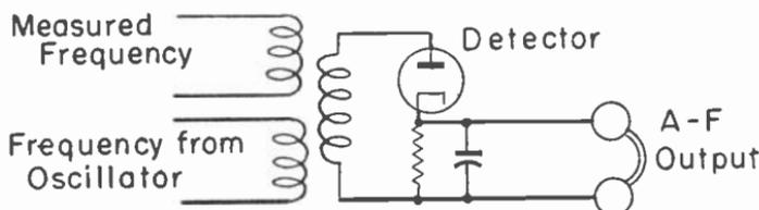
Fig. 17.—Basic principle of the heterodyne frequency meter.
