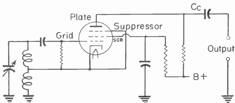
Fig. 10.—One type of electron coupled oscillator.
