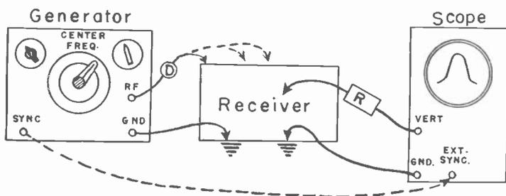
Fig. 25.—Connections for a frequency-modulated signal generator.
