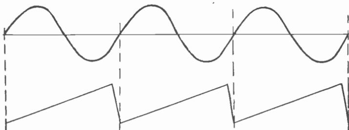
*Fig. 7.—Vertical and horizontal deflecting potentials continue, keeping in step or in synchronization with each other.*
