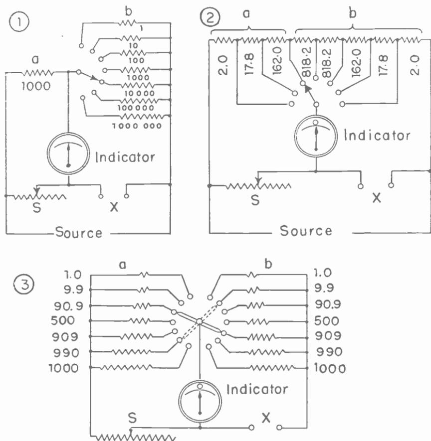
Fig. 7.—Connections and resistance values for ratio arms.
