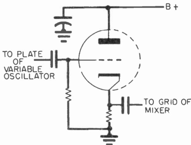
Fig. 13.—The cathode follower in the output circuit of the r-f oscillator in a Hickok signal generator.
