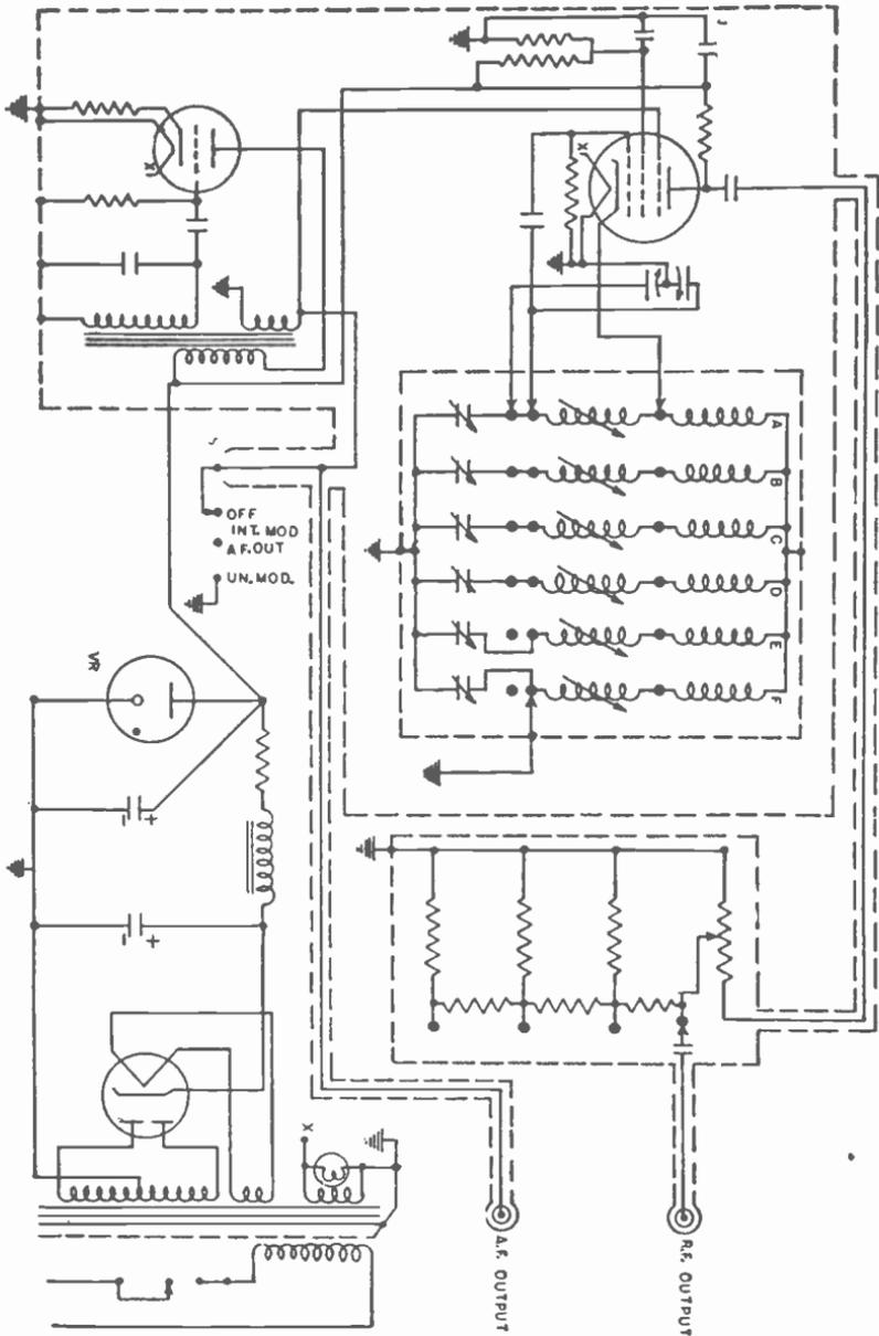
Fig. 12.—The complete schematic circuit diagram for the Triplet signal generator.
