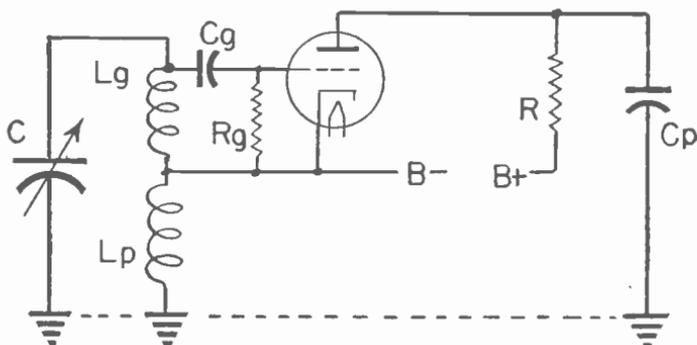
Fig. 6.—One arrangement of the Hartley oscillator circuit.
