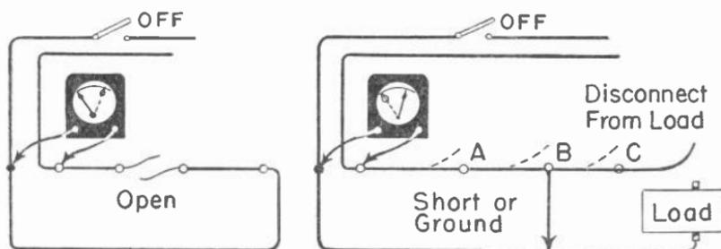
Fig. 7.—Locating circuit troubles with a self-contained tester.
