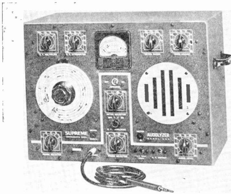
Fig. 1.—The Supreme Audalyzer, showing meter of electronic voltmeter, frequency measuring dial, speaker grille, test probe, and controls.
