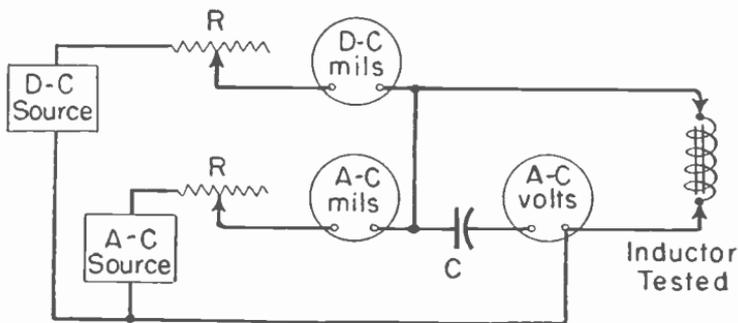
Fig. 11.—An inductance testing circuit with which direct current is put through the inductor during measurement.
