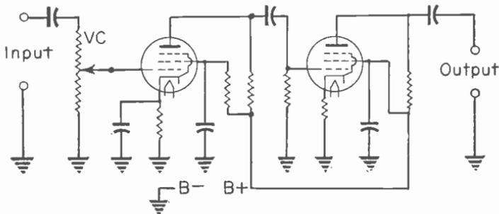
Fig. 5.—An untuned amplifier such as used with crystal or detector types of probes.
