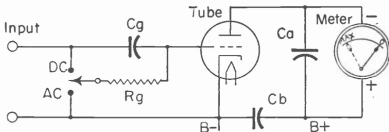
Fig. 3.—The grid rectification or grid leak electronic voltmeter.
