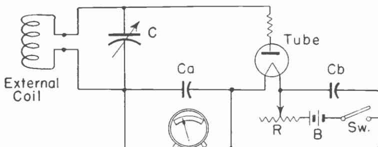
Fig. 16.—A wavemeter with tube rectifier and current meter in the resonance indicator
