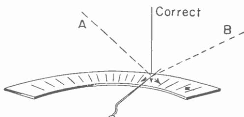
Fig. 6.—The effects of parallax when reading a meter.
