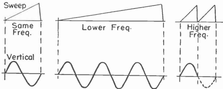
Fig. 15.—Relations between sweep frequencies and vertical frequencies.
