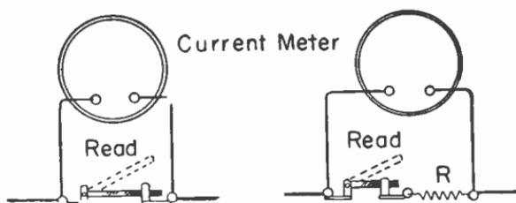
Fig. 4.—Protective devices for current meters.
