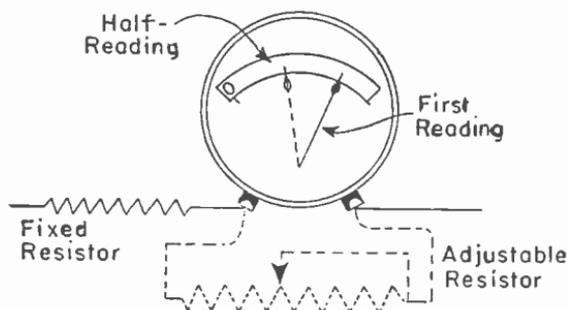
Fig. 15.—A method for measurement of meter resistance.
