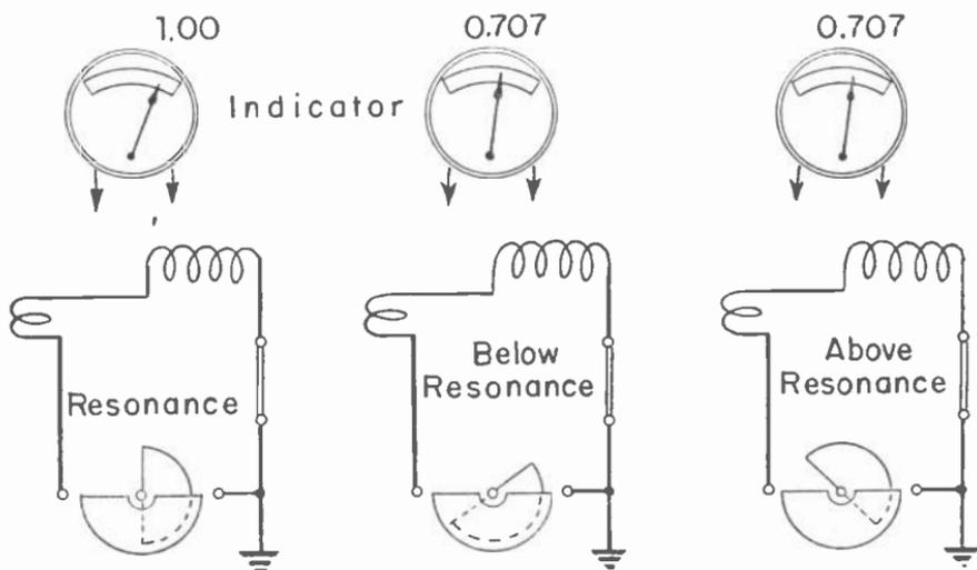
Fig. 12.—High-frequency resistance measured by reactance variation.
