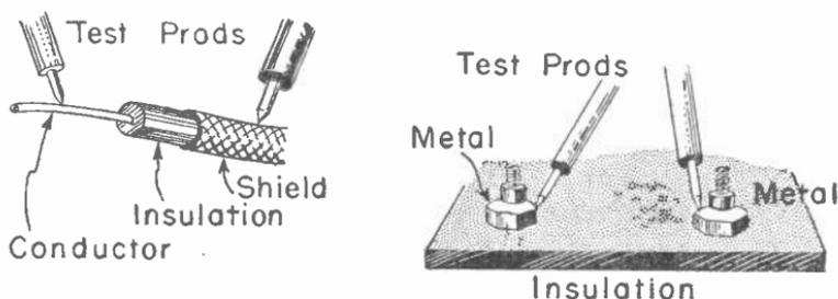
Fig. 4.—Checking the resistance of insulation.
