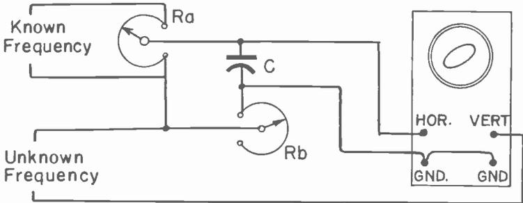
Fig. 19.—A phase-splitting circuit used for frequency comparisons
