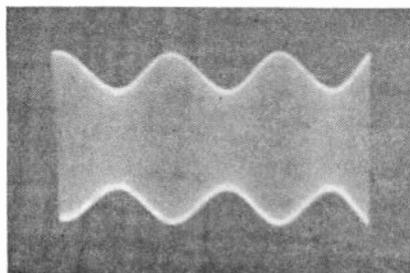
Fig. 15.—Smaller percentage modulation.
