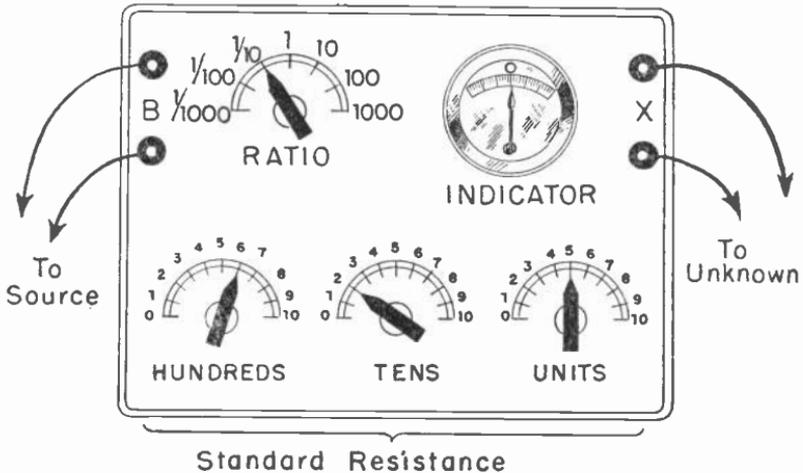
Fig. 1.—The panel controls of a resistance bridge.
