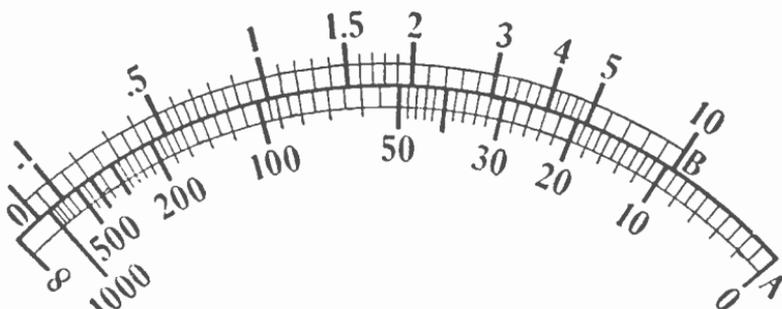
Fig. 9.—A shunt-resistance scale (top) and a series-resistance scale (bottom) for the same instrument.
