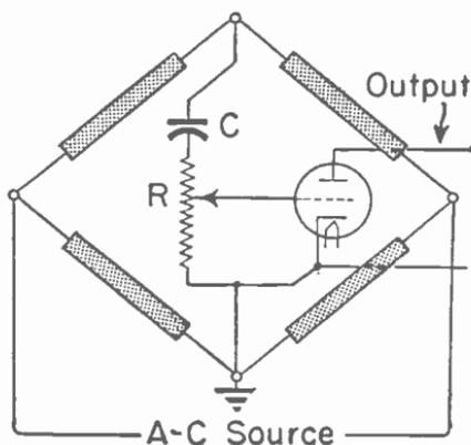
Fig. 21.—An amplifier tube in the indicator circuit.
