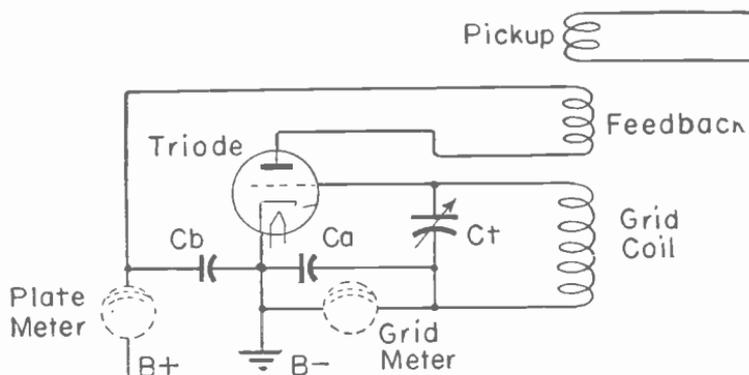
Fig. 2.—A simple oscillator with tickler feedback.
