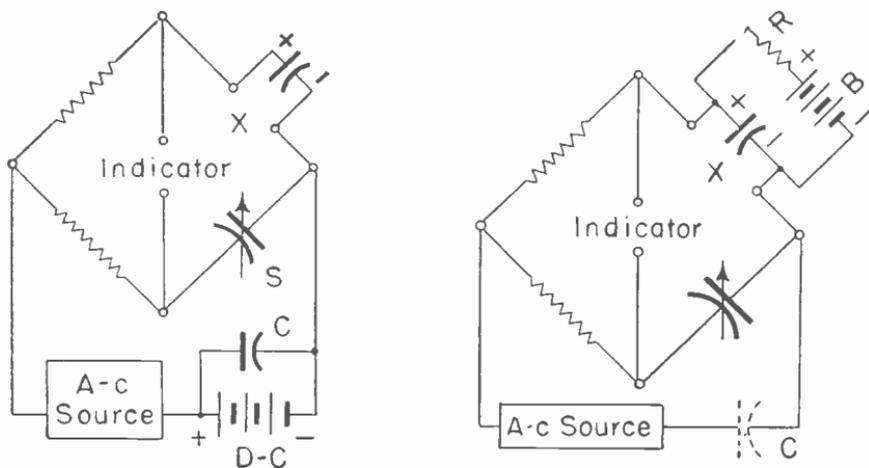
Fig. 15.—Testing electrolytic capacitors on capacitance bridges.
