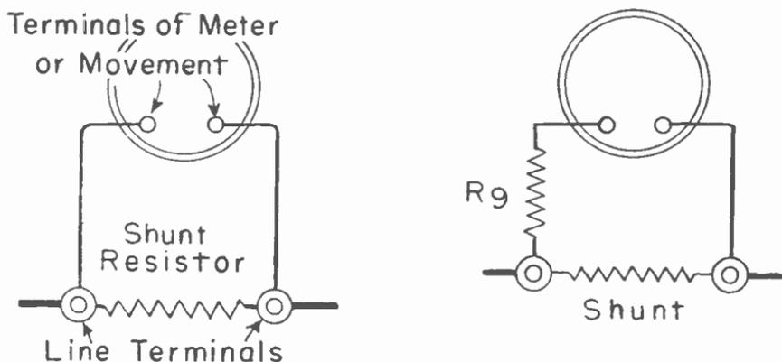
Fig. 12.—Connections of shunt resistors for current meters.
