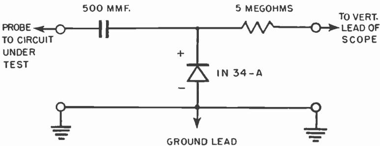
A circuit for a small efficient probe good from 50 kc to 250 megacycles is shown.
