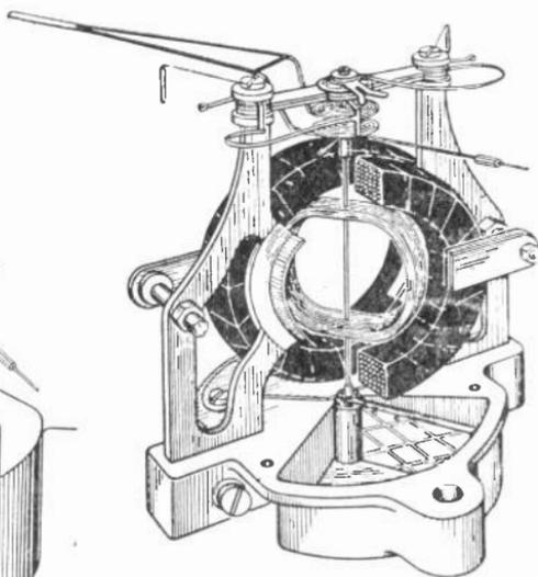
Fig. 23.—The principle of the dynamometer instrument.
