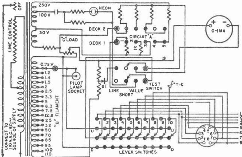
Fig. 5.—The complete wiring diagram for one type of Triplet tube tester.
