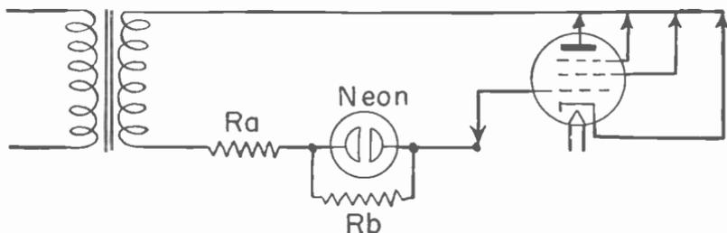
Fig. 10.—One method of testing for short-circuited elements.
