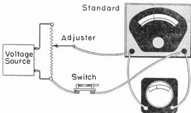
Fig. 11.—Connections for calibration of a voltmeter.
