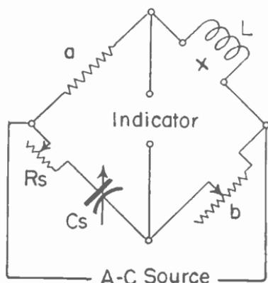
Fig. 19.—The Hay bridge for inductance measurement.
