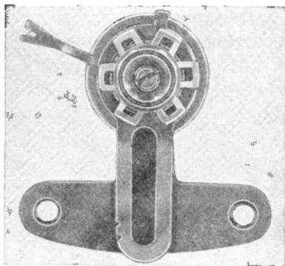
Fig. 13.—A zero adjuster with the jewel screw showing in the center.
