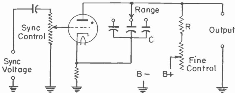
Fig. 9.—A sweep oscillator employing a gas triode.
