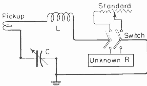
Fig. 10.—High-frequency resistance measurement by substitution.
