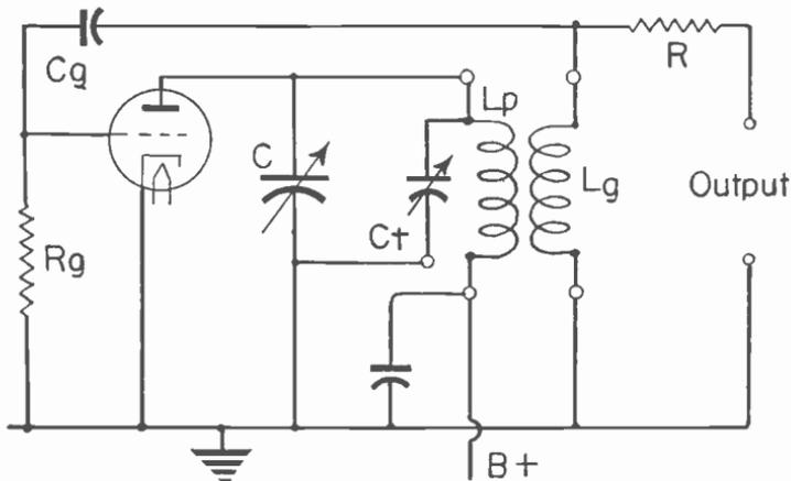
Fig. 5.—A tuned plate oscillator with inductive feedback.
