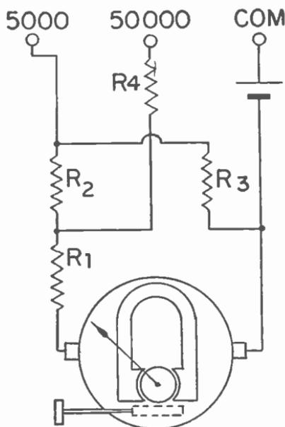
Fig. 5.—A Weston ohmmeter and its internal connections.
