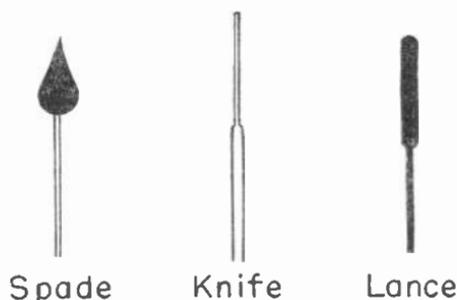
Fig. 11.—Shapes of pointers used in indicating meters.
