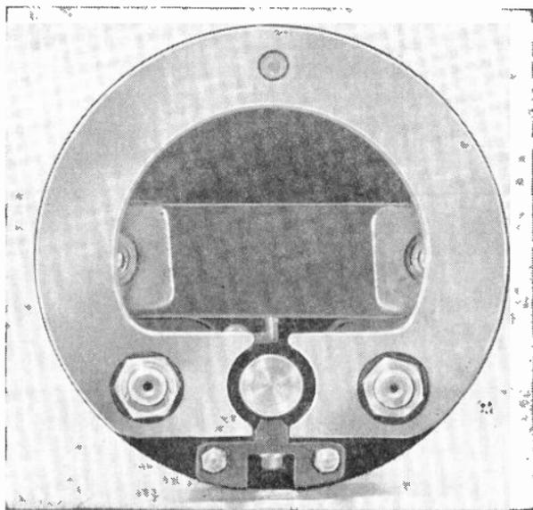
Fig. 6.—A cylindrical core of iron nearly fills the field space.
