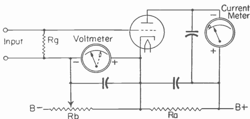
Fig. 5.—The circuit for one type of slide-back voltmeter.
