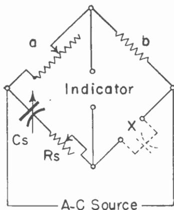
Fig. 11.—A series resistance type of capacitance bridge.
