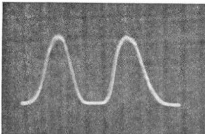
*Fig. 27.—Two resonance curves formed during one horizontal sweep.*
