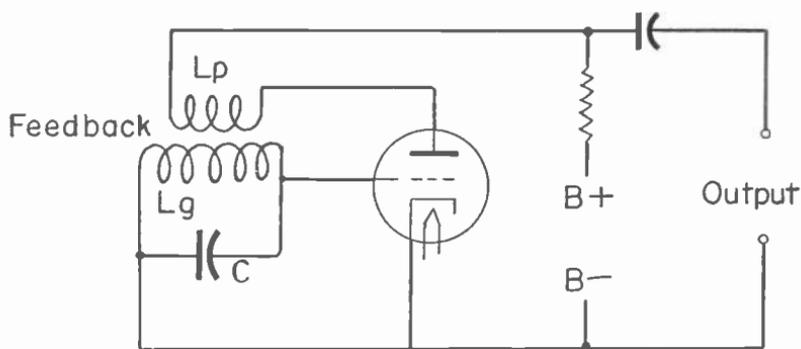
Fig. 2.—The elementary oscillator circuit.
