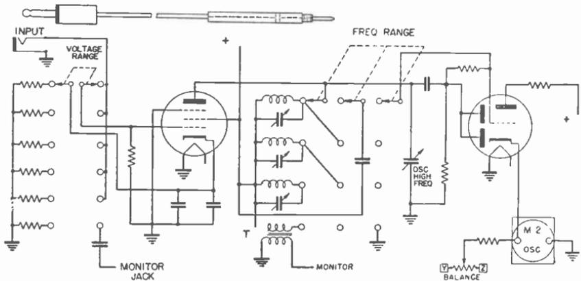
Fig. 10.—Simplified diagram of the amplifier and electronic voltmeter for frequencies between 0.6 and 15 mc in the Traceomate.
