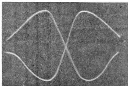
Fig. 36.—The crossed curves used for discriminator alignment.
