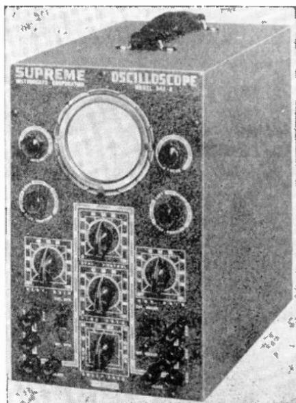
Fig. 11.—A Supreme Instruments oscilloscope with all controls and connections on the front panel.
