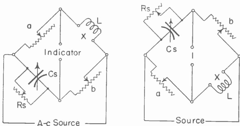
Fig. 17.—The Maxwell bridge for measurement of inductance.
