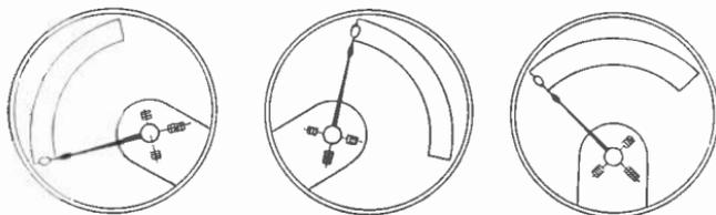
Fig. 16.—Positions in which a movement is balanced.
