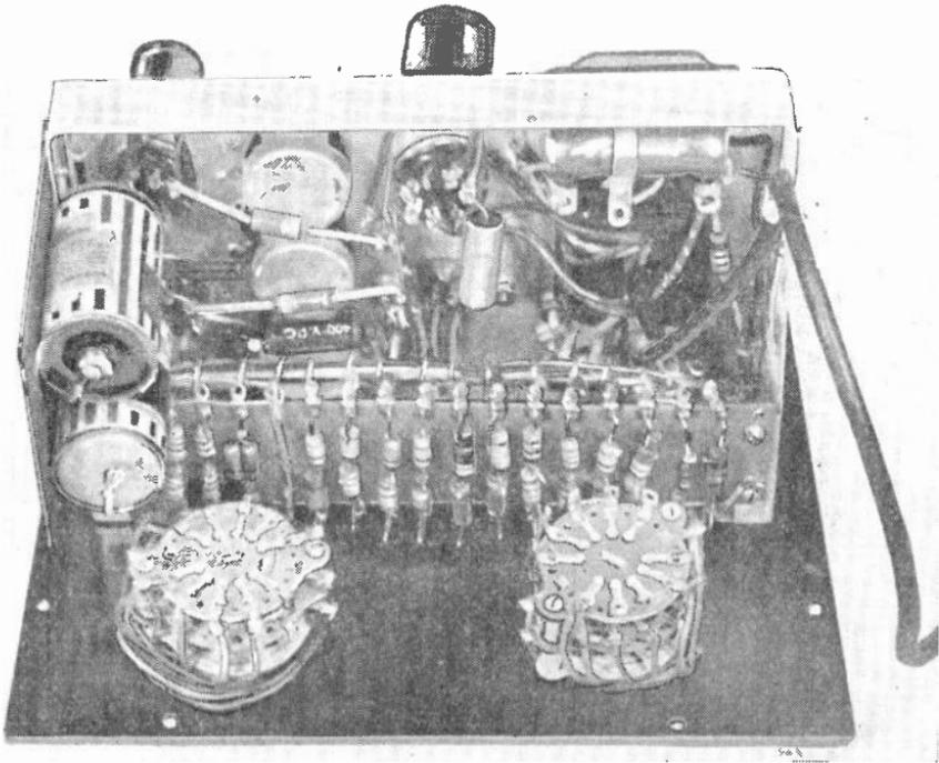
Fig. 2.—The parts inside of an electronic voltmeter.
