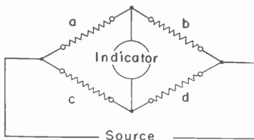
Fig. 6.—The fundamental bridge circuit.
