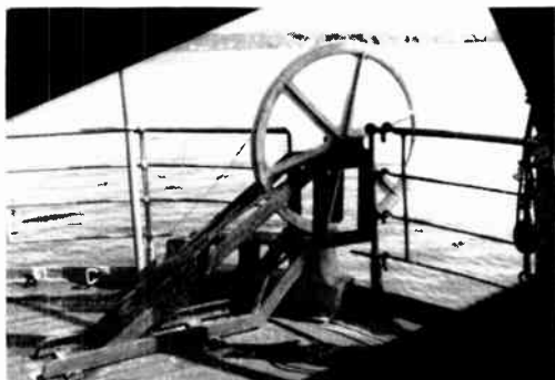
Stern sheave on starboard quarter over which cable was paid out from cable ship
