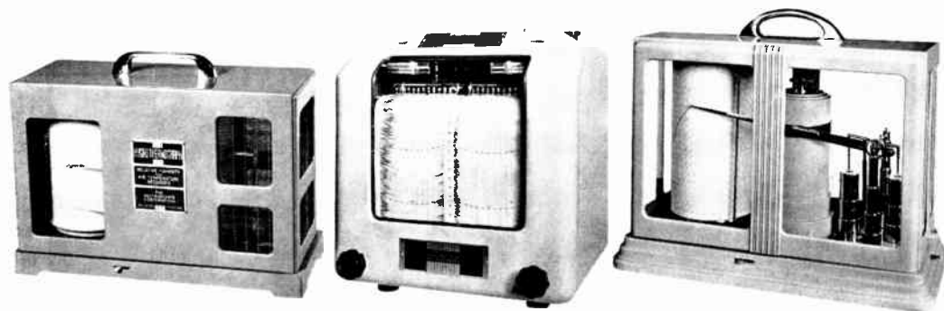
Typical meteorological instruments used to record weather data. Relative humidity and air temperature are charted by Hygro-thermograph at left. Wind direction and its velocity are recorded by meter shown in center. Pressure changes are plotted by Microbarograph at right. Illustrations by courtesy of The Instruments Corporation
