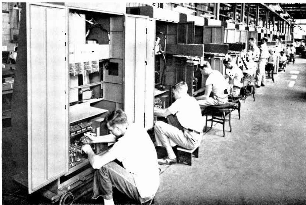
Figure 3. Large unit assembly line carrying printer-perforator tables
