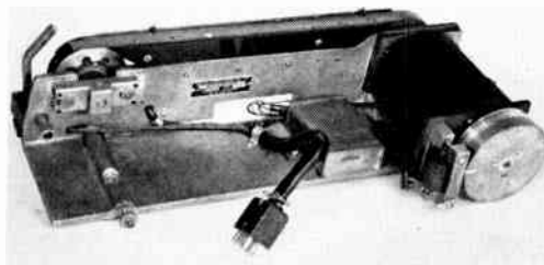
Figure 4. Stylus drive unit
