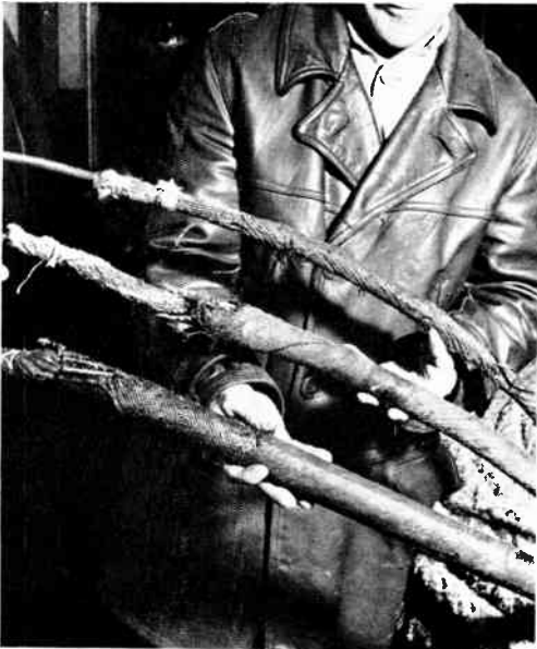
Jute and steel wire wrappings make up most of diameter of undersea cables
