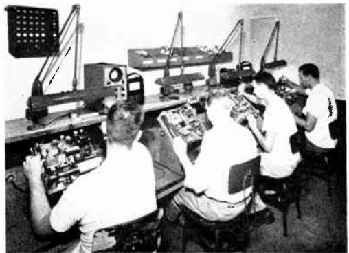
Figure 6. Testers at work on Desk-Fax units
