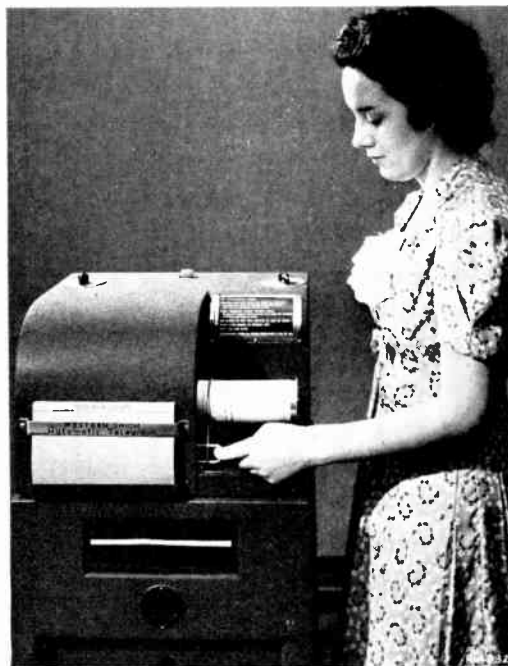
Figure 1. Telefax transmitter-recorder with optical scanning
