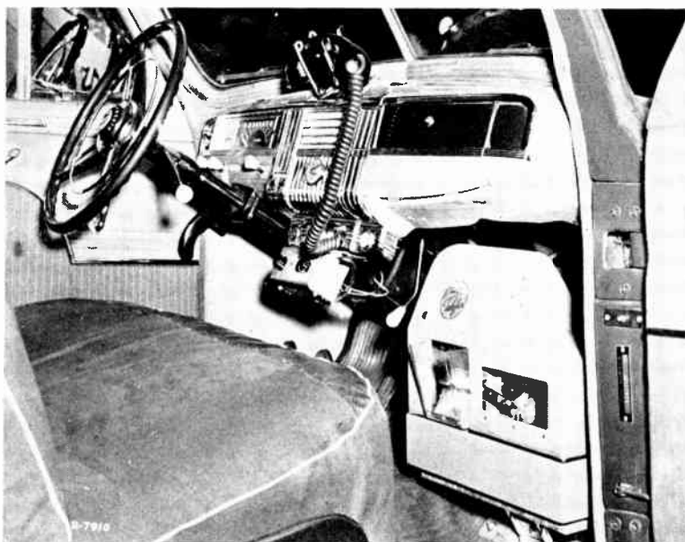
Figure 3. Telefax recorder for mobile delivery of telegrams
