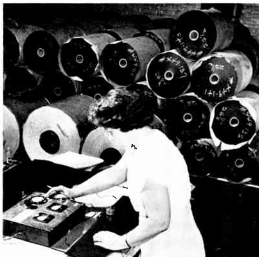
Electrical tests are made during production. Note unfinished stock rolls in background
