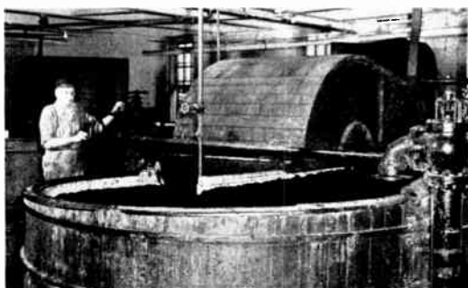
Manipulation of beater rolls governs fiber length and dispersion of conductive material
