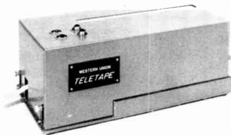
Figure 9. Transceiver with self-contained amplifier and control unit
