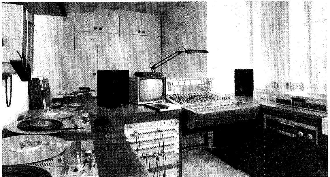
Control room with Studer 901, 2x A807, A710, A725 and A68.
