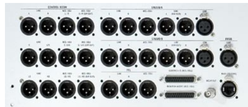
Monitoring inputs and outputs on the rear of the desk
