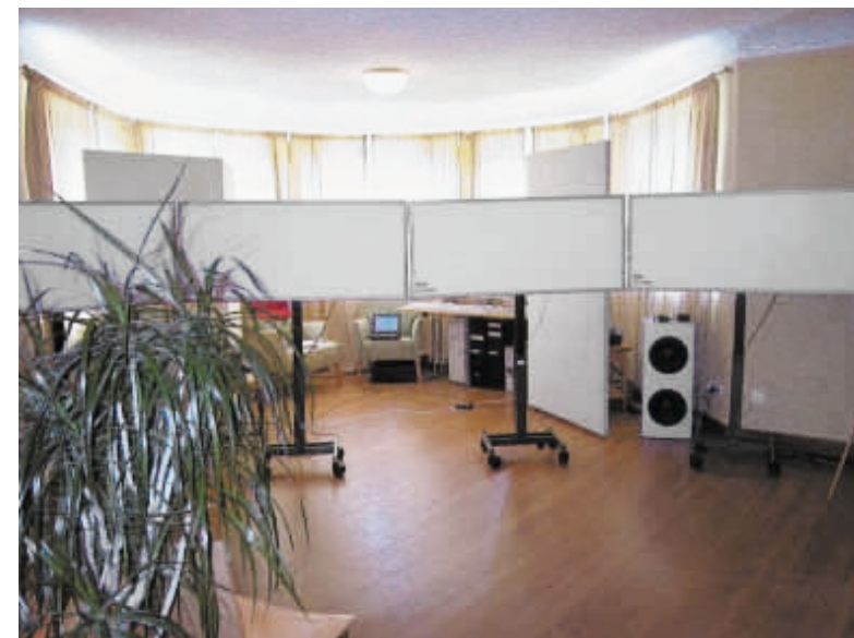
Figure 1: Four DML panels reproducing a total of 32 loudspeaker channels – an amazing sonic experience.
