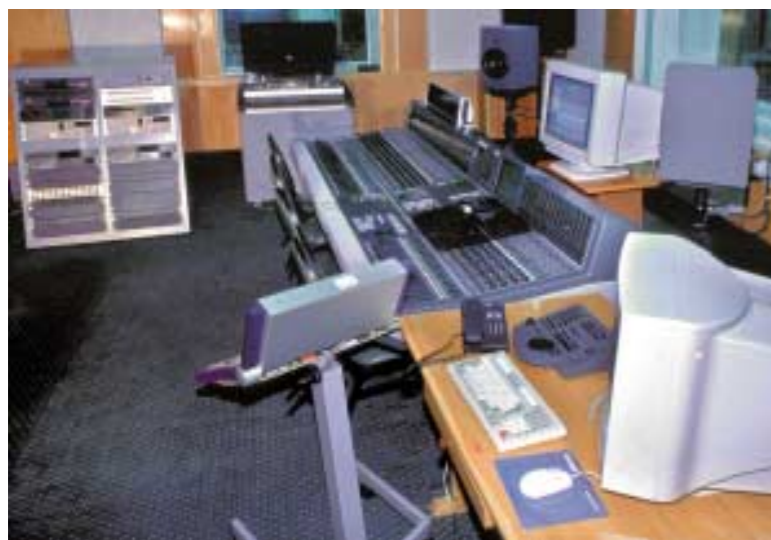
The first Studer D950 at ERTU was installed in Studio 45 for music recording
