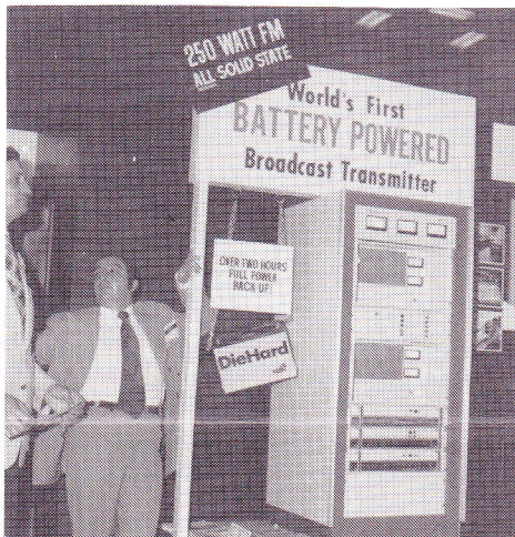
LOOKING IT OVER . . . Juan Gregorio, Sparta transmitter design engineer (left), spends some time with Angel Antonio Pachon of Bogota, Colombia, discussing the radically new battery operated Model 600BX 250-watt FM transmitter. —Sparta Photo
