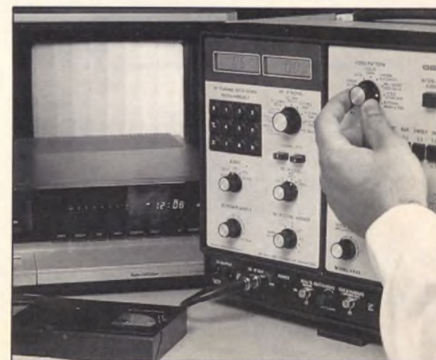
Fig. 6: Most VCR performance tests are done by using a television receiver connected to the VCR's output. Be sure that the television has a good tuner and frequency response.
