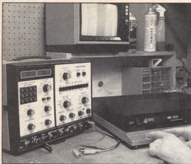
Fig. 7: Always terminate the VIDEO OUTPUT jack with a 75 Ohm resistor. This correctly loads the signal and prevents overshoots and rolloffs.
