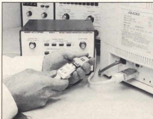
Fig. 1: A special adapter cable such as the 39G206 D 9-pin test lead lets you hook up directly to the RGB monitor.
