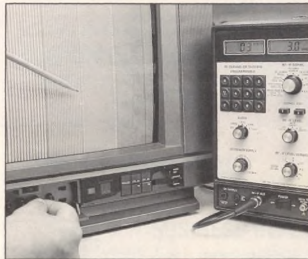
Fig. 5: The innovative VA62 video patterns provide a complete test of the circuits, and then help you isolate the problem by watching the TV screen.
