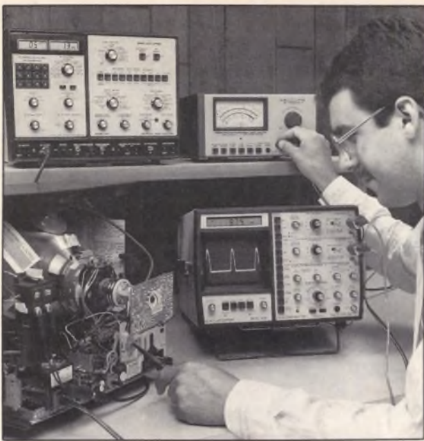
Fig. 2: By connecting an oscilloscope to the collector of the horizontal output transistor you can tell if the circuit is operating and monitor the effects of driving the circuit.
