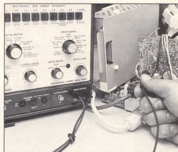
Fig. 2: The RG67 NTSC Video Monitor Adapter keeps digital or analog RGB monitors running and in sync while you troubleshoot with your VA62.
