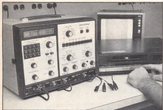
Fig. 6: The VA62 provides a series of patterns to test the performance of a VCR.
