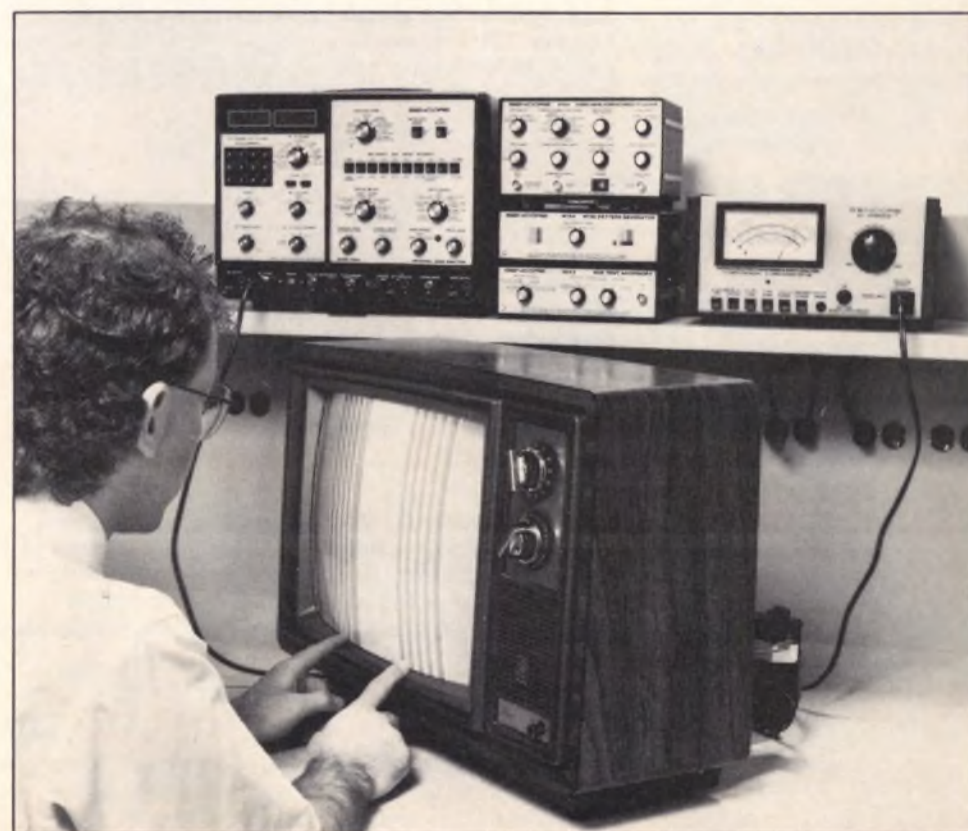
Fig. 7: Sharp response in the outside bars of the Chroma Bar Sweep pattern means the TV has the chroma bandpass needed for a good color picture.
