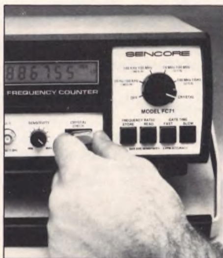
Fig. 2: Test crystals at their fundamental frequency in seconds.
