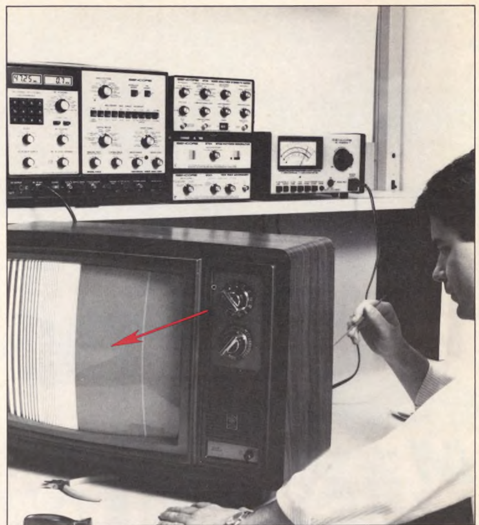
Fig. 4: Adjacent channel cable interference is easily minimized by simply adjusting the IF trap for minimum noise on the CRT while injecting the exclusive VA62 trap setting signal.
