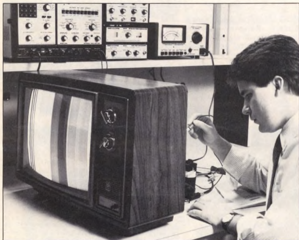
Fig. 6: When you inject a known-good troubleshooting signal and a good pattern does not appear on the CRT, you know the trouble is between your injection point and the CRT.
