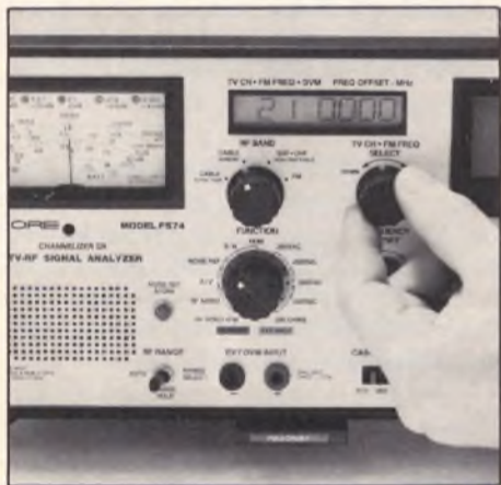
Fig. 5: Measure the signal-to-noise ratio, for any channel, even while it is in use!
