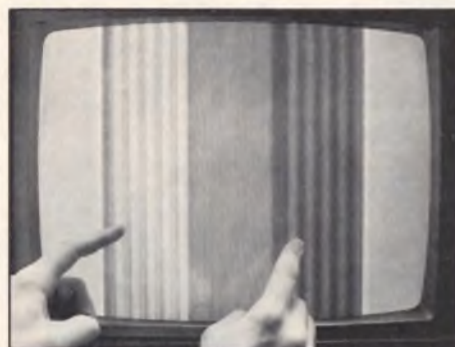
Fig. 2: The exclusive Sencore Chroma Bar Sweep gives you 3 dynamic parameter checks not available on any other pattern: saturation, hue, and 1 MHz frequency response.
