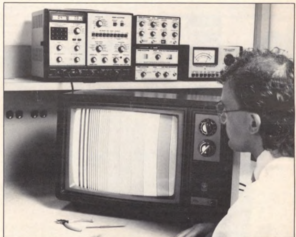
Fig. 1: Equally bright bars on the left two-thirds of the screen, (0-3 MHz), without smear or ringing, indicates good luminance channel, performance from the antenna input to the CRT.
