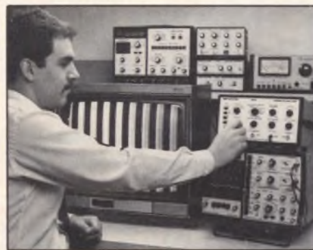
Fig. 2: A thorough performance check, with the ST66's special MTS signals, will help prevent call backs.
