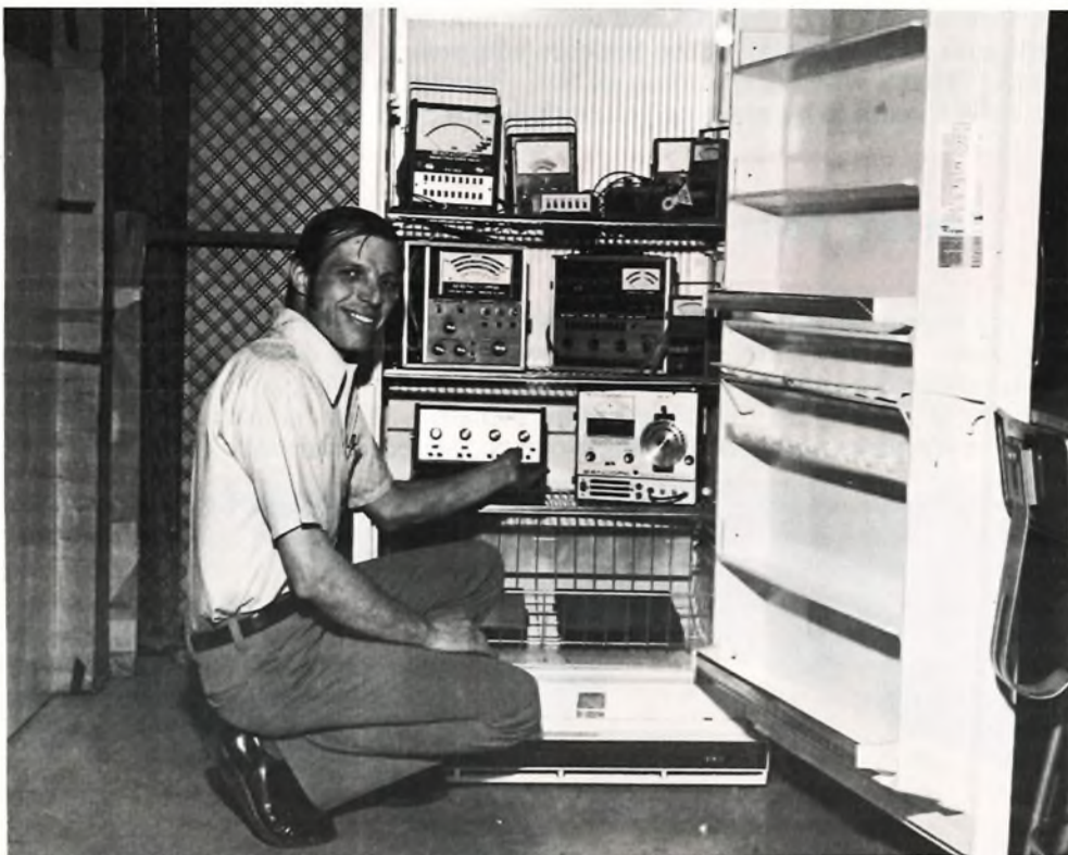
John subjects Sencore instruments to both freezing cold and extreme heat to assure you they will work anywhere, anytime you need them.
