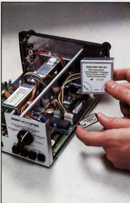
Field calibrate to full specifications (NBS traceable) with a simple module and ROM change.
