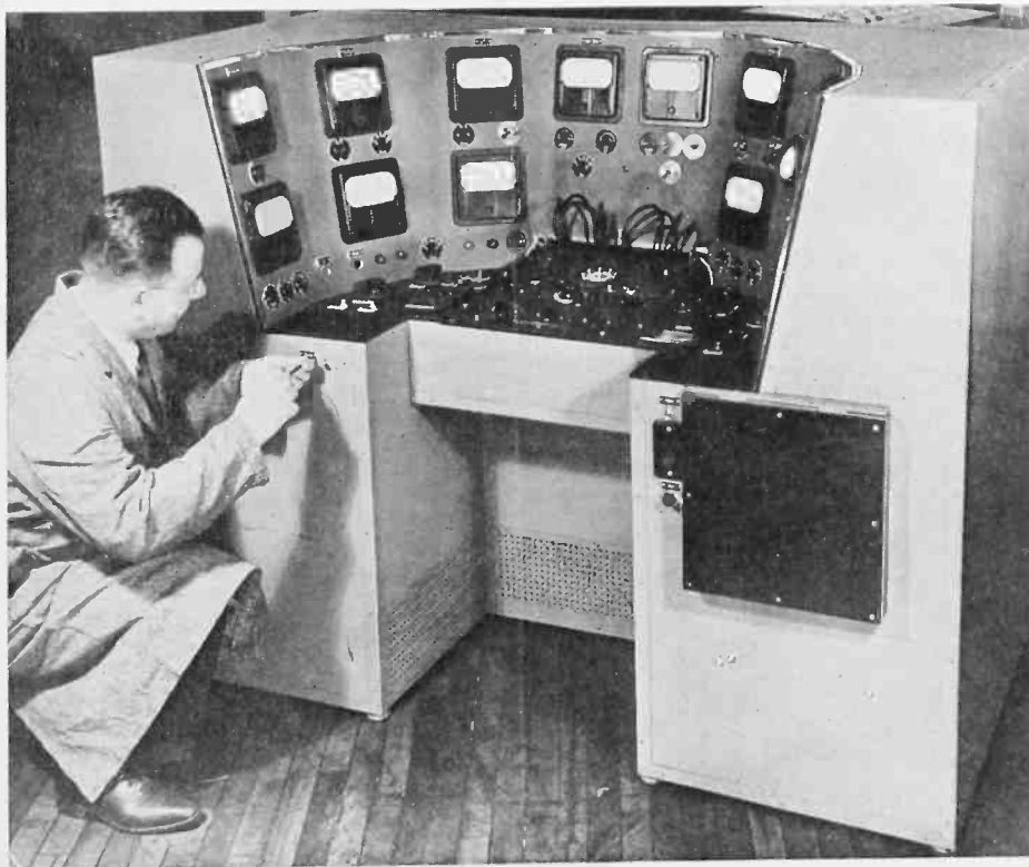
FIGURE 2. Laboratory Tube Test Set—An Example of Sylvania Design.
