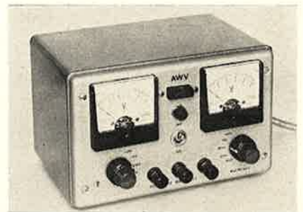
THE ORIGINAL REGULATED BIAS SUPPLY WHICH FORMS THE BASIS OF THIS ARTICLE.
