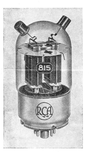
with very low driving power. For example, a single 815 operated in push-pull class C telegraph service is capable of handling a power input of 75 watts (ICAS) with less than 0.2 watt of driving power.
