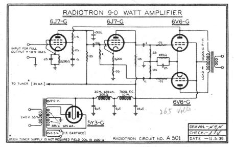
This circuit gives a power output of 9 watts with a total overall harmonic distortion less than 3% second harmonic and negligible higher order harmonics. The input voltage for maximum power output is 0.31 volt RMS. and the gain reduction due to feedback is 3.98.
