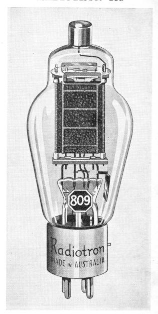
Radiotron 809 is a transmitting triode with a plate dissipation of 25 watts. It may also be used as an audio frequency Class B Amplifier or modulator with a power output up to 100 watts from two valves. Radiotron 809 is Australian-made.
