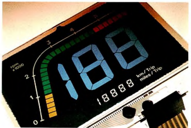
Fig.13 Prototype Videlec integrated display (VID) with chip-on-glass and printed translucent colours, the LCD is driven in a multiplex 1:2 mode
