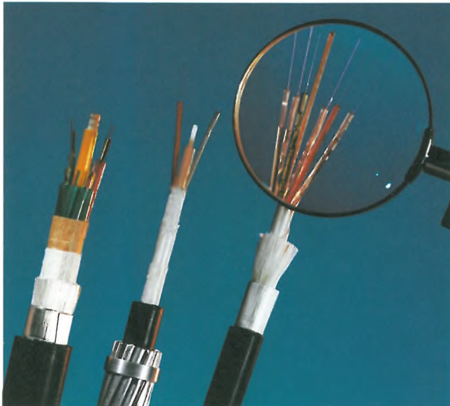
Fig. 2. Three optical-fibre cables. The left-hand cable contains six groups of ten optical fibres. The cable at the centre is a high-voltage cable intended for power distribution, with two optical-fibre cables at the centre for communication purposes. The right-hand cable contains six separate optical fibres. The optical fibres themselves are extremely thin, but each can carry many millions of bits per second.
