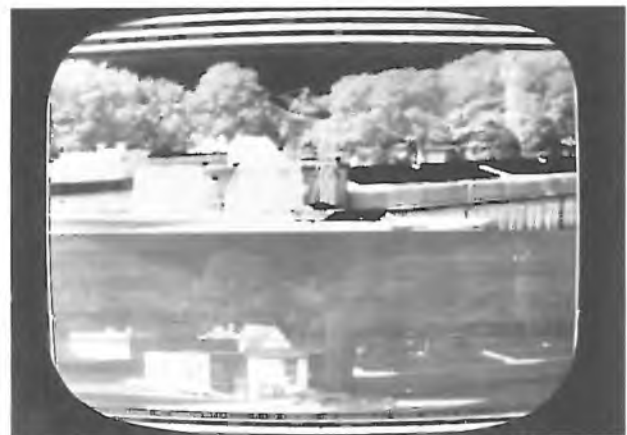
Fig. 11. An application of the image bulk-storage system. Here two optically coincident infrared images from the IRSCAN system are combined on one television screen. The upper image displays information obtained at wavelengths of 8 to 14 μm; the lower image represents wavelengths of 3 to 5 μm.
