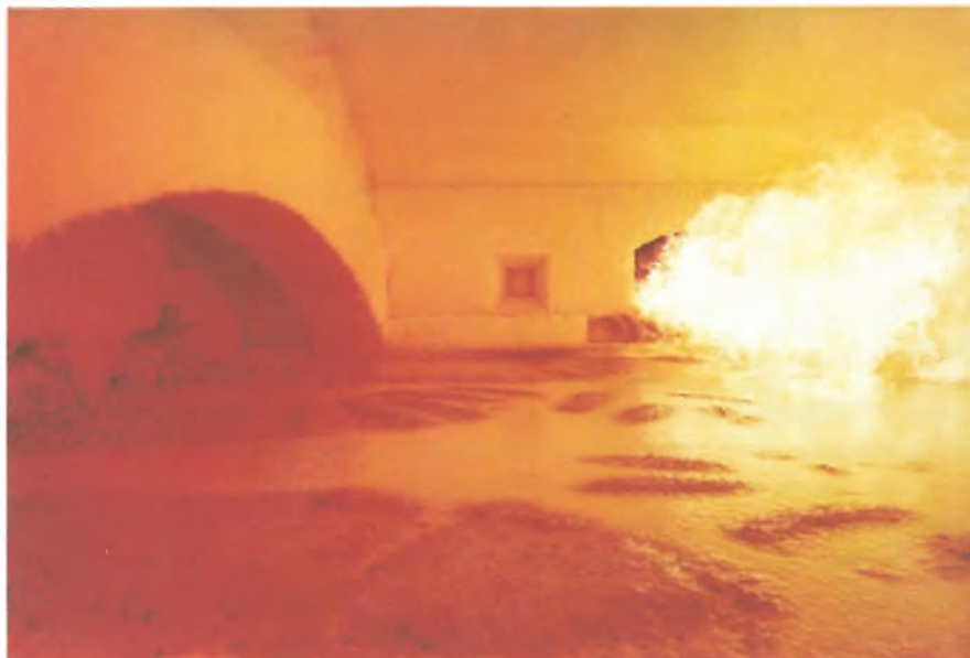
Fig. 2. Looking into a glass furnace at the Philips glassworks in Aachen, West Germany. The mix enters the furnace through the three openings on the left of the furnace, to form the 'sandbanks' further along in the 'river' of molten glass. The furnace is 7 m wide and 15 m long, and contains a glass melt about 1 m deep. Above is one of the burners that melt the mix at a temperature of about 1350 °C.
