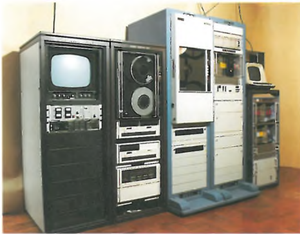
Fig. 3. System hardware under test in the laboratory. From left to right: preprocessing and postprocessing rack with monitor; system-control computer and computer-compatible tape recorder; 24-track digital image tape recorder (the actual image bulk store); electronics of digital image tape recorder in combination with sync encoder and sync decoder; electronic frame store control console.
