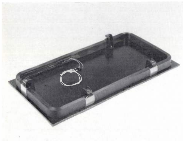
Fig. 5. One of the coils of the magnetic 'torquer'. There are three such coils at the base of the satellite, each perpendicular to one of the coordinate axes ( fig. 2 ). The coils are orthocyclically wound (5) with aluminium wire and embedded in a thermoplastic material. The power required is 2 W. Each coil delivers a maximum torque of 5 \times 10^{-4} Nm.
