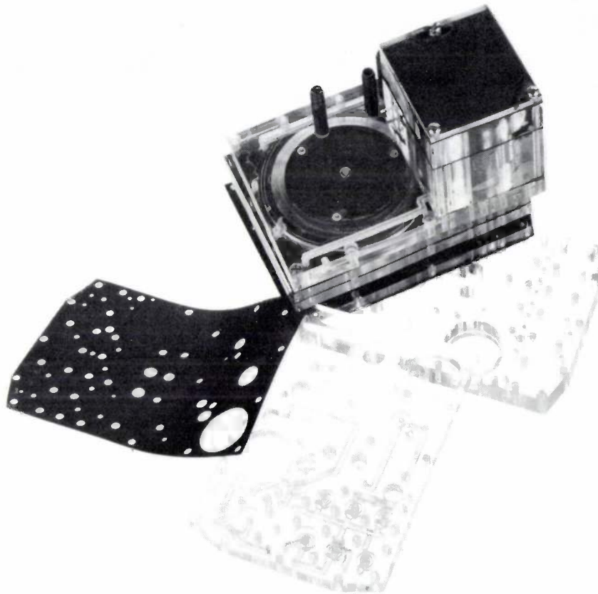
Fig. 14. The sandwich construction of the control system; the plastic plates and rubber sheets have been stacked one above the other without the separate components of the logic elements (springs, valves, etc.). Two plates and a rubber sheet have been turned outwards to show details on the bottom plates such as the row of diaphragm seats for the baffle nozzles of the programme input, and the motor piston chamber. The block mounted on the top plate contains the delay element. The pressostat diaphragm is visible through the top plate.
