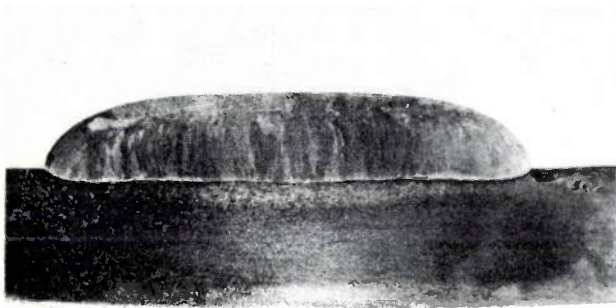
Fig. 4. Square-butt weld in plate of 8 mm stainless steel welded by the plasma-MIG method using a thin arc. The filler wire (PZ 6061) had a diameter of 1.2 mm and was also of stainless steel. The plasma gas was argon (6.5 l/min), the shielding gas a mixture of argon (10 l/min) and CO 2 (5 l/min). The diameter of the plasma exit was 6 mm, and its distance to the workpiece was 15 mm. Plasma-arc current 100 A at 50 V. Current in the filler wire 180 A at 40 V. Both electrodes were positive with respect to the workpiece. The rate of travel was 40 cm/min at a deposition rate of 95 grams of filler metal per minute. Under these conditions the critical current through the wire at which the arc starts to rotate is approximately 250 A.
