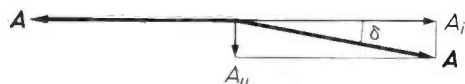
Fig. 2. A slight deviation \delta in the 180^\circ phase difference between the light (amplitude A ) reflected from the bottom of a pit and light reflected at the record surface beside it gives an out-of-phase component with an amplitude A_u . Now A_u = A \sin \delta \approx A\delta . The corresponding intensity is therefore A^2\delta^2 . Since \delta is directly proportional to variations from the nominal value \frac{1}{4}\lambda for the depth of the pit, the remaining intensity is proportional to the square of the deviation from the correct depth.
