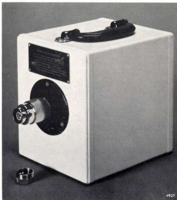
Fig. 12. Ionization chamber in open communication with the atmosphere and containing an internal radiation source for correcting the sensitivity of the measuring circuit (figs. 11 and 13) to allow for different values of temperature and air pressure.
