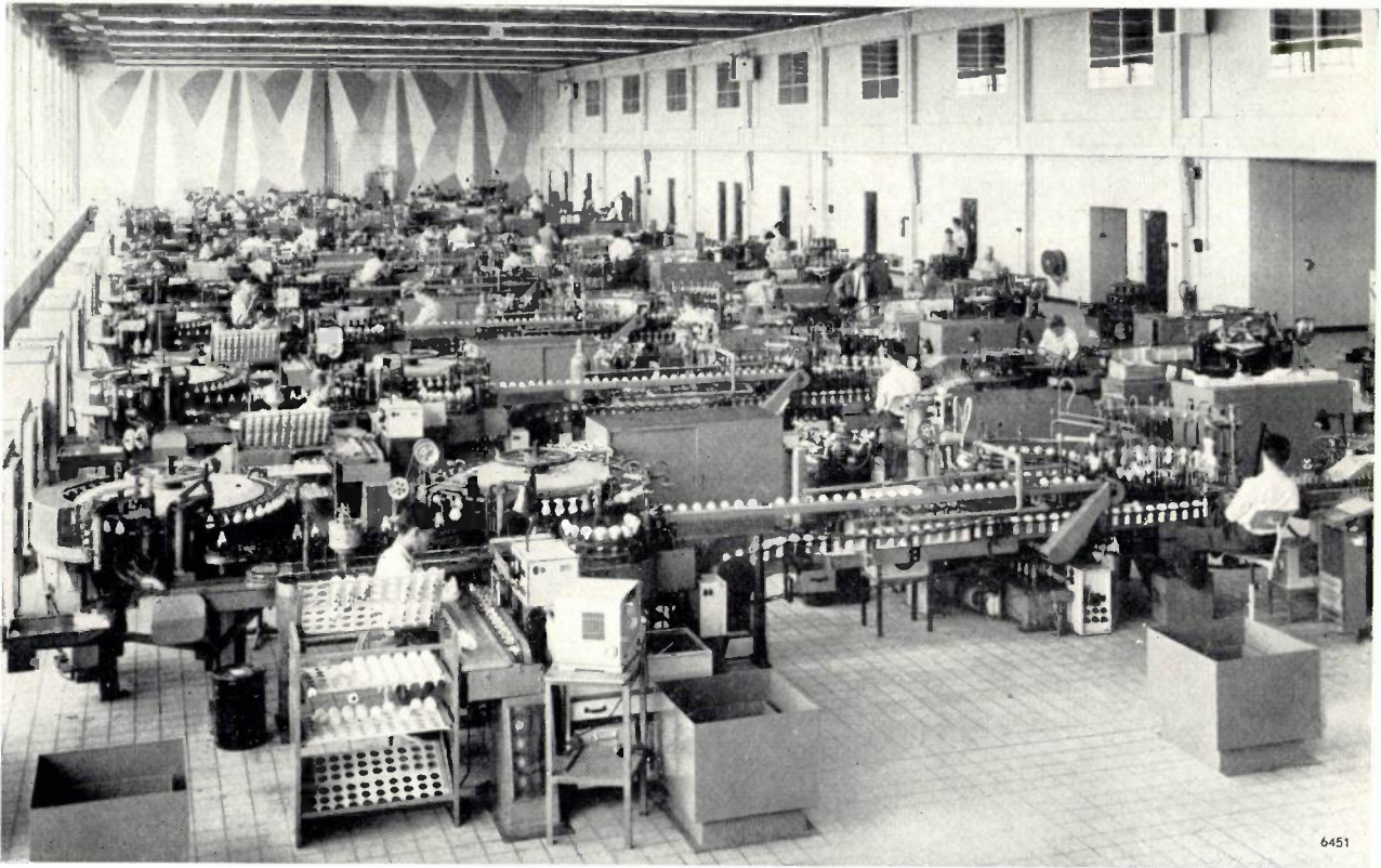
Fig. 10. A modern lamp factory: hall with a number of production groups parallel to each other, in the Philips lamp works at Weert (Netherlands), opened in 1961. Each production group covers the whole width of the hall and constitutes an independent unit. Each group, which is operated by three or four persons, is supplied with tungsten filaments, support
