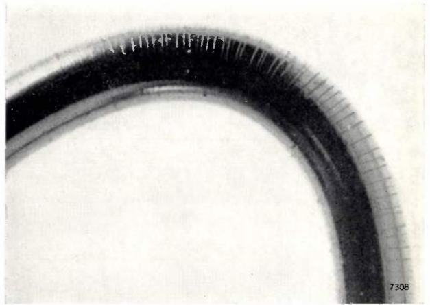
Fig. 11. A series of cracks (magnification 20 \times ) in a piece of "Povin" wire, produced by bending the wire and dipping it into methanol. No really satisfactory explanation has yet been found for this "solvent cracking".
