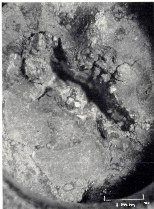
Fig. 14. Effect of the focussed electron beam on a gold target after exposure for about 1.5 hours.
