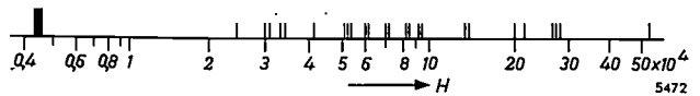
Fig. 15. Measured values of rejection factor H (thin marks) and calculated minimum value H_{min} (thick mark) for the circuit of fig. 14 .
