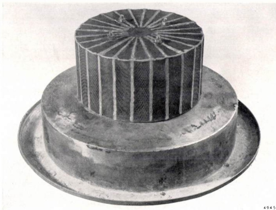
Fig. 3. Cylinder of fine copper gauze, on which water vapour and carbon dioxide from the air are deposited in the form of porous snow.
