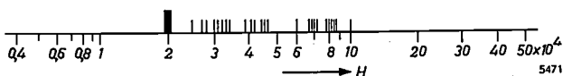
Fig. 13. Measured values of rejection factor H (thin marks) and calculated minimum value H_{min} (thick mark) for the circuit of fig. 12 .
