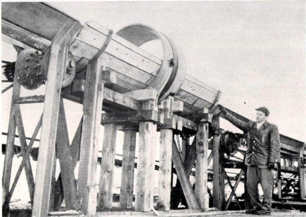
Fig. 15. Metal detector, in use in the sawmill of Tunabergs Trävaru AB at Koppartorp. The logs on their way to the saws are transported on a non-metallic conveyor through the coil 1 metre in diameter seen in the centre of the picture. Logs containing big nails or other metal objects that might damage the saws change the inductance of the coil during their passage and thereby actuate a relay giving an alarm signal. (The relay in some installations causes a paint gun to produce a spot on the log at the location of the metal, or it causes the log to be put off the conveyor.)
