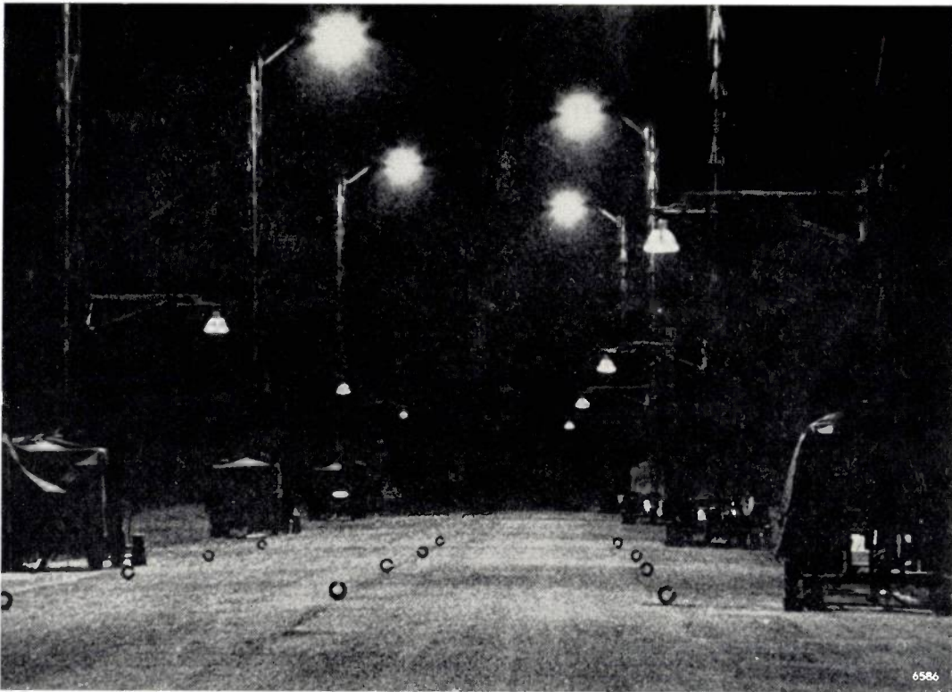
Fig. 9. View of Philips outdoor laboratory for road lighting at Turnhout 14) , showing Landolt rings systematically distributed for investigating the influence of the kind of light on perceptibility.
