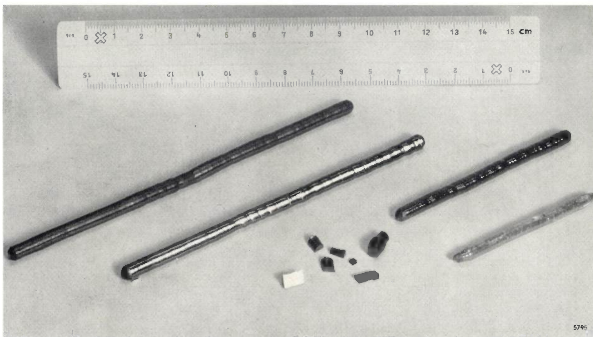
Fig. 4. Some monocrystalline rods of oxides produced in different atmospheres with the apparatus described. The zone speed in all cases was 6 cm per hour. From left to right: \text{MnFe}_2\text{O}_4 in air; \text{Mn}_{1.1}\text{Fe}_{1.9}\text{O}_4 in nitrogen with 0.2% oxygen; \text{Mn}_{1.2}\text{Fe}_{1.8}\text{O}_4 in nitrogen with 0.2% oxygen; \text{TiO}_2 in air. In the foreground are some fragments of an NiO rod, showing good cleavage planes; this rod was grown in pure oxygen.
