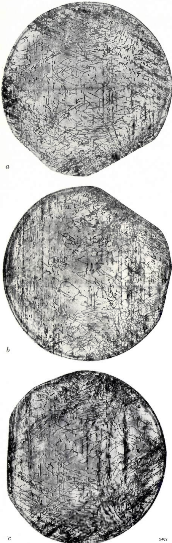
Fig. 10. Three projection topographs of the same slice as in fig. 5, made by reflection from a ) the (11\bar{1}) plane, b ) the (1\bar{1}1) plane, c ) the (\bar{1}11) plane. The photographs illustrate the varying visibility of individual dislocations when different reflections are used.
