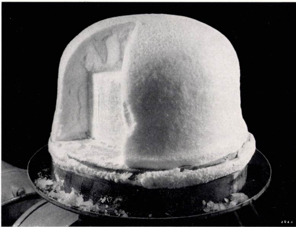
Fig. 4. A porous snow cake, about 10 cm thick, grown on the gauze in about a week.
