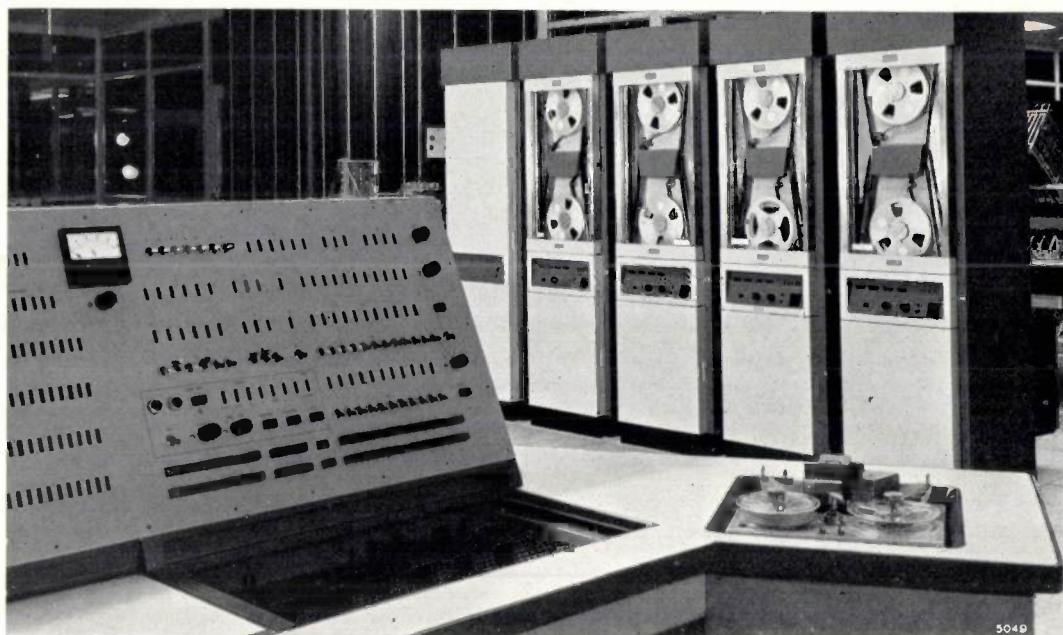
Fig. 11. Part of the control desk. At the back are some tape units which are used as a large, slow memory. The plug-board memory can be vaguely seen on top of the desk while the push-button register for address 0 is at the bottom right-hand side of the panel. To the right on the desk there is the reader for the input of programmes recorded on punched tape.
