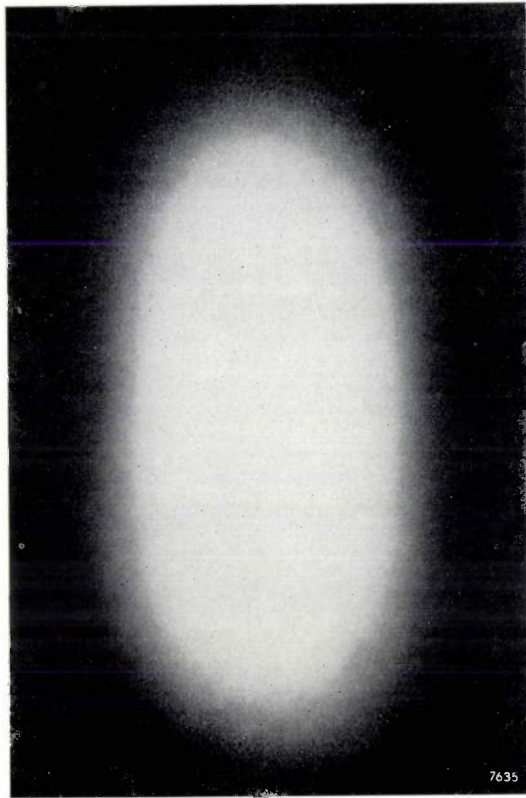
Fig. 20. Autoradiograph (true size) of the cross-section of the external proton beam, three meters behind the exit of the extraction system. The quadrupole lenses (2 in fig. 1) were not in operation when this autoradiograph was made.
