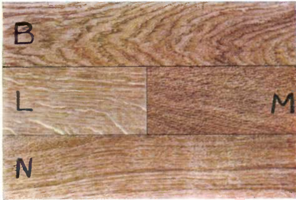
Fig. 10. Oak parquet blocks of four different classes: L bright, N medium, M dark, B patterned.
