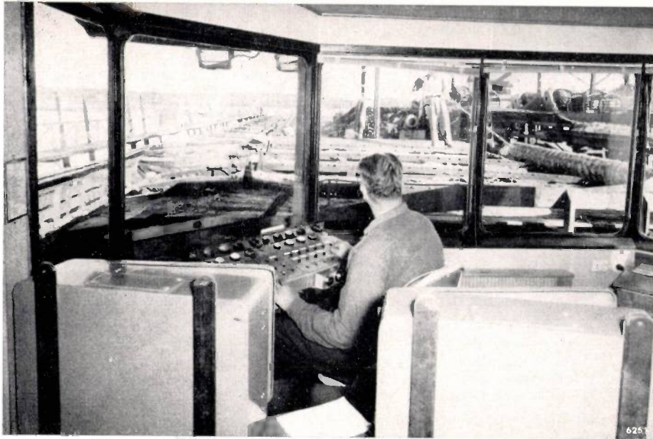
Fig. 18. Operator at desk containing the 23 buttons for directing the logs to their respective bays. The logs arrive from the right-hand side on the platform visible through the window. To the left the conveyor with the 23 bays.
