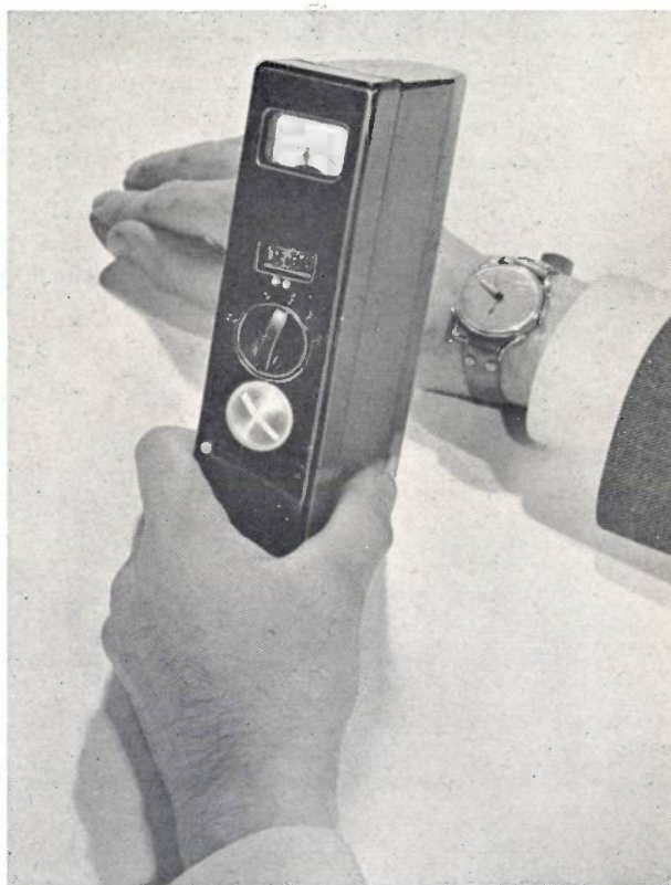
67065 Portable radiation counter for detecting beta and gamma rays, fed entirely from built-in batteries. The counter reacts perceptibility to the rays from the luminescent paint on the hands of a watch.
