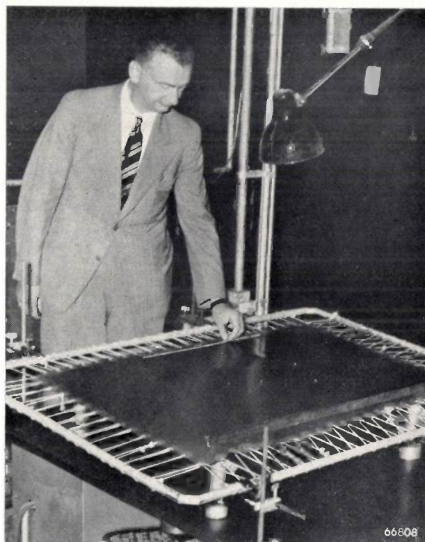
Small steel balls made to roll over a sheet of rubber give a picture of the paths followed by electrons in, for instance, electronic valves.
