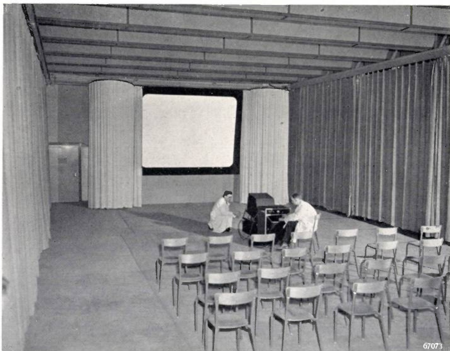
Hall for acoustical investigations (i.a. stereophony) and large-screen television (almost 3\text{ m} \times 4\text{ m} ).
