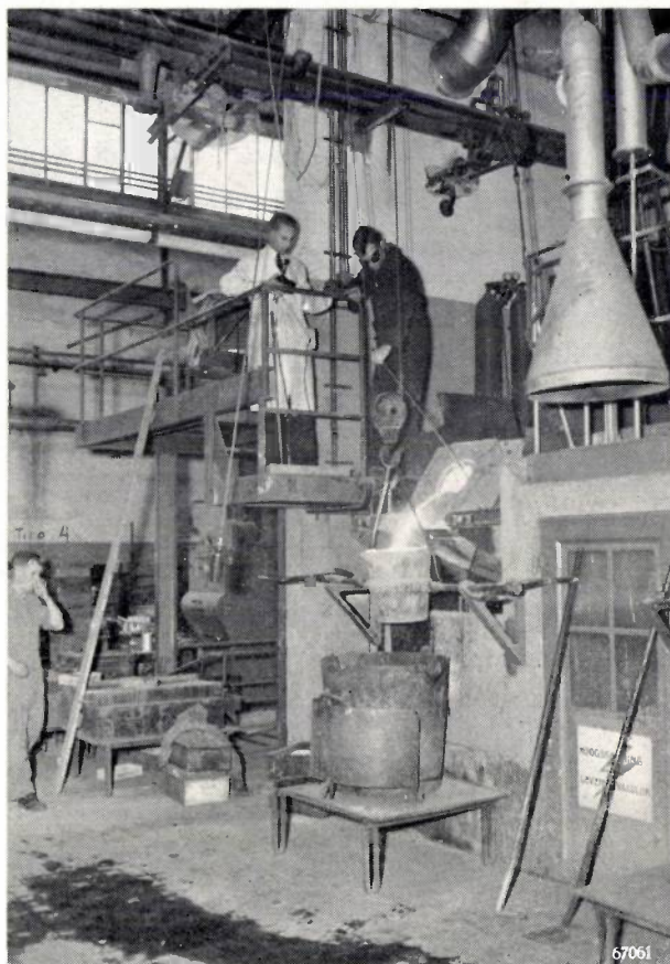
Preparation of magnet steel. Emptying the furnace in which the alloy has been melted by induced high-frequency currents.
