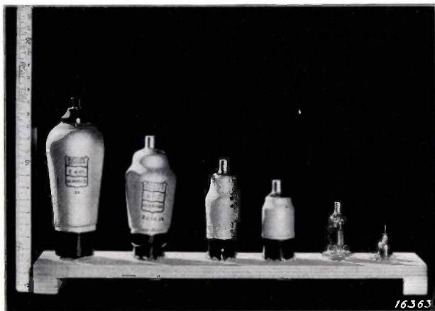
Fig. 3. The picture depicts the evolution of the high-frequency amplifying valves (pentodes) for short-wave reception. The second valve on the left (AF7) is used in modern radio receivers. The smallest pentode on the right, which is a little more than 1 cm high can still be used at a wave length of 50 cm.
