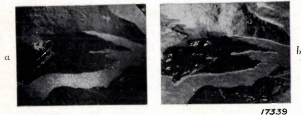
Fig. 6. Crystalline structure diagram of iron on magnification 20 times: Agreement between a the emission diagram (at 880 °C) and b the etching diagram (at 20 °C).
