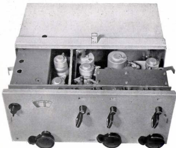
Fig. 5. V.O. 18 receiver with chassis pulled out. The housing and chassis are made of duralumin.
