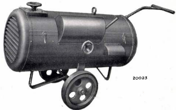
Fig. 9. Twin-current welding unit, type 1306. The lever change-over switch serves for changing over from alternating to direct current. The current intensity is regulated by means of the upper handwheel; the magnetic shunt cores are clamped against the middle core by means of the side handwheel.
