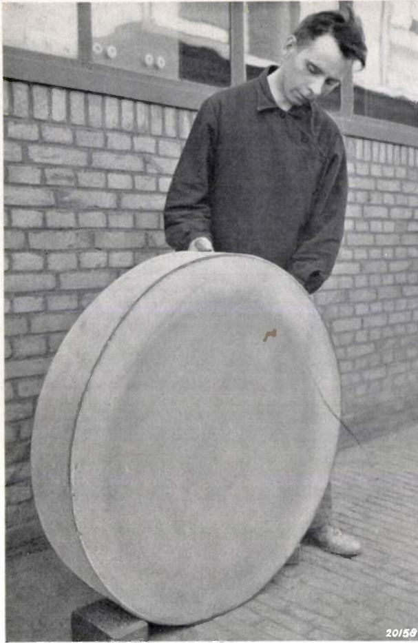
Fig. 4. Chromium-iron casting of 35" diameter, covered on the front with glass to a thickness of 10 mm (shaded). The glass is later ground completely smooth, after which the surface is silvered.
