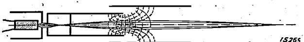
Fig. 6. Arrangement of an electronic lens in the Philips 3951/3952 cathode ray tube. Lines of force: — — — — —; equipotential surfaces: - - - - -; path of electrons: —
