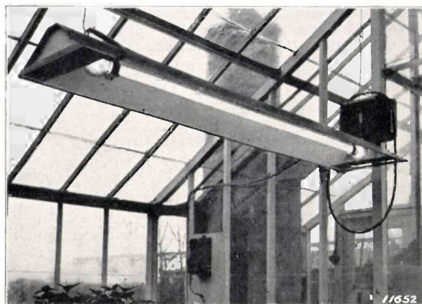
Fig. 10. The large plant irradiator 4310 installed for use. The input unit ( T, B, R, C and S in fig. 8 ) is enclosed in the watertight cast-iron box on the right, to which the tubes mounted in the reflector are connected by a cable.
