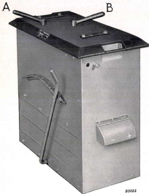
Fig. 10. Twin-current unit, Type 1307. The side lever serves for adjusting the current, while changing over from alternating to direct current is performed by means of the switch B on the cover. The clamping arrangement is operated by means of the crank A.
