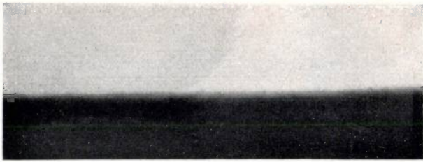
Fig. 4. a) Edge of an unmodulated Philips-Miller sound track, magnification \times 100 . The absence of granulation is clearly visible also in the transparent part removed by the cutter wedge.
