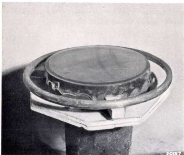
Fig. 2. Casting for a 12" concave mirror (focal length 80"). On affixing the glass, part has run over the edge. Shaping is done by polishing two glass discs one against the other, using a suitable lubricant (carborundum, alundum or rouge).
