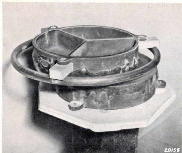
Fig. 1. Rear side of the 12" mirror. The casting by which the mirror is later secured in the telescope can be clearly seen. During surface working which is done by hand a wood ring is attached to the casting to provide a grip.
