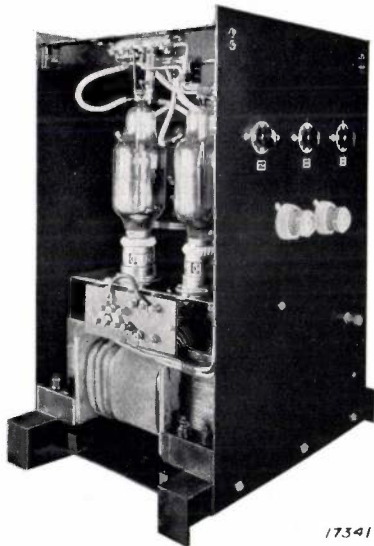
Fig. 4. View of a telephone rectifier for 50 volts and 7 amps D.C. The unit is wired as shown in the diagram in fig. 3 . It is suitable for connection to a single-phase A.C. mains supply and can be adjusted for various supply voltages between 190 and 260 volts (50 cycles).
