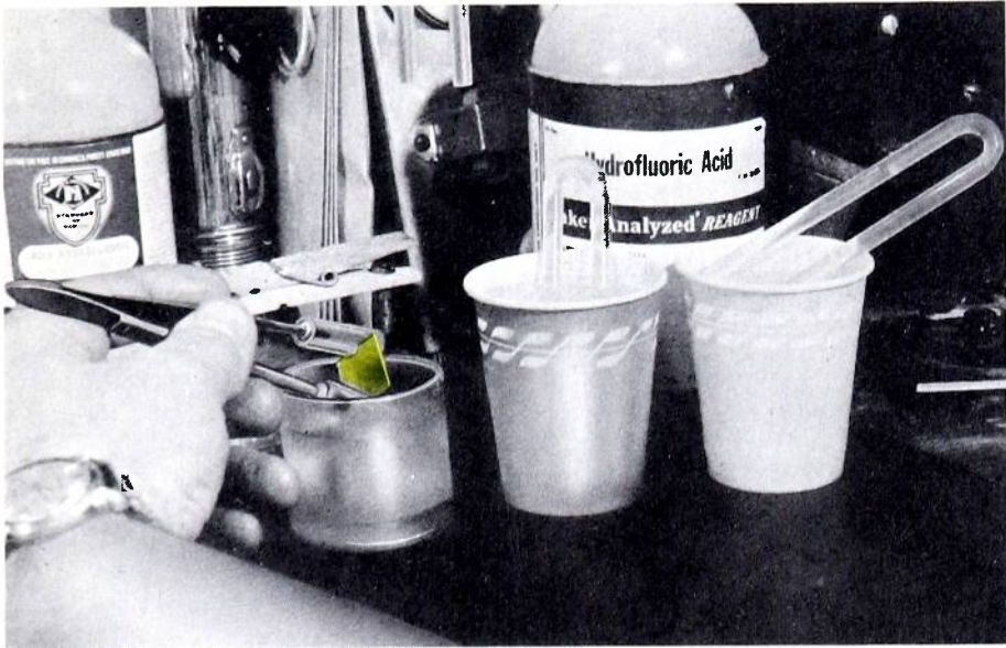
Figure 4. Equipment Required for Crystal Etching, Including Tongs, Acid Bath, Neutralizer Bath with Tongs, and Rinse Bath with Tongs
