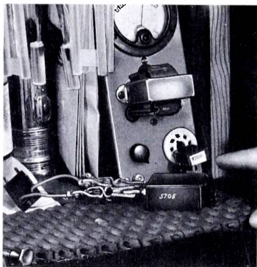
Figure 2. Test Oscillator Used To Determine Crystal Frequency
