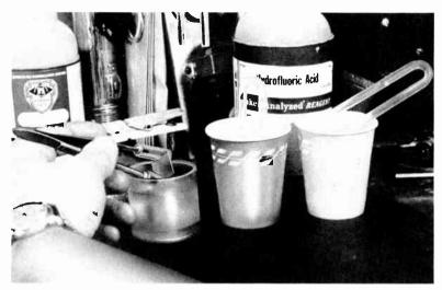
Figure 4. Equipment Required for Crystal Etching, Including Tongs, Acid Bath, Neutralizer Bath with Tongs, and Rinse Bath with Tongs
