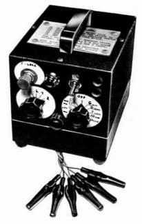
Figure 2. Utility Synchro Test Set
