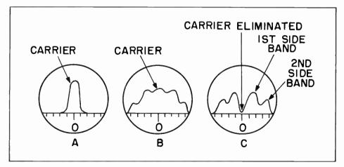
Figure 2. Panoramic Adapter Presentations Used in Calibration of T-14/TRC-1 Transmitter
