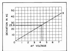
Figure 3. Graphical Representation Showing Frequency Deviation Versus Arbitrary Values of R-19/TRC-1 Output Voltage
