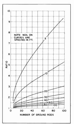
Figure 5. Ratio of Resistivity of Ground Rods in Parallel in an Area to That of Isolated Rods
