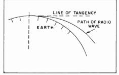
Figure 2. Bending Effect of Radio Wave Due to Variable Velocity of Propagation
