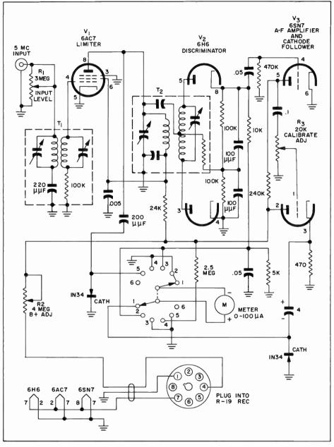
Figure 1. Schematic Diagram of Deviation Meter
