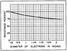
Figure 1. Relation of Electrode Diameter to Ground Resistance (Soil of Uniform Resistivity)
