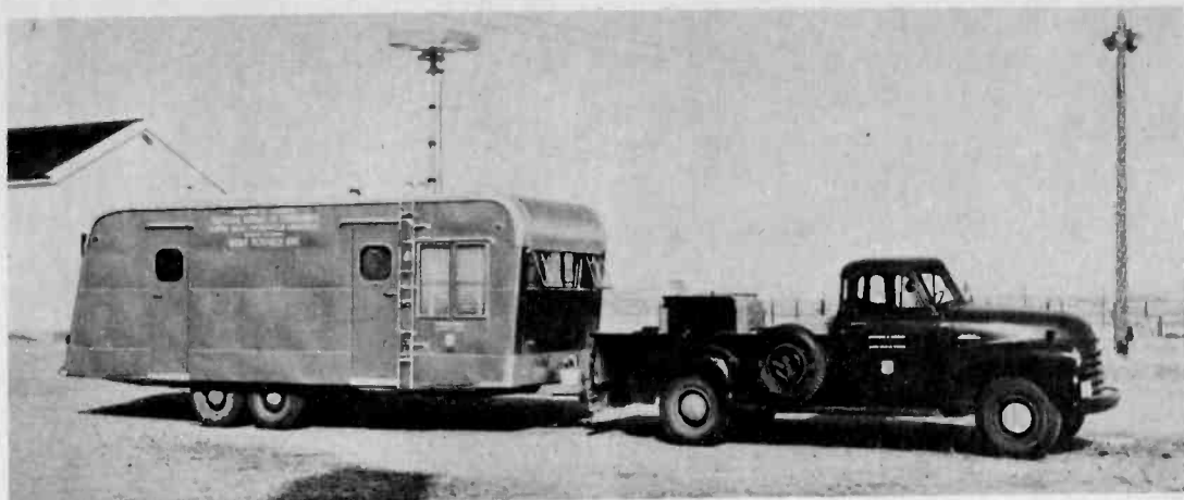
Figure 6. Mobile Research Unit Used by the National Bureau of Standards to Measure the Field Strength of Radio Signals. Mobile units such as these have been sent to Pikes Peak to determine range of transmitted signals from installations in the general area. Others have cruised in service areas common to several transmitters to determine the amount of interference offered by each station. The antenna (on top of trailer) can be raised to a height of 30 feet by remote control while the unit is in motion.
