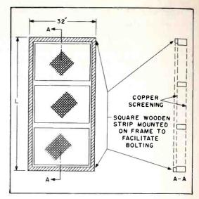
Figure 3. Construction of a Typical Cell
