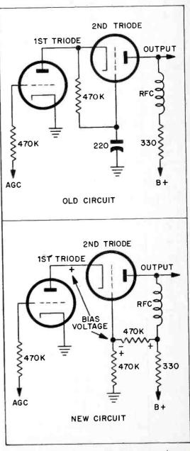
Figure 12. Circuit Modification for Improved AGC Performance
