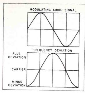
Figure 4. Phase Relationship Between Modulating Signal and Carrier Deviation
