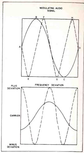
Figure 5. Comparison of Two Modulating Signals to Carrier Deviation, Showing the Effect of Increasing the Modulating Frequency
