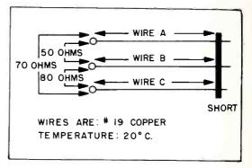
Wire-to-Wire Resistance Measured on Shorted Three-Wire Circuit
