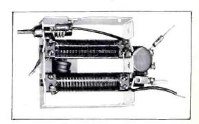
Figure 4. Tapered-Line Input Section
