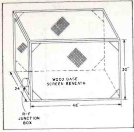
Figure 6. Poor Man's Screen Room
