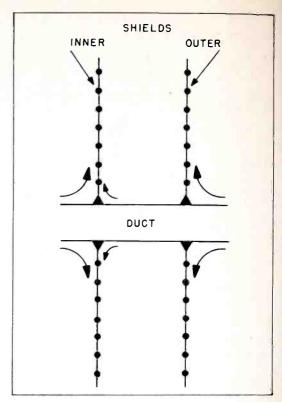
Figure 5. Paths Taken by Interfer<mark>ence</mark> When Duct for Power Line is Sold<mark>ered</mark> to Both Shields
