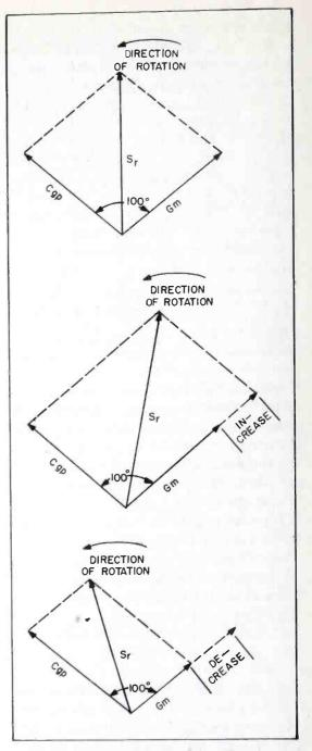
Figure 3. Vector Diagram Showing Effect of Modulation
