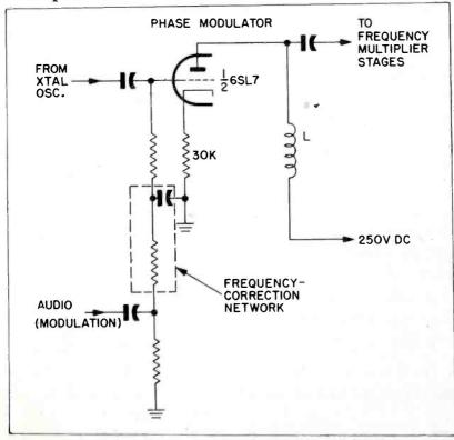
Figure 1. Schematic Diagram of Phase Modulator
