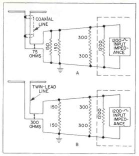
Figure 3. Simplified Diagram of Tapered-Line Input Section
