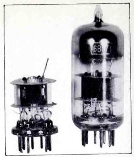
Figure 10. Left—An Assembled 6BQ7
