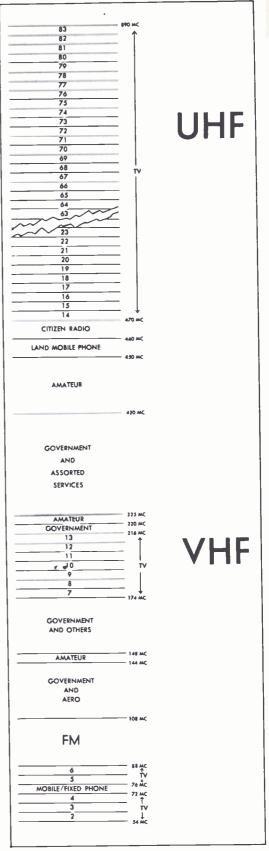
Figure 1. TV-Channel Frequency
