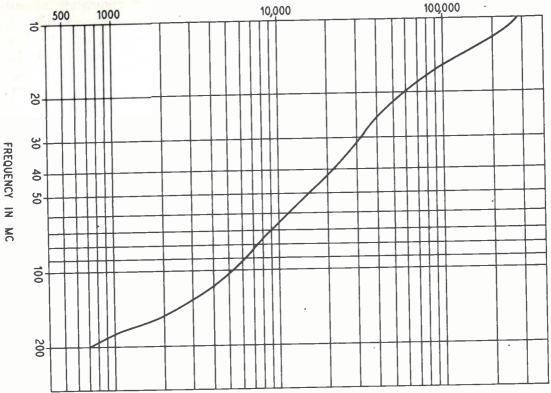
Figure 5. Input Resistance of a 6AG5 at Various Frequencies
