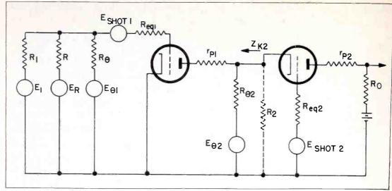
Figure 8. Noises Sources in a Modified Cascode Amplifier
