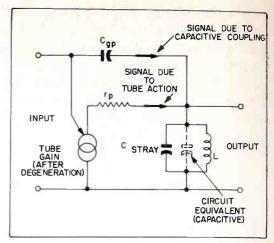
Figure 2. Equivalent Circuit of Phase Modulator
