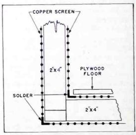
Figure 7. Construction Details at Joint of Floor and Wall
